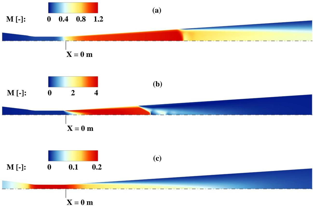
**Figure 13.** Contour plot of the Mach number in the throat and downstream regions (predictions of the pressure-based solver): (a) Case 1 of **Table** :  $p_{in} / p_{out} = 11.4 \text{ bar} / 2.6 \text{ bar}$ , (b) Case 2 of **Table** :  $p_{in} / p_{out} = 43.0 \text{ bar} / 10.0 \text{ bar}$ , and (c) Case 3 of **Table** :  $p_{in} / p_{out} = 133.0 \text{ bar} / 124.2 \text{ bar}$ .
