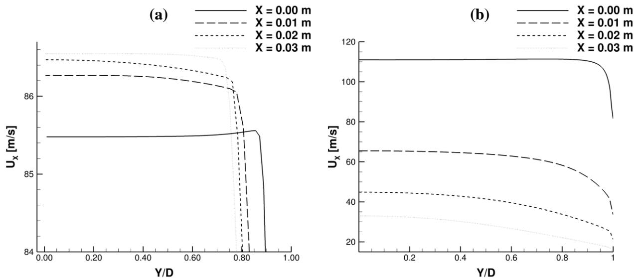
**Figure 14.** Cross-flow velocity profiles for: (a) subcritical case 2 ( $U_{x,max} = 86.6$  m/s) and (b) supercritical case 3 ( $U_{x,max} = 111.4$ ) m/s of **Table** .
