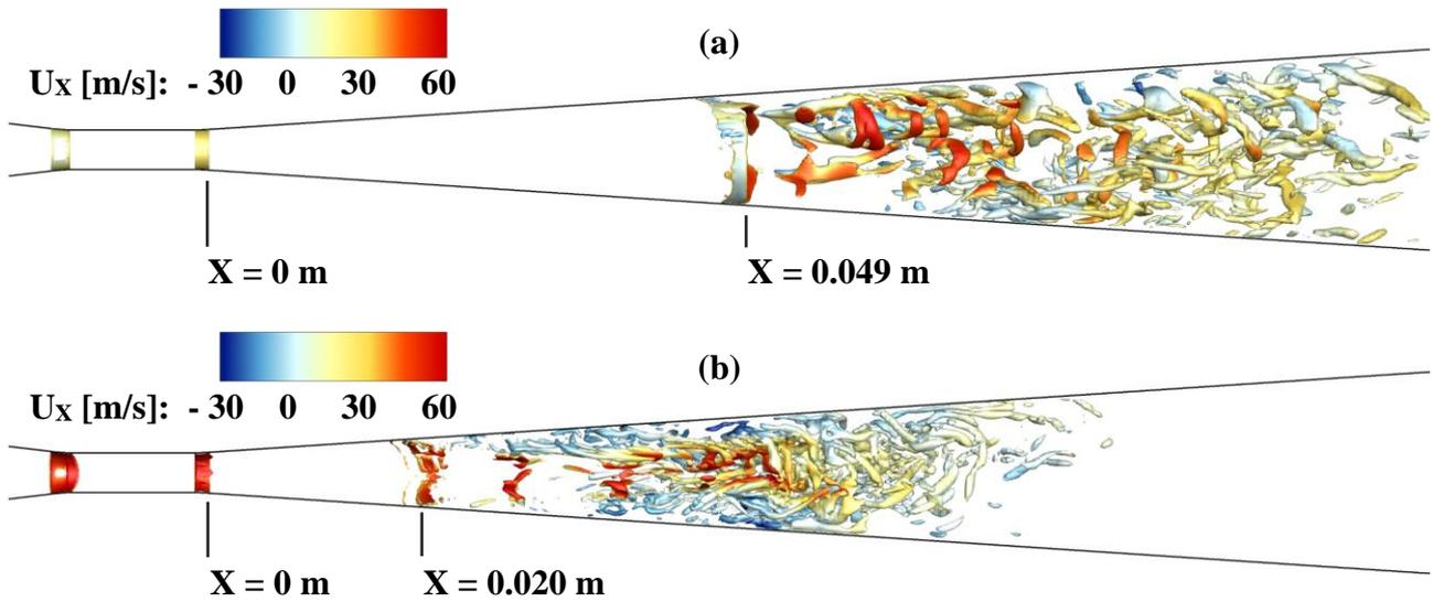
**Figure 18.** Visualisation of vortices using  $Q$ -Criterion iso-surfaces ( $Q=2 \cdot 10^8$ ) coloured by axial velocity values for the DES results of (a) Case 1 of **Table** :  $p_{in} / p_{out} = 11.4 \text{ bar} / 2.6 \text{ bar}$ , (b) Case 2 of **Table** :  $p_{in} / p_{out} = 43.0 \text{ bar} / 10.0 \text{ bar}$ . The figures include the part of the nozzle from  $X = -0.017 \text{ m}$  to  $X = 0.11 \text{ m}$ .
