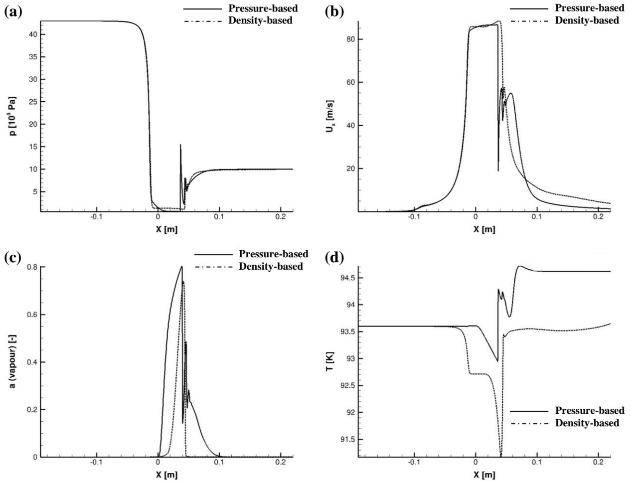
**Fig. 10.** (a) Pressure, (b) velocity, (c) vapour volume fraction and (d) temperature distributions at the orifice symmetry axis, as predicted by the two thermodynamic approaches for case 2 of **Table** .
