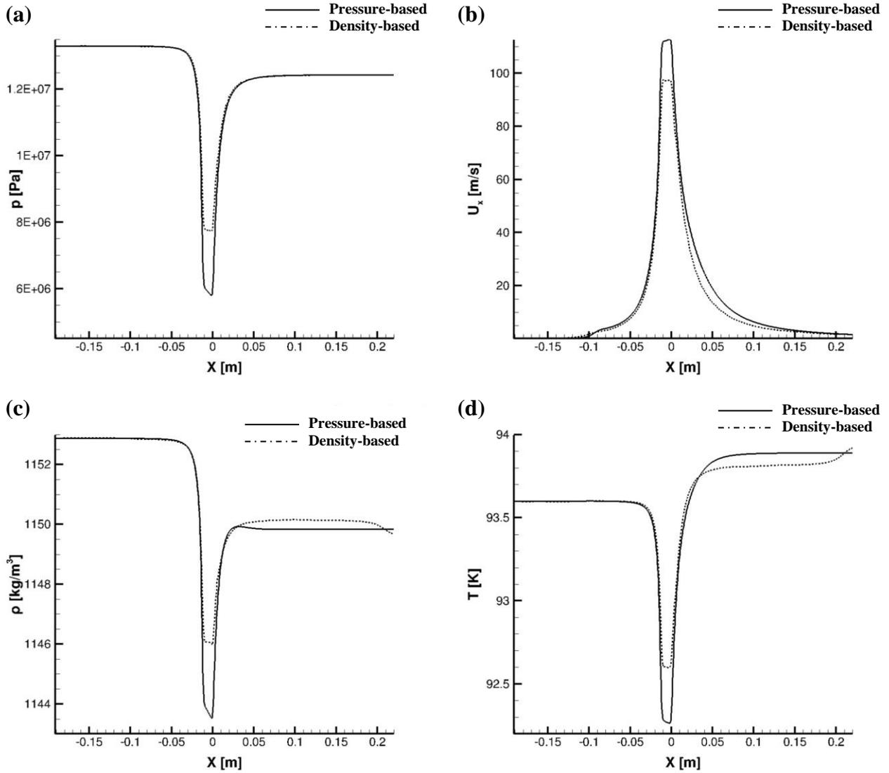
**Figure 12.** Distribution of (a) pressure, (b) velocity, (c) density and (d) temperature at the orifice symmetry axis, as predicted by the two solvers adopting different thermodynamic approaches for case 3 of Table .
