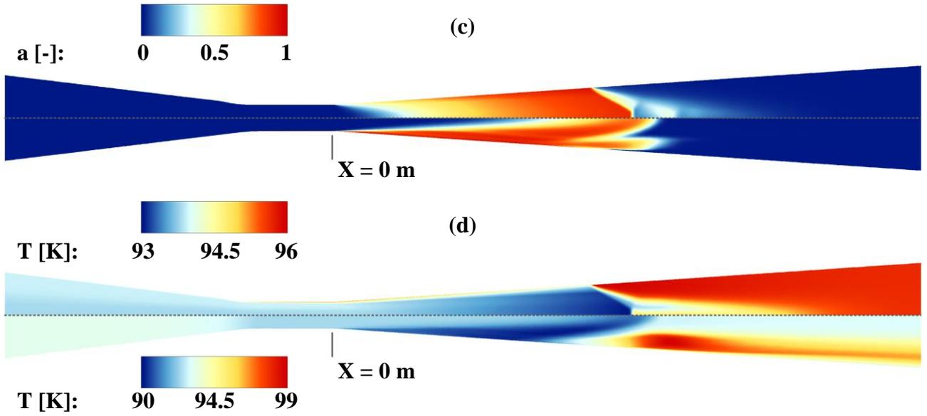
**Fig 9.** Contour plots of the (a) pressure, (b) velocity (c) vapour-volume fraction and (d) temperature fields in the nozzle throat region for case 2 of **Table** . It is noted that different variable ranges have been used in frame (d) to enhance clarity. Upper and lower panels depict predictions produced using the pressure- and density-based solver, respectively. All contours represent the part of the nozzle from  $X = -0.045$  m to  $X = 0.08$  m.
