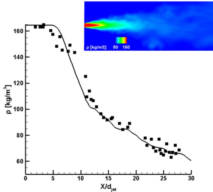
**Fig. 6.** Validation of the pressure-based solver using NIST-REFPROP database: Comparison of numerical predictions of the average  $N_2$ -jet density distribution at the jet axis (solid line) against experimental data (symbols) [58]. The average density contour plot is depicted in the inset.
