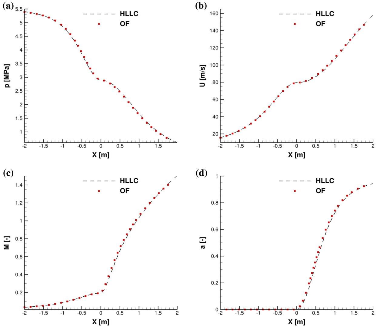
**Fig. 5.** Validation of the density-based solver (OF) for the converging-diverging nozzle case: Numerical results for (a) pressure, (b) velocity magnitude, (c) Mach number (d) vapour volume-fraction distributions along the orifice symmetry line and comparison against the predictions of the 1-D solver (HLLC).
