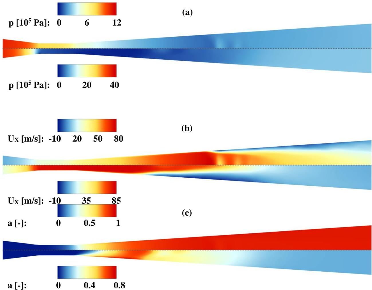
**Figure 15.** Contour plots of time-averaged field over the nozzle plane of symmetry; upper frames correspond to case 1 and lower ones to case 2 of **Table** : (a) pressure (b) axial velocity and (c) vapour-volume fraction. The figures include the part of the nozzle from  $X = -23.5$  mm to  $X = 98.2$  mm.
