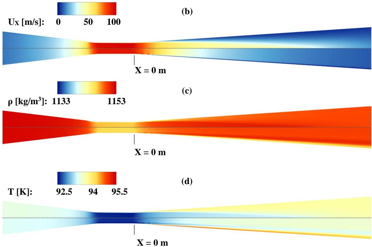
**Figure 11.** Contour plots of the (a) pressure, (b) velocity, (c) density and (d) temperature field for supercritical injection (case 3 of **Table 1**). Upper frames of each figure depict the predictions produced using the pressure-based solver and the NIST database, while lower frames those produced using a density-based solver and tabulated data produced by solving the Helmholtz EoS. All contours represent the part of the nozzle from  $X = -0.045$  m to  $X = 0.08$  m.
