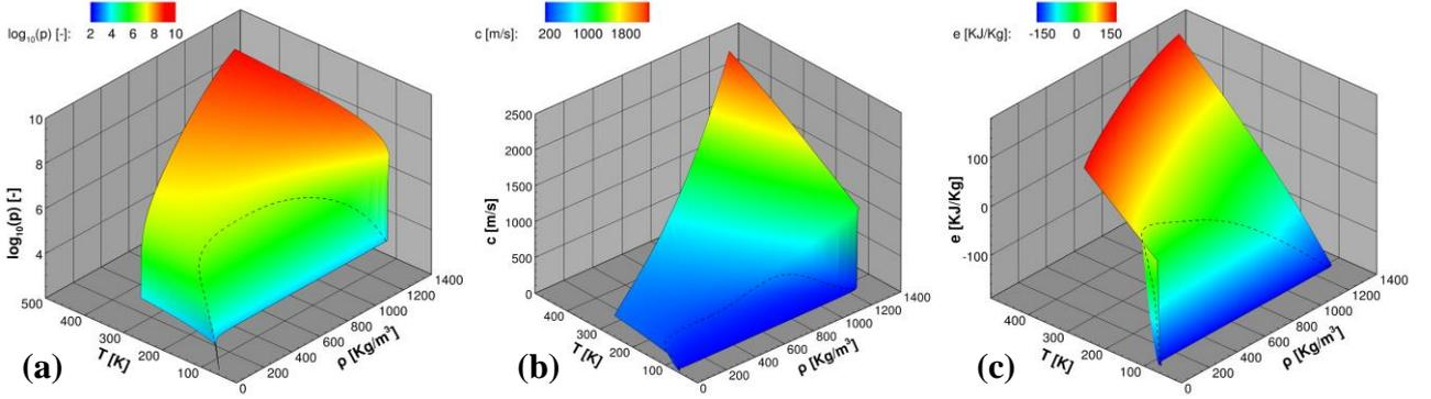
**Fig. 1.** Three-dimensional phase diagrams for oxygen: (a) pressure, (b) speed of sound and (c) internal energy in terms of density and temperature.
