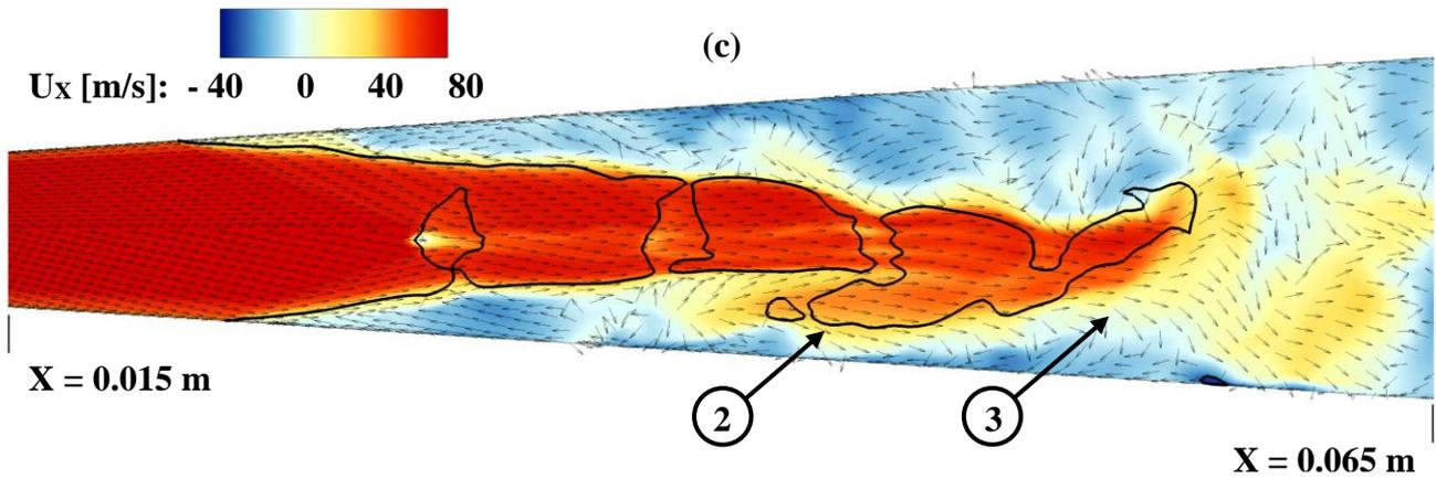
**Figure 16:** Velocity vectors over axial velocity contour plots in a detailed view after the nozzle throat exit ( $X=0.015$  m) corresponding to characteristic time instances of DES: (a)  $t=0.240$  s, (b)  $t+1.0$  ms and (c)  $t+2.0$  ms. The black iso-line signifies  $M=1$  regions, while the numbered vectors indicate regions of distinct flow features.
