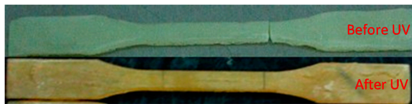
Figure 11. Comparison of physical changes of resin adhesive specimens before and after UV exposure.
