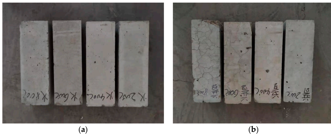
Figure 3. The changes in the color and surface cracks of specimens after high temperatures: (a) SAC, (b) NC.
