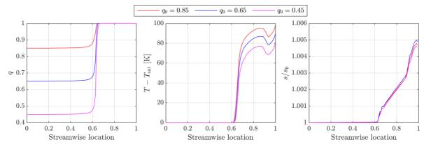
**Figure 7:** Variation in circumferentially averaged vapour quality (left), degree of superheat (centre) and normalised entropy (right) with streamwise location for different inlet vapour qualities.
