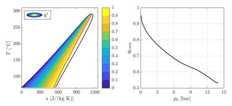
**Figure 3:** Vapour qualities related to the two-phase expansion of MDM. Left: throat vapour quality  $(q^*)$  for isentropic expansion from within the saturation dome; right: minimum stagnation vapour quality  $(q_{0,\min})$  that results in dry expansion downstream of the throat at different stagnation pressures  $(p_0)$ .
