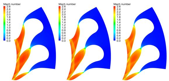
**Figure 9:** Mach number contours for different inlet vapour qualities: left:  $q_0 = 0.85$ ; centre:  $q_0 = 0.65$ ; right:  $q_0 = 0.45$ . Speed of sound is defined using the ANSYS built-in function which calculates the speed of sound based on the volume-weighted sum of the acoustic impedances of the saturated components.
