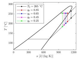
**Figure 1:** Expansion of MDM from a stagnation pressure of 8 bar to 0.4 bar with varying inlet conditions.
