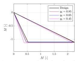
**Figure 6:** Stator outlet Mach number triangles based on averaged velocities.
