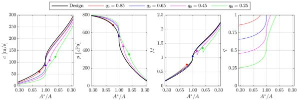
**Figure 2:** Variation in velocity c, pressure p, Mach number M, and vapour quality q, for an isentropic expansion of MDM from different stagnation vapour qualities  $(q_0)$  within a nozzle sized for the design point. The expansion process occurs from left to right with the throat being positioned at  $A^*/A = 1$ . The circular markers indicate the transition from two-phase to superheated conditions.
