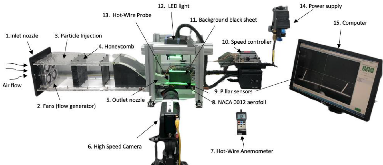
Figure 5. Experimental setup of the calibration tunnel, showing different components for various calibration related tests.
