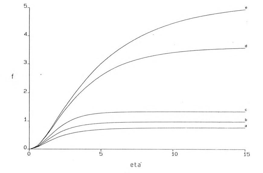
Figure 3.2 Graph of f' against  $\eta$  for  $\sigma = 0.028(a)$ , 0.1(b), 0.72(c), 8.1(d), 17.2(e).
