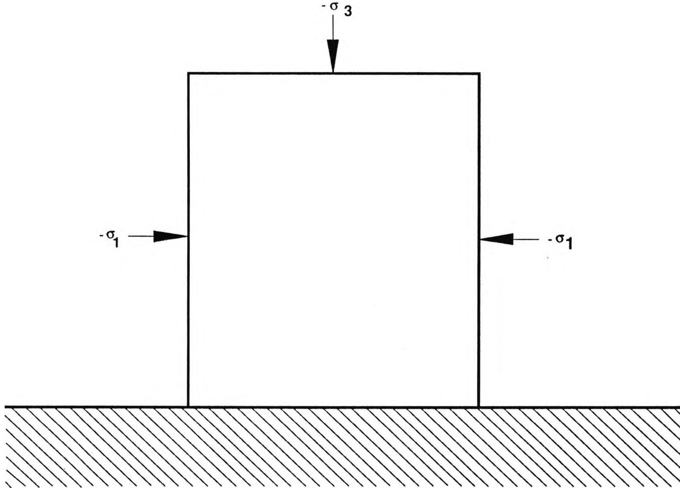
FIG. 9. SCHEMATIC OF EXPERIMENTAL STRESS CONFIGURATION (AFTER WILKINS).
