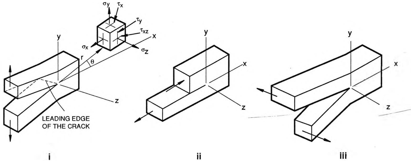
FIG. 1. BASIC MODES OF CRACK LOADING :
