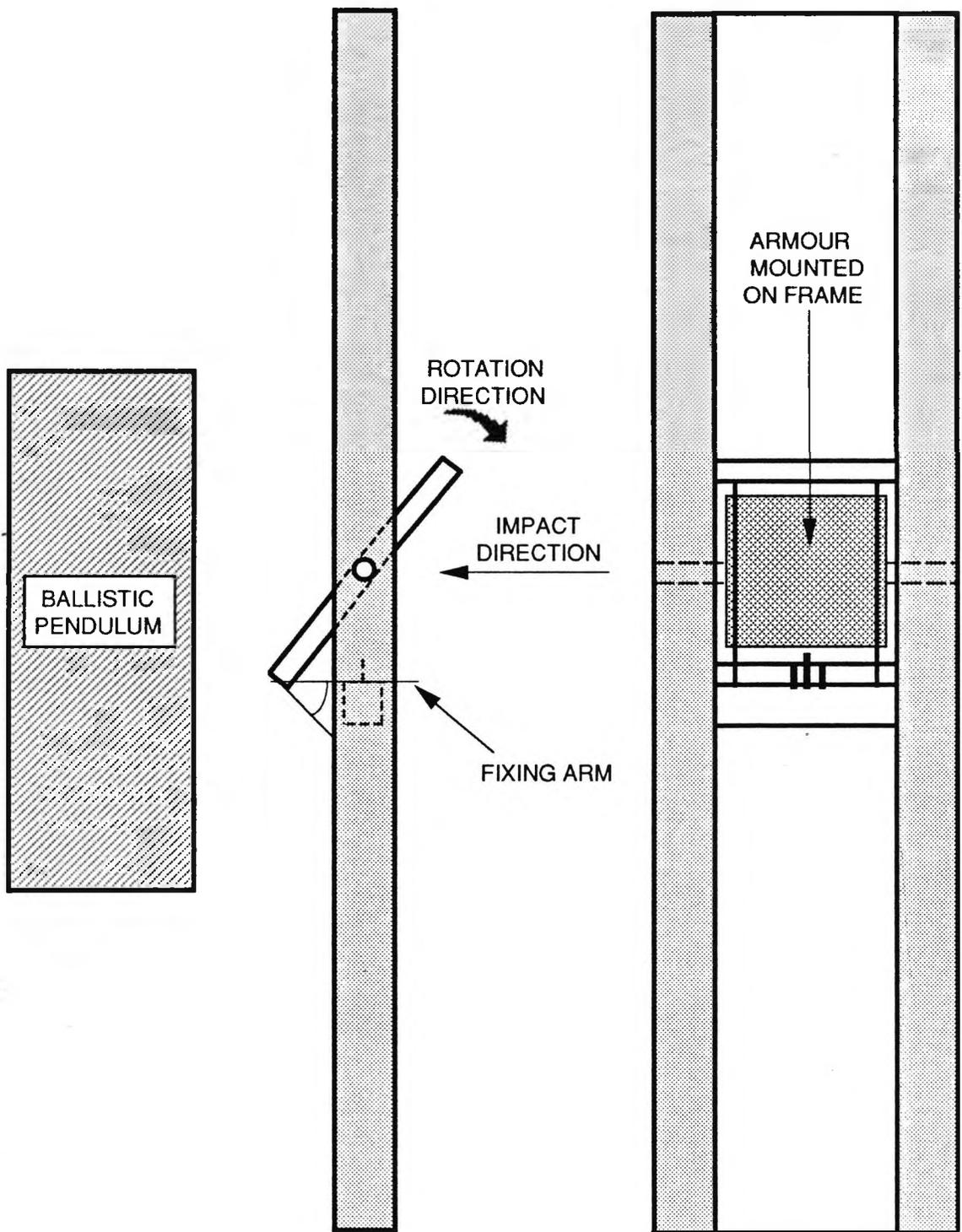
**FIG. 24. FRAME FOR SUPPORT OF ARMOUR DURING TESTING AT OBLIQUE ANGLES OF ATTACK.**
