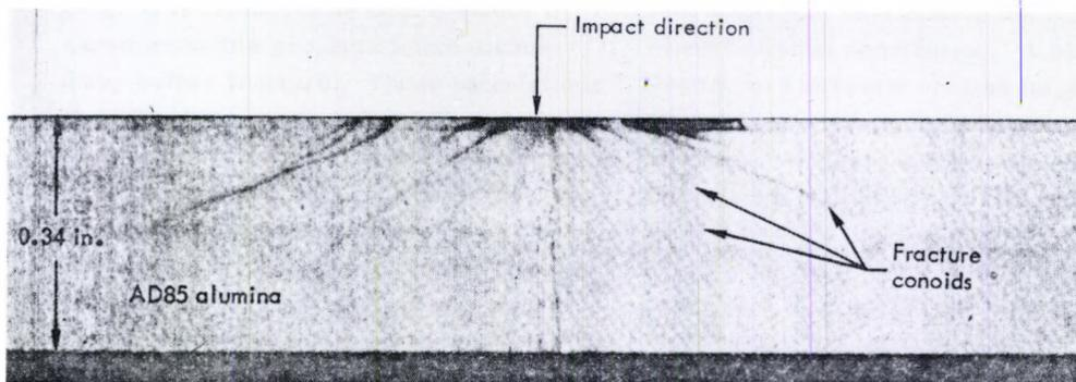
**FIG. 7. SECTION VIEW OF RIGID CERAMIC STRUCK BY A SHARP STEEL PROJECTILE AT 2300 ft/sec. (AFTER WILKINS).**
