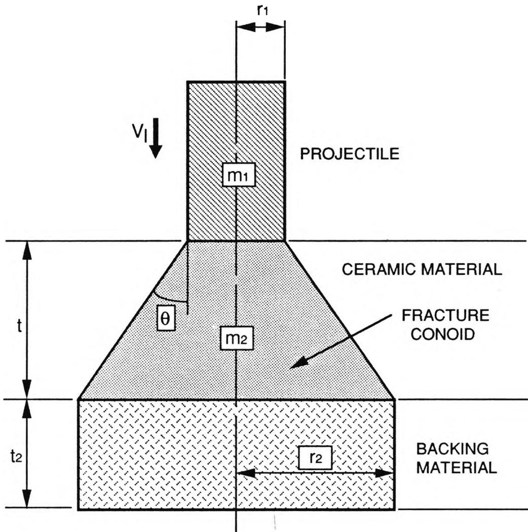
FOR A GIVEN CONOID SEMI - ANGLE  $\theta$  THE AREA OVER WHICH ENERGY IS ABSORBED IS PROPORTIONAL TO THE SQUARE OF THE CERAMIC THICKNESS  $t_1$ . MATERIALS HAVING A GREATER THICKNESS FOR A GIVEN AREAL DENSITY (i.e. LOWER DENSITY) WILL BE POTENTIALLY BETTER ARMOURS
