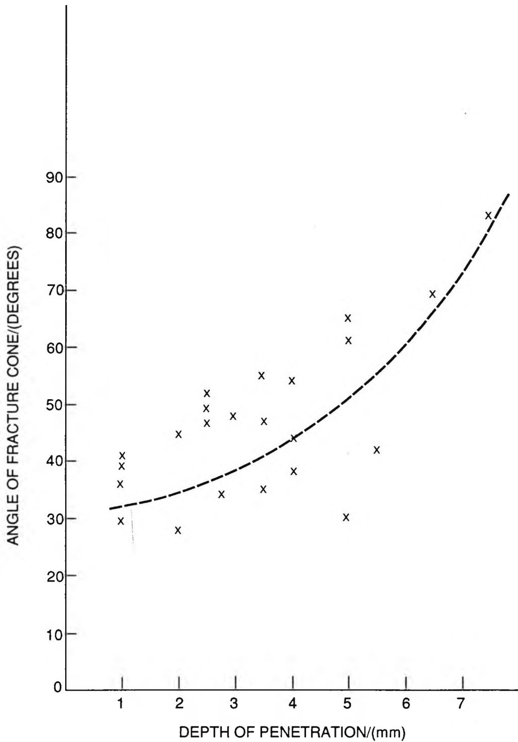
**FIG. 54. FRACTURE CONE ANGLE v DEPTH OF PENETRATION.**
