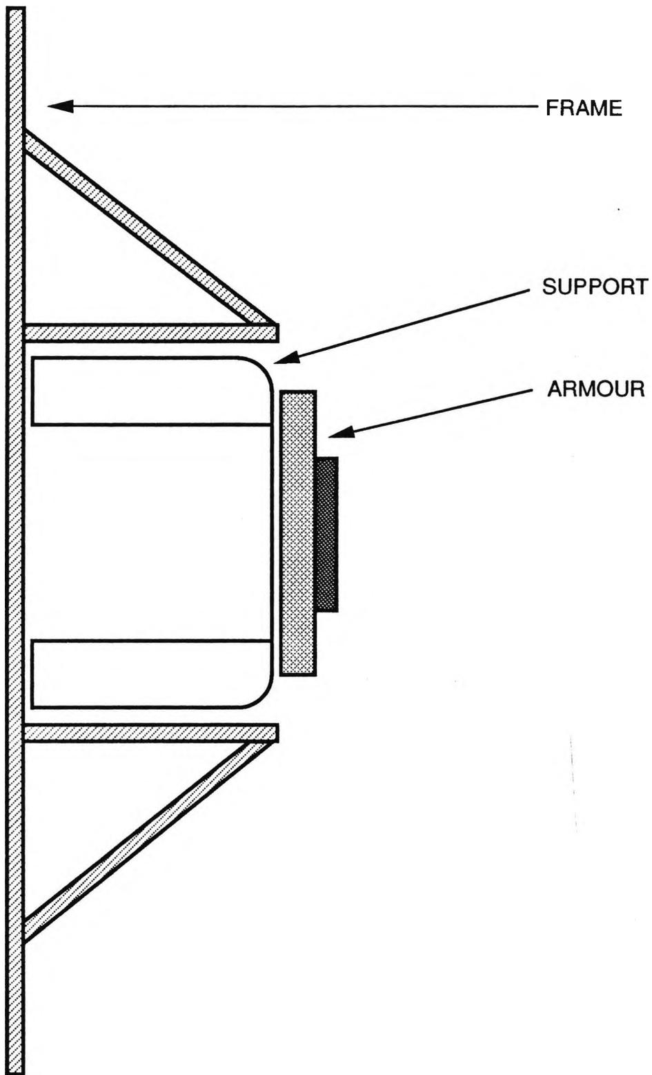
FIG. 23. FRAME FOR SUPPORT OF ARMOUR
