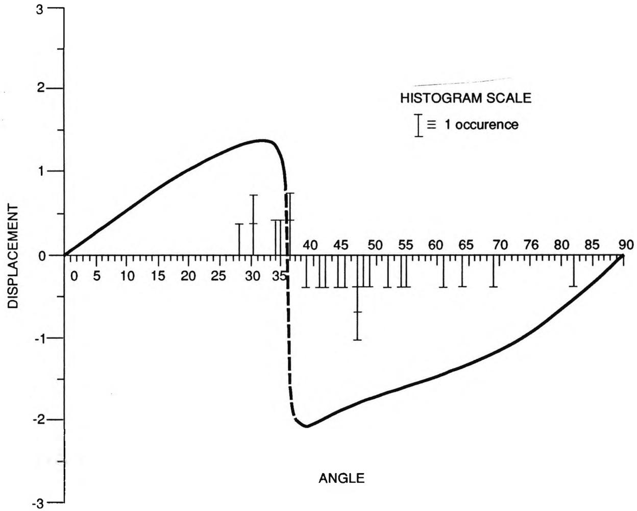
**FIG. 52. DISPLACEMENT OF SHEAR WAVE v ANGLE.**
