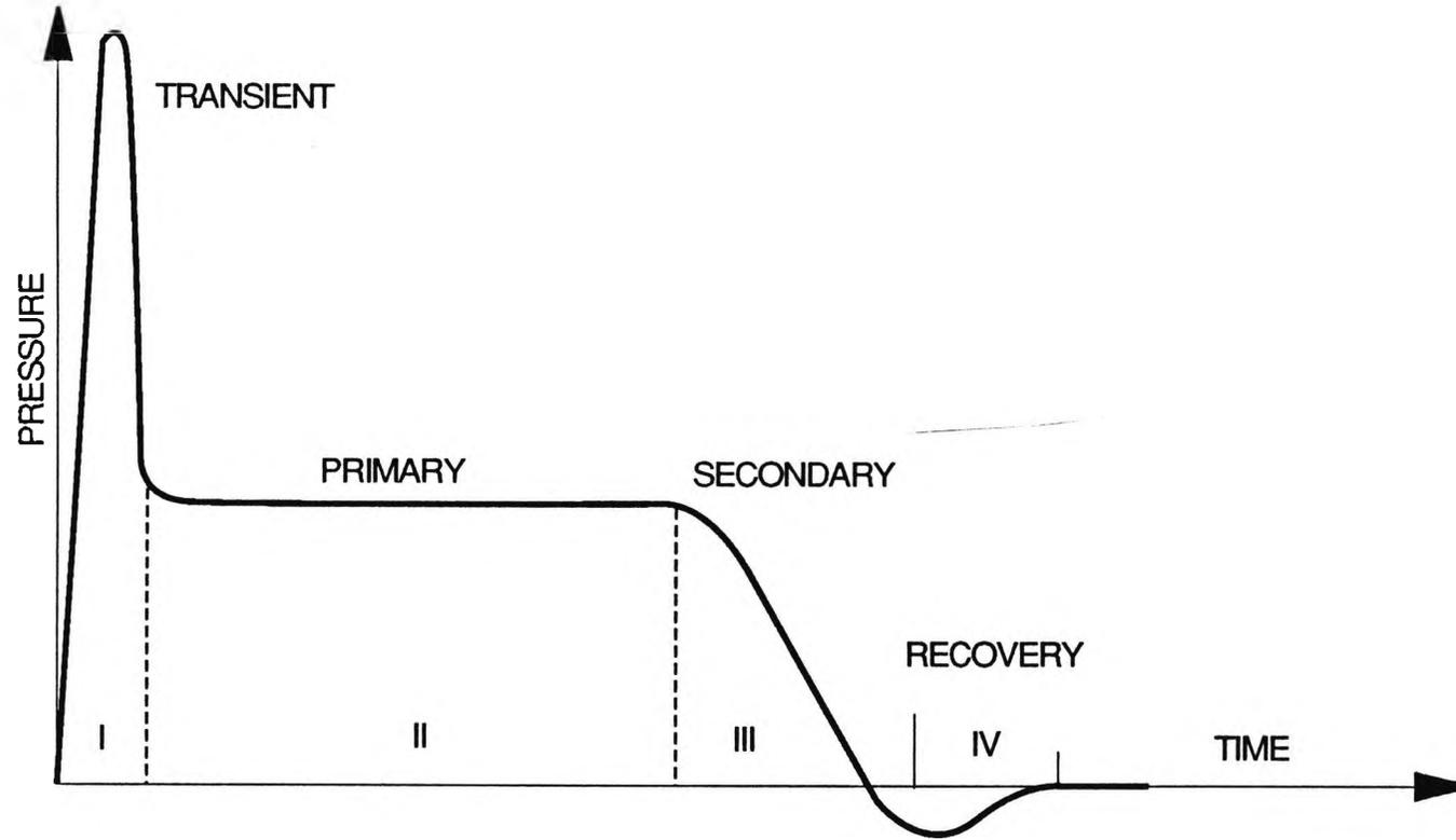
**FIG. 10. SCHEMATIC PRESSURE-TIME PRESENTATION OF THE FOUR PHASES OF HIGH VELOCITY PENETRATION (AFTER HOHLER & STILP).**
