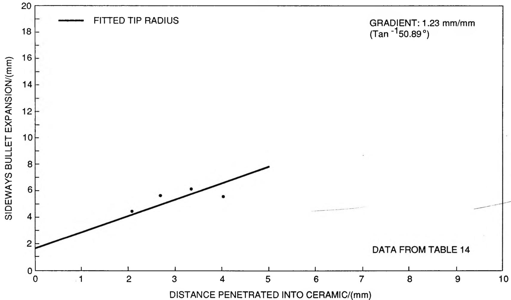
**FIG. 44. SPREADING OF BULLET TIP AS IT PENETRATES THE ALUMINA FACING (WITH GRP BACKING).**
