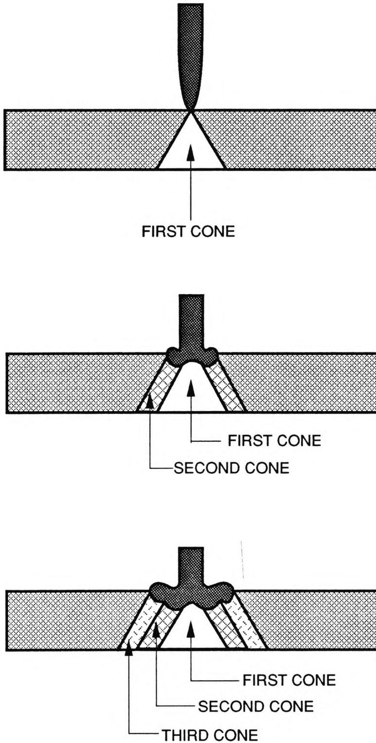
**FIG. 55. DIAGRAM OF FRACTURE CONE AND BULLET PENETRATING.**
