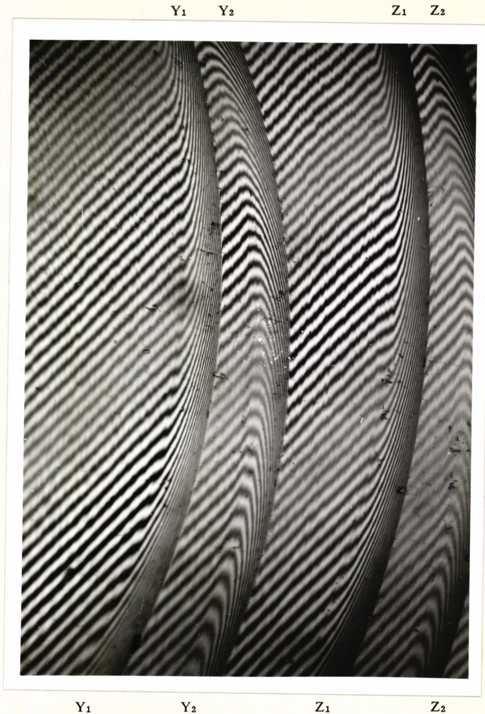
Figure 3.1-6 An interference micrograph of the surface of a rigid diffractive BCL. Everything is doubled by the Wollaston prism, including the dust particles (e.g. the two dark oval shaped spots in the bottom left corner). Two complete DZJ (each seen as the two curved, vertical lines, labelled Y and Z) are shown. As shown diagrammatically in Figure 3.1-5 the interference fringes (diagonal stripes) are displaced vertically (up) by the DZJ at e.g. Y_1 (first wavefront in Figure 3.1-3 ) and then return at e.g. Y_2 (down, at the DZJ of the second wavefront) to lie as a continuation of the original position of the fringe. The relative displacement of the fringe represents the height of the surface feature, in this case the DZJ.
