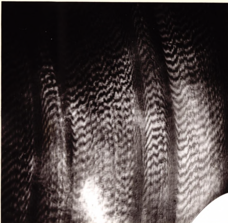
Figure 4.1-12 An interference micrograph of the BCL rated grade 4 (variations >0.27 \mu\text{m} i.e. 1 fringe width).
