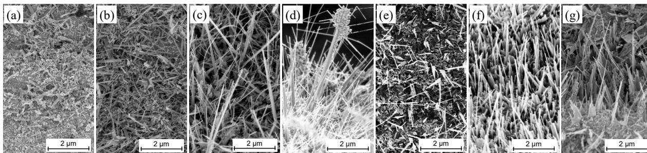
Fig. 1: FESEM images of brass (Cu - 37.2 wt% Zn) wires oxidized in the presence of 5% O<sub>2</sub> in N<sub>2</sub> flown at a rate of 200 sccm at temperatures of (a) 300 °C, (b) 350 °C, (c) 400 °C, (d) 450 °C, (e) 500 °C, (f) 550 °C, and (g) 600 °C.
