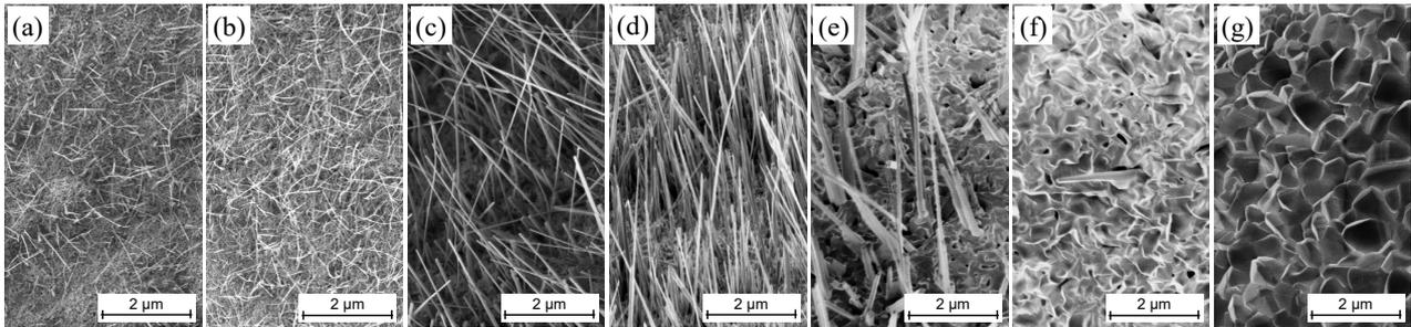
Fig. 3: FESEM images of Cu wires oxidized in ambient at temperatures of (a)  $300 \text{ }^\circ\text{C}$ , (b)  $350 \text{ }^\circ\text{C}$ , (c)  $400 \text{ }^\circ\text{C}$ , (d)  $450 \text{ }^\circ\text{C}$ , (e)  $500 \text{ }^\circ\text{C}$ , (f)  $550 \text{ }^\circ\text{C}$ , and (g)  $600 \text{ }^\circ\text{C}$ .
