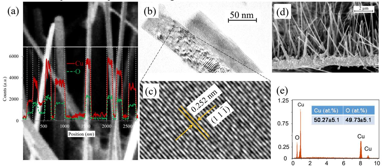
Fig. 4: (a) FESEM image of CuO nanowires grown at  $450 \text{ }^\circ\text{C}$  and corresponding elemental line scanning, (b, c) bright-field TEM image of nanowires and corresponding HRTEM image, (d, e) exfoliated oxidized layer in cross-sectional view and corresponding EDX spot analysis.
