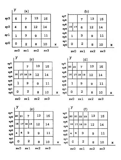
Figure 2. z-hashing splitting sequence.
