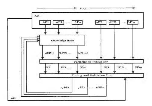
Figure 4.41 The Framework for System Tuning.
