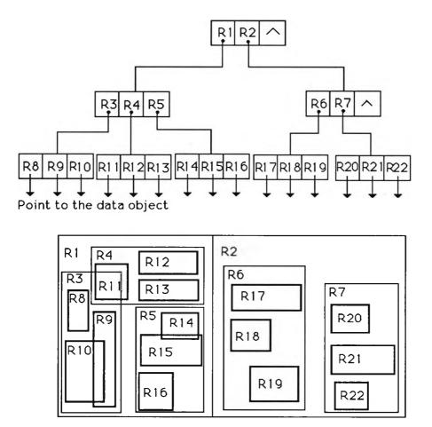
Figure 4.26. The R-tree algorithm.
