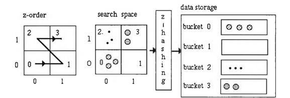
Figure 4.14.(a) Binary code z-hashing algorithm.
