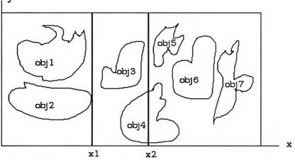
Figure 4.24. Multi-layered 2-d grid partition.
