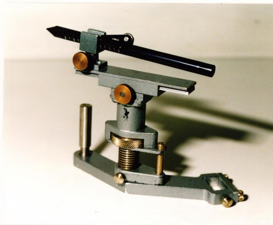
**Figure 2.** A Cochet-Bonnet aesthesiometer attached to an applicator which allows precise manipulation of the orientation of the aesthesiometer.
