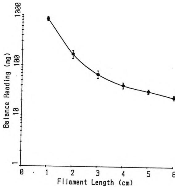
Figure 72. Calibration curve for the Cochet-Bonnet aesthesiometer
