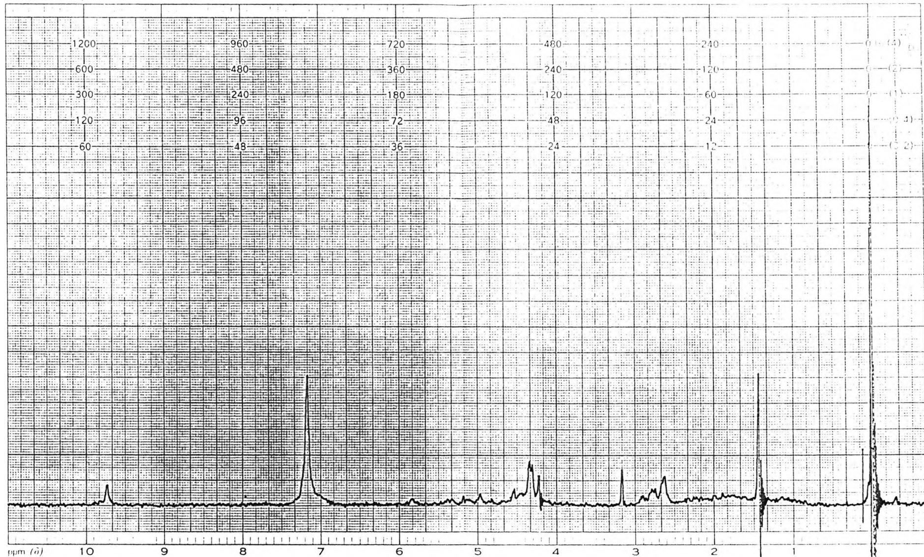
Fig. 3.25:  $^1\text{H}$  n.m.r. ( $\text{CDCl}_3$ ) spectrum of 1-dodecene
