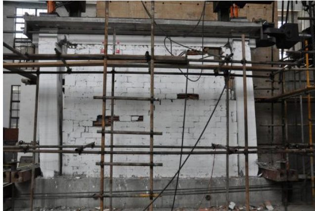
Figure 6 Damage of Specimen 3 at R = 4%
