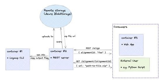
Figure 1: High level overview of container configuration and intercommunication
