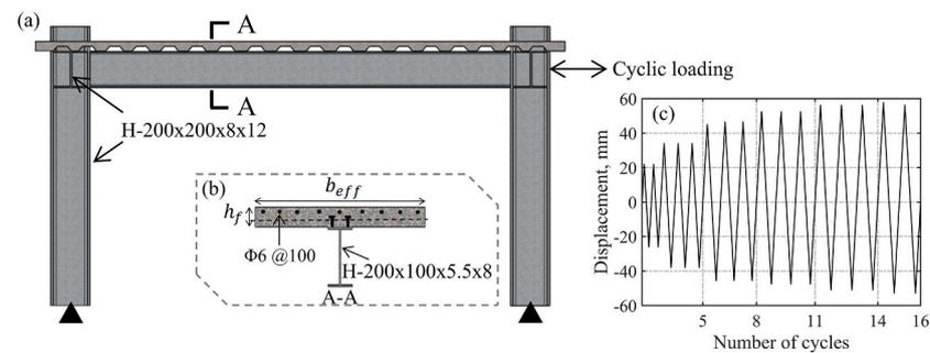
Fig. 5. Schematic test details of CS3 [49]: a) test configuration, b) composite beam cross-section, and c) applied loading history.
