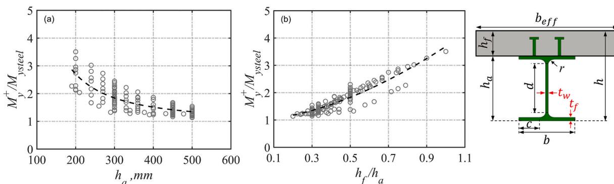
Fig. 23. Ratio of yield strength of composite beam to that of steel beam under positive bending vs: a)  $h_a$  and b)  $h_f/h_a$ .
