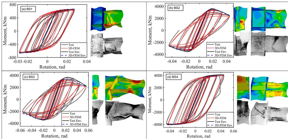
Fig. 10. Comparison between experimental and numerical results for (a) BS1, (b) BS2, (c) BS3, and (d) BS4.
