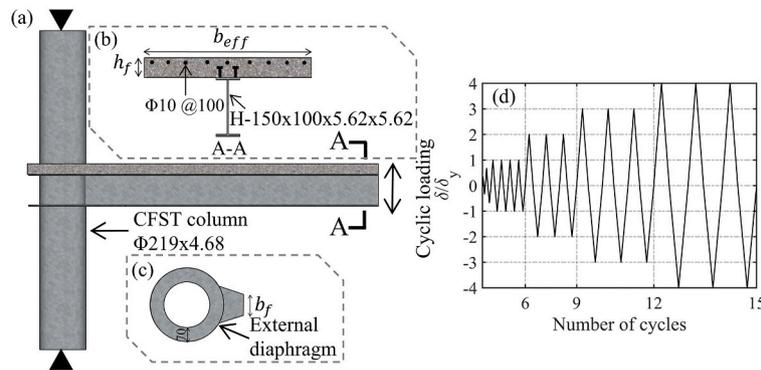
Fig. 6. Schematic test details of CS4 [50]: a) test configuration, b) composite beam cross-section, c) connection details, and d) applied loading history.
