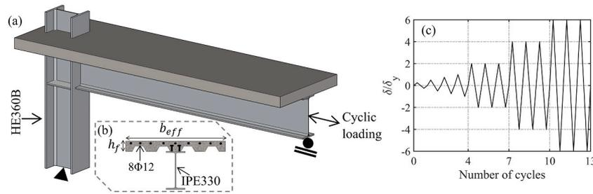
Fig. 3. Schematic test details of CS1 [47]: a) test configuration, b) composite beam cross-section, and c) applied loading history.
