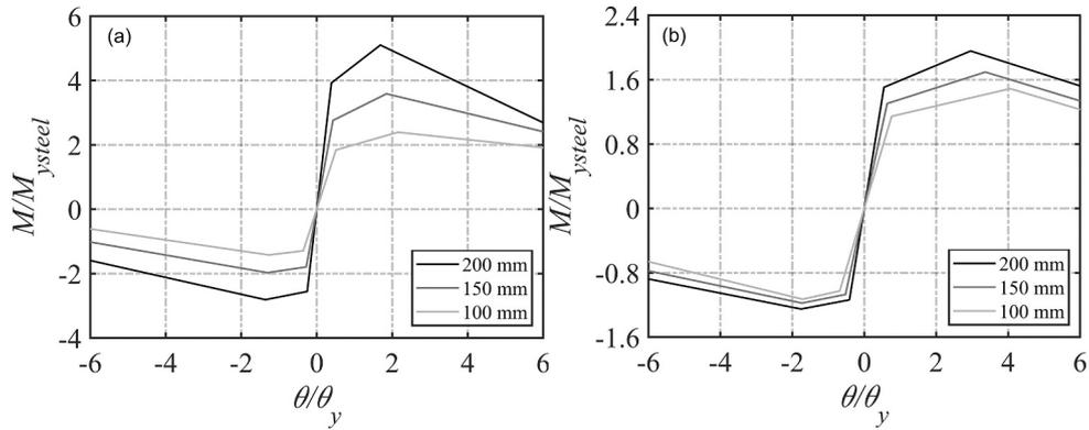
Fig. 27. Examples of backbone curves for various slab thicknesses,  $h_f$ , (as 200 mm, 150 mm, and 100 mm) plotted via proposed formulations: a) IPE200, and b) IPE500.
