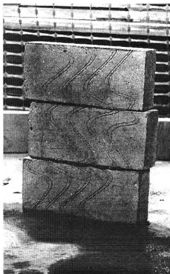
Figure 8.15 Three blocks assemblies with the middle block offset
