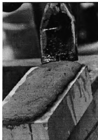
Figure 3.8.3 Nozzle attached to the delivery pipe of the pump
