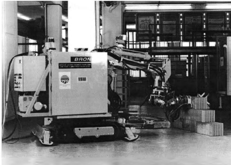
Figure 2.4 Mobile robot for masonry construction at the University of Stuttgart
