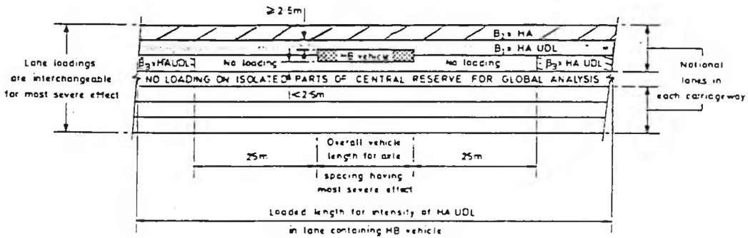
FIGURE 5.7. LOADING SCENARIOS FOR HB LOADING AND ASSOCIATED HA LOADING (BD 37/88, 1989).
