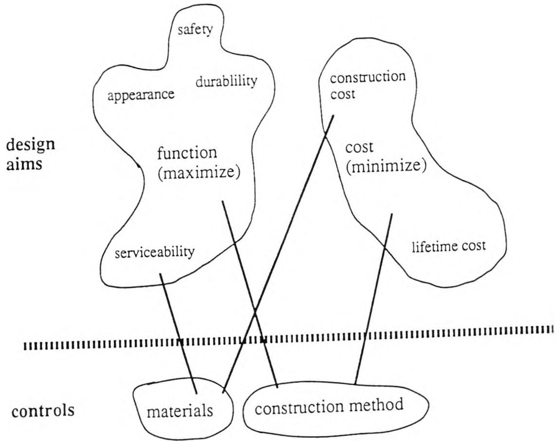
**FIGURE 2.1. A REPRESENTATION OF BRIDGE DESIGN SPACE.**
