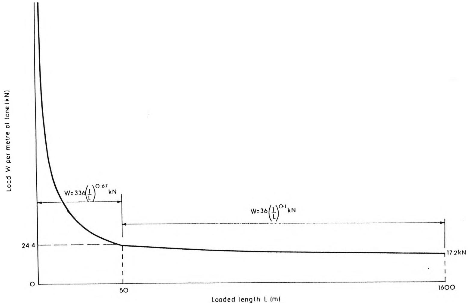
FIGURE 5.4. LOADING CURVE FOR HA UDL (NOT TO SCALE)
