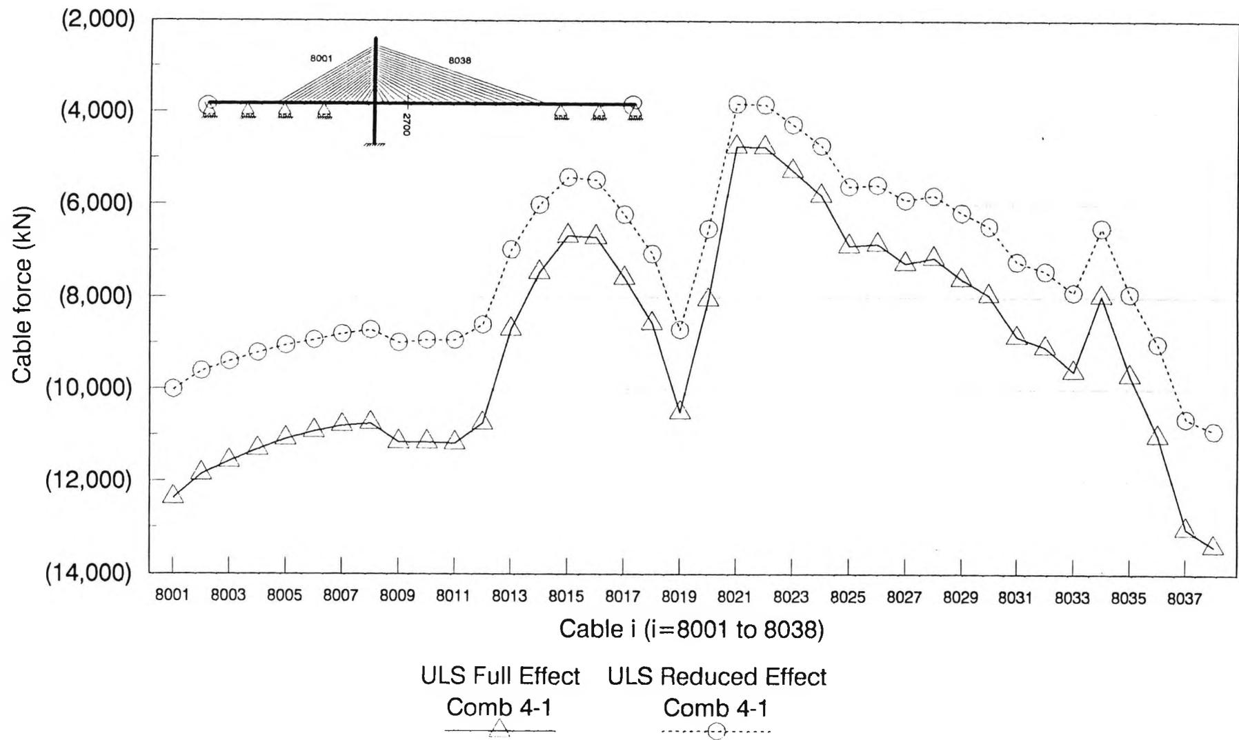
FIGURE 6.4. FORCES DEVELOPED IN CABLES AT THE INITIAL STAGE (i.e. NO CABLE OUT).
