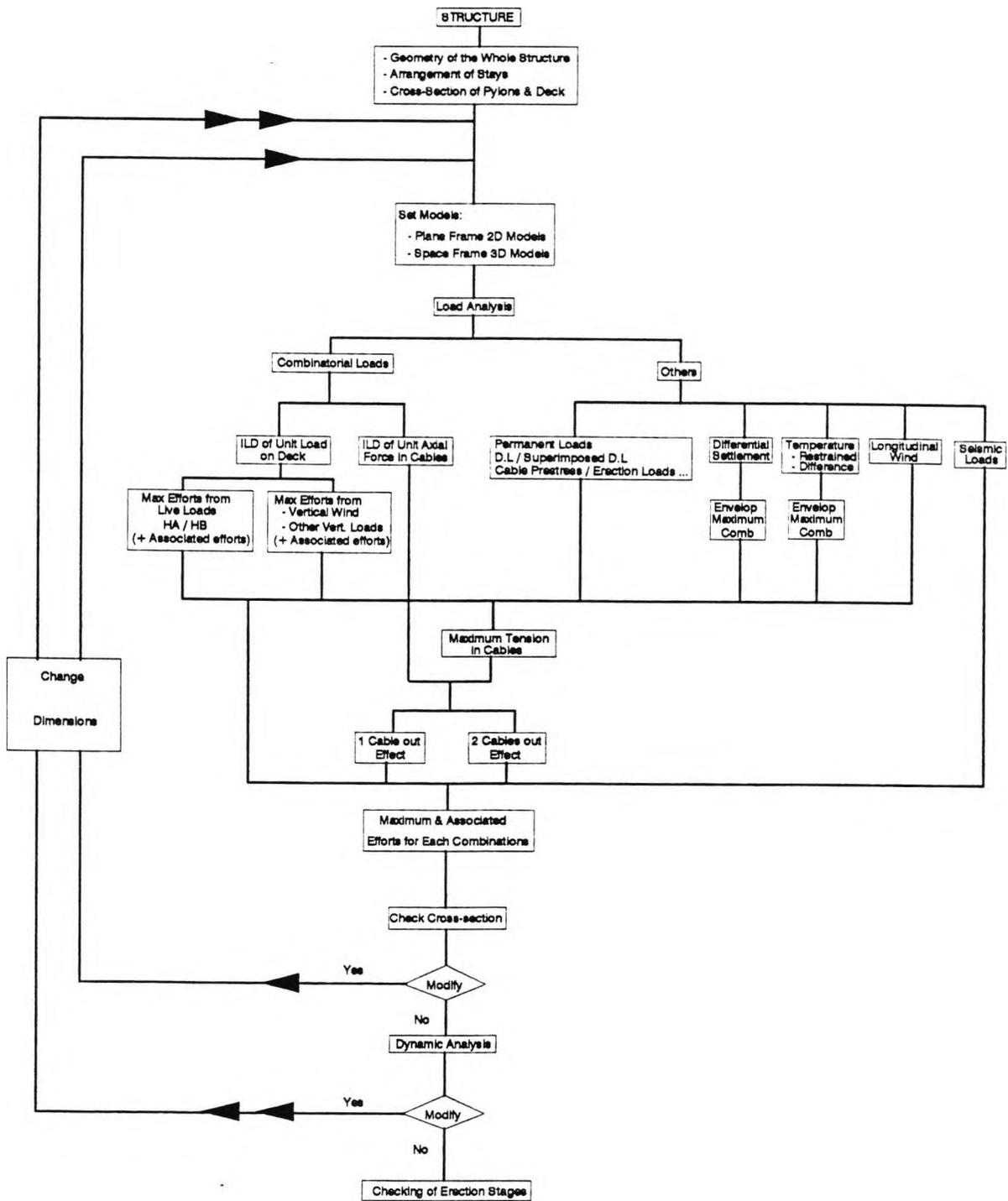
FIGURE 6.1. DESIGN AND ANALYSIS CONCEPT OF CABLE-STAYED BRIDGES SUBJECT TO CABLES OUT CONDITIONS.
