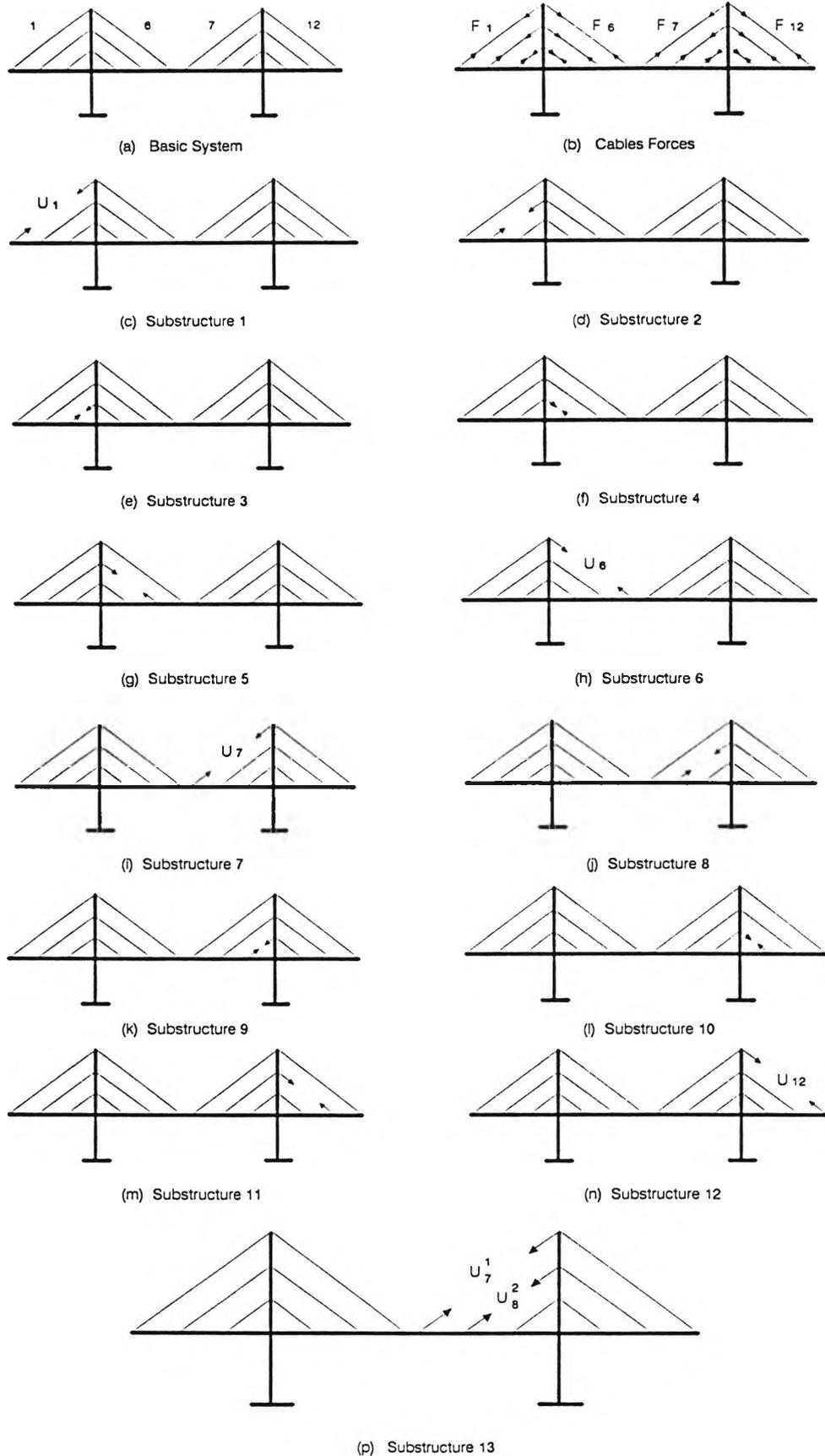
FIGURE 6.2. CABLE STAYED BRIDGE UNDER DIFFERENT STAY CONDITIONS.
