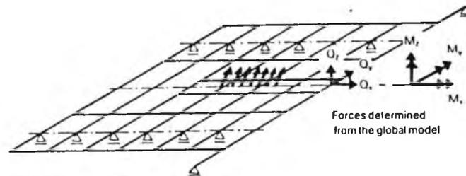
(b) DUSSELDORF-FELHE BRIDGE: PARTIAL MODEL (GRID-WORK MODEL) INTENDED FOR THE DESIGN OF THE ANCHORAGE ZONE OF THE STAYS IN THE DECK.
