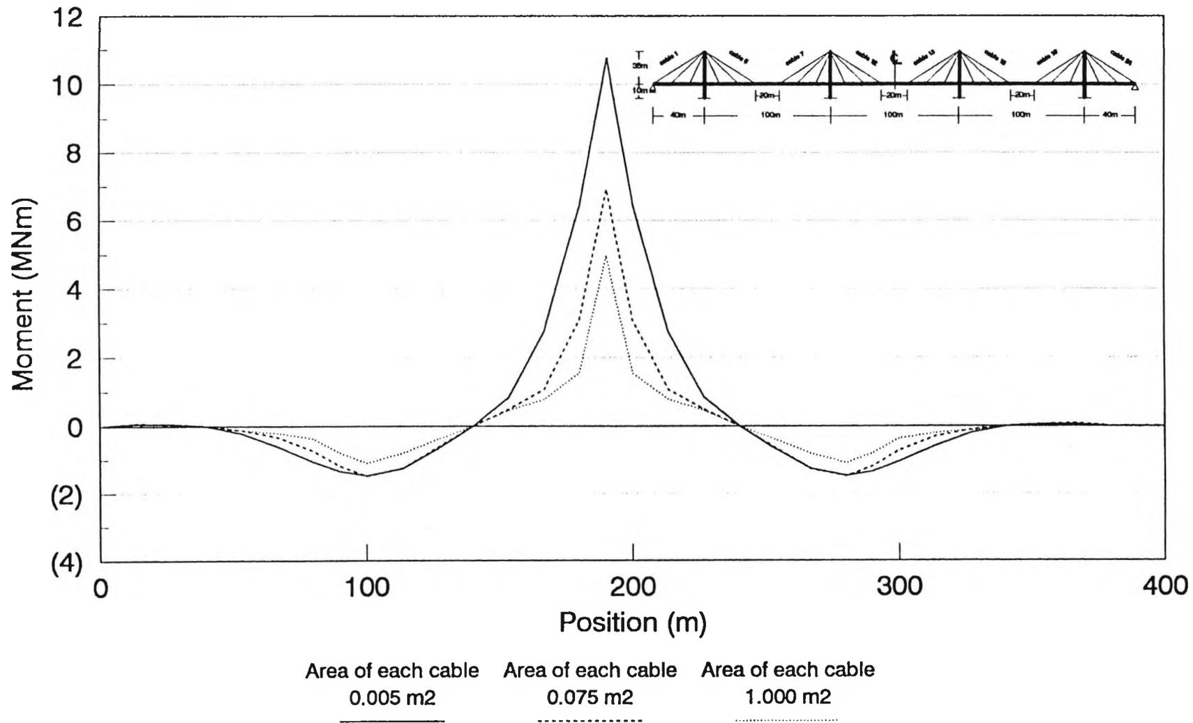
FIGURE 5.2. VARIATION OF ILD FOR MOMENT WITH CABLES STIFFNESSES.
