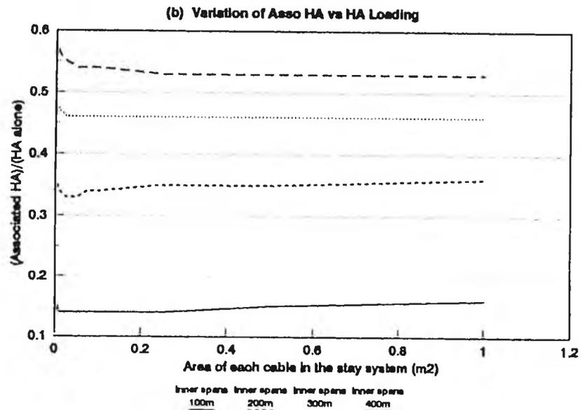
FIGURE 5.19. VARIATION IN LIVE LOAD RATIO FOR FOUR CABLE-STAYED BRIDGES WITH DIFFERENT SPANS ARRANGEMENT.
