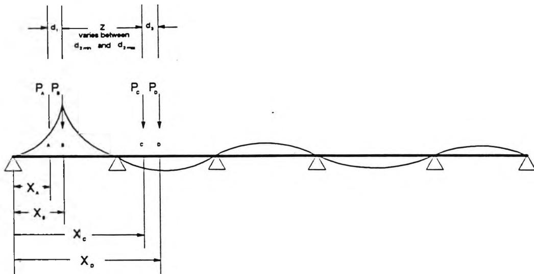
FIGURE 5.9. INFLUENCE LINE LOADED WITH AN HB VEHICLE.
