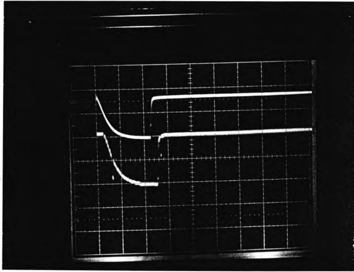
Fig. 7.12 'Disintegrated' output (lower trace) of the ADC-FOL-DAC due to ADC driver instability. Upper trace is the input to the ADC.  $\rightarrow 1 \mu\text{s}/\text{div.}$  and  $\uparrow 50 \text{ mV}/\text{div.}$
