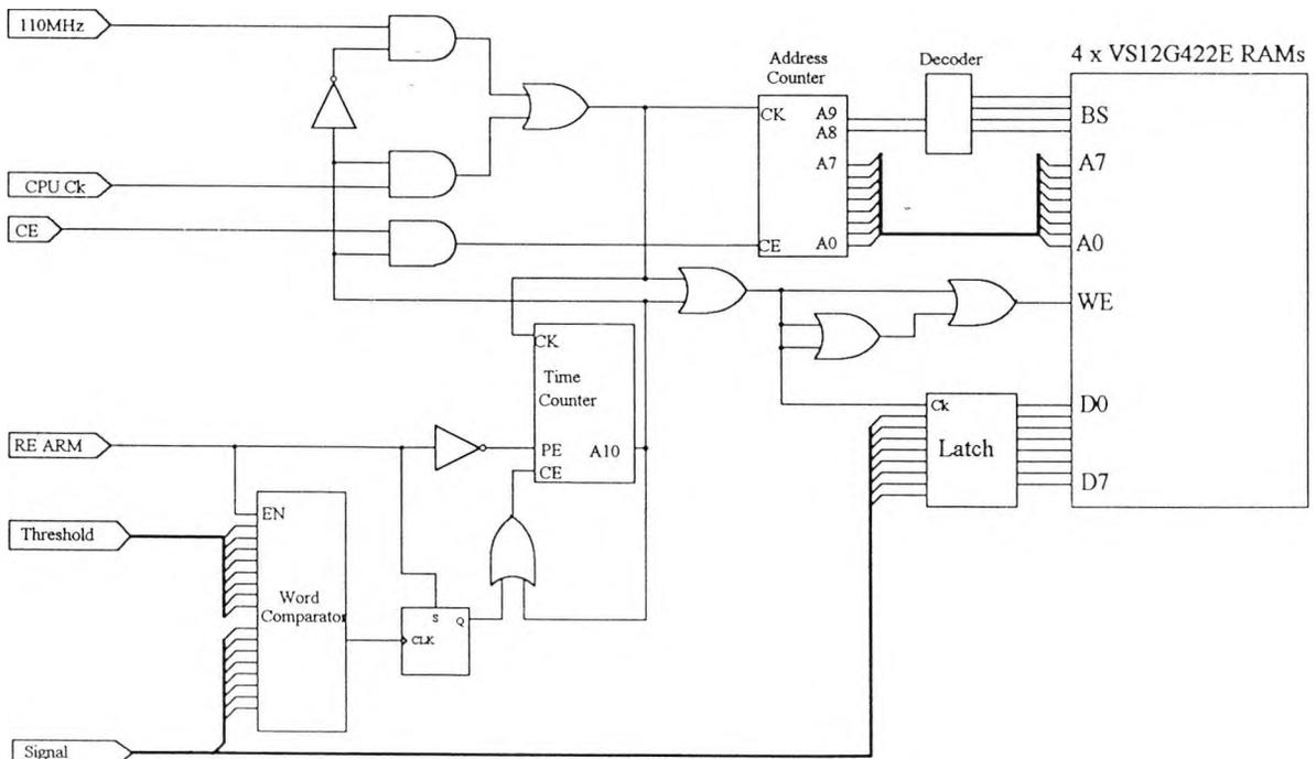
Fig 5.6 Circuit for VS12G422E RAMs
