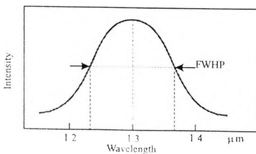
Figure 4.8 LED output spectrum
