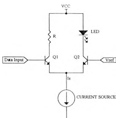
FIG. 4 15 Current-Routing Configuration
