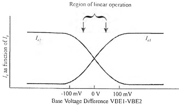
Figure 4.16 Current-routing transfer characteristics
