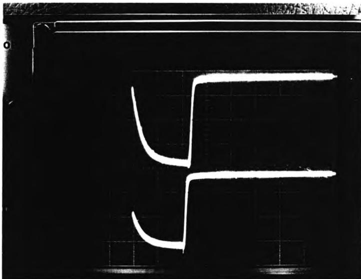
Fig. 7.9a Chopped-impulse input to the ADC (lower trace) and the corresponding output (upper trace) of the ADC-FOL-DAC. (  $\uparrow$  0.1 V/div,  $\rightarrow$  1  $\mu$ s/div )
