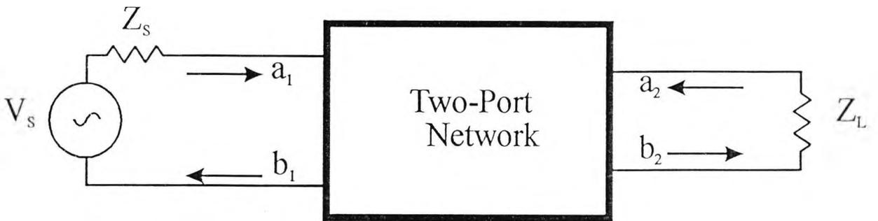
Figure 4.27 Two-port network showing incident ( $a_1, a_2$ ) and reflected ( $b_1, b_2$ ) waves used in s-parameter definitions.
