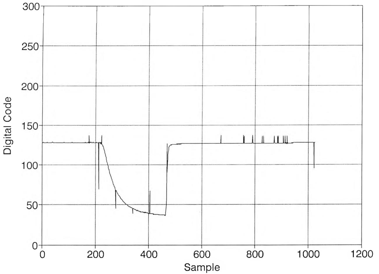
Fig. 7.20 A record of a 'partially disintegrated' chopped impulse captured by the recorder unit.
