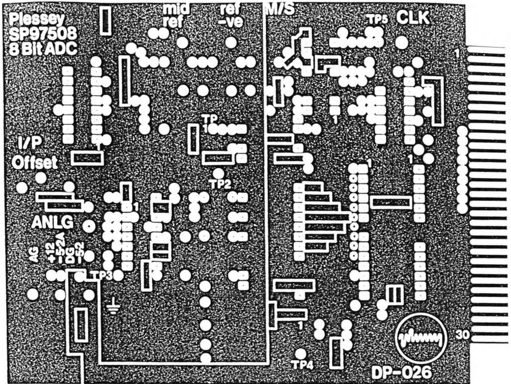
Fig D 2(a) ADC Board (ground plane)
