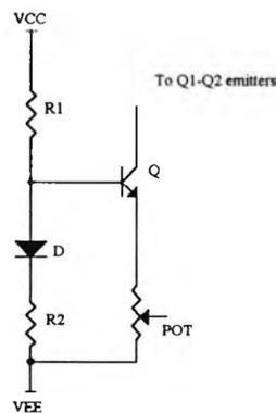
FIG. 4.17 A Transistor Used As A Constant Current Source
