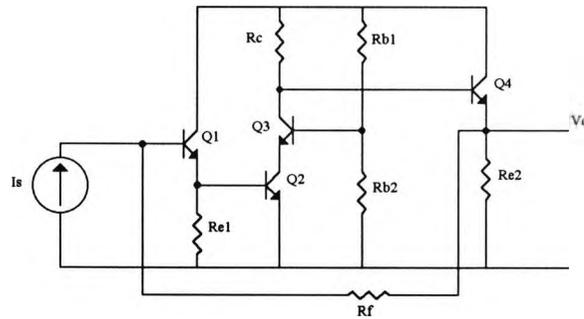
FIG. 4.35 CC-Cascode Configuration
