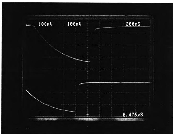
Fig. 7.9b Chopped-impulse input and output of the ADC-FOL-DAC system on a faster time scale. (200 ns/div)
