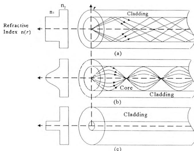
Figure 4.2 Refractive index profile and light propagation through (a) multimode step index (b) multimode graded index and (c) single mode stepindex fibre
