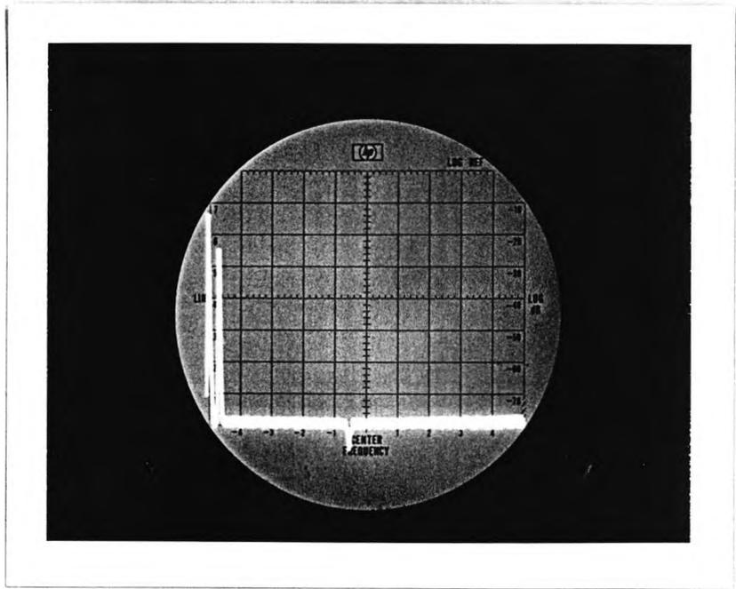
Fig. 7.6 Frequency spectrum of the filtered output of the Marconi generator over the frequency range of 0-100 MHz.
