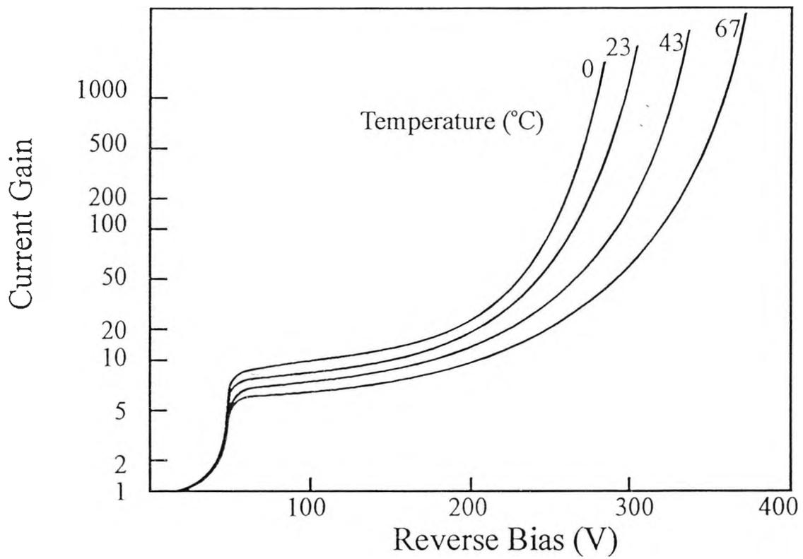
Fig. 4.31 Current gain vs reverse bias for silicon APD
