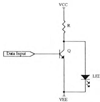
FIG. 4.12 Current shunt LED driver
