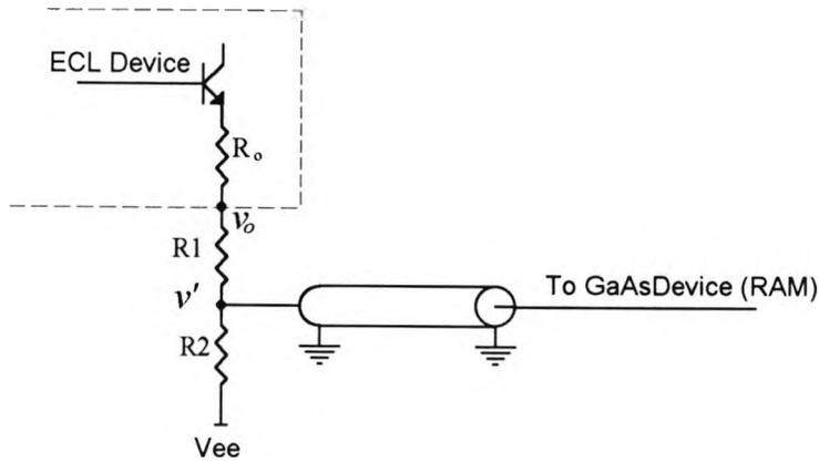
Fig B.1 Arrangement For Matching Standard ECL to GaAs-based Devices
