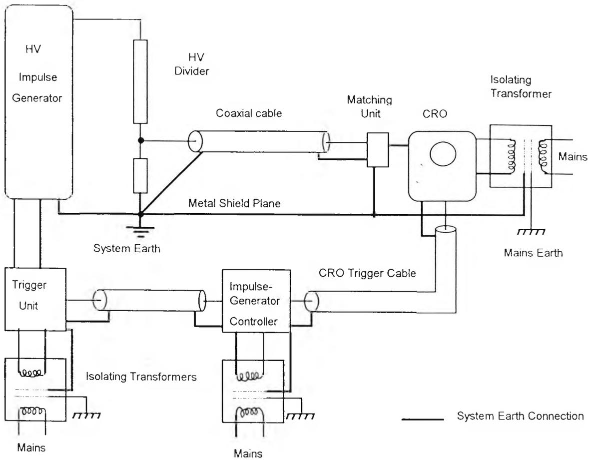
Figure 2.1 HV circuit showing monitoring systems and supplies
