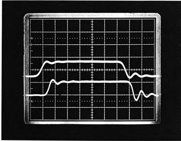
Fig. 4.39a The input (upper trace) and the output (lower trace) of the preamplifier showing the response time of the device. The scale is at 5 ns/div. The input to the preamplifier seem to have a slightly slower rise time but this is due to the loading effect of the preamplifier on the output of the generator.
