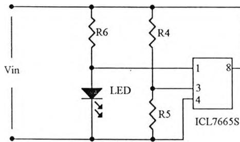
Fig H.2 Low voltage detector
