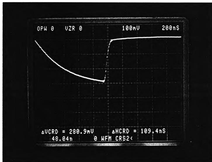
Fig. 7.11b Output of ADC-FOL-DAC; impulse chop time of 109 ns.
