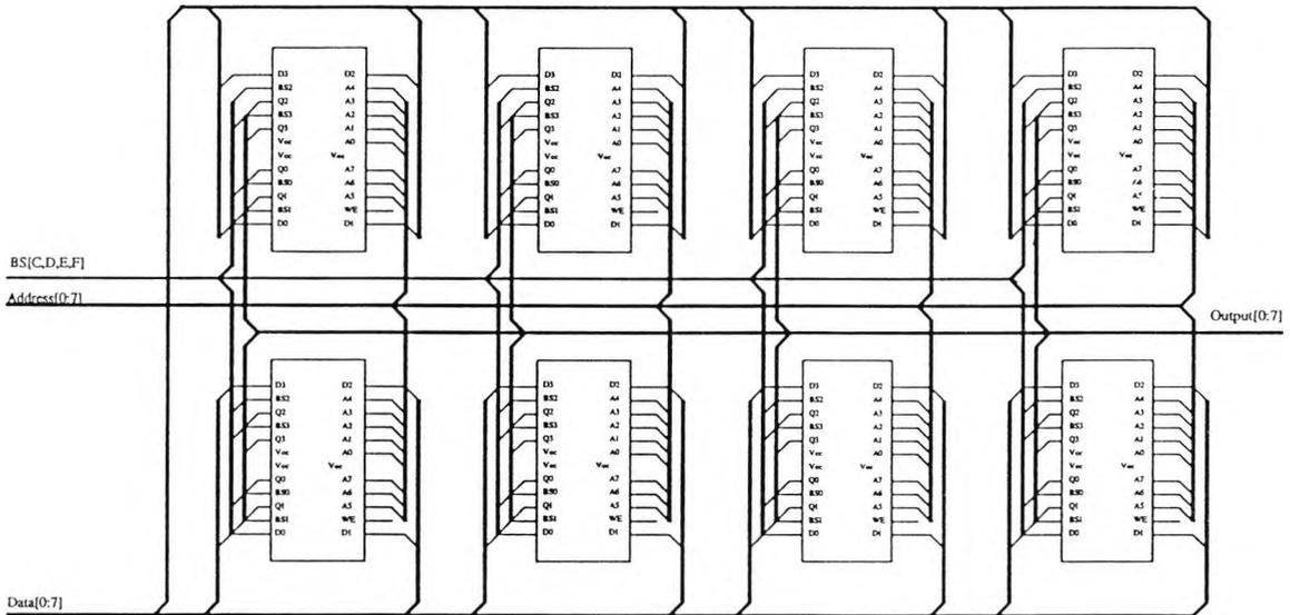
Fig 5.7 Layout for the VS12G422E RAM ICs
