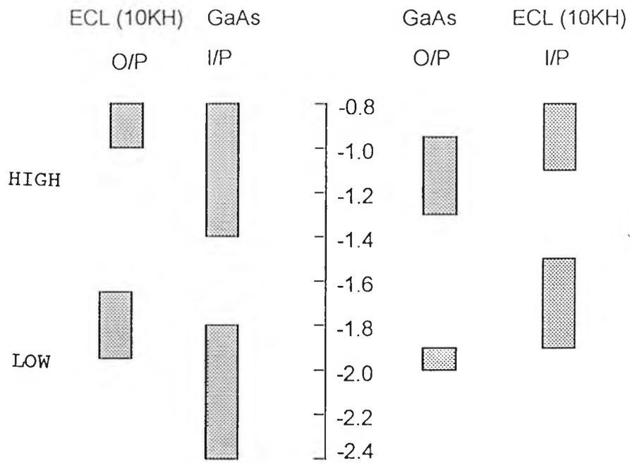
Fig 5.10 ECL and GaAs RAM input/output voltage ranges
