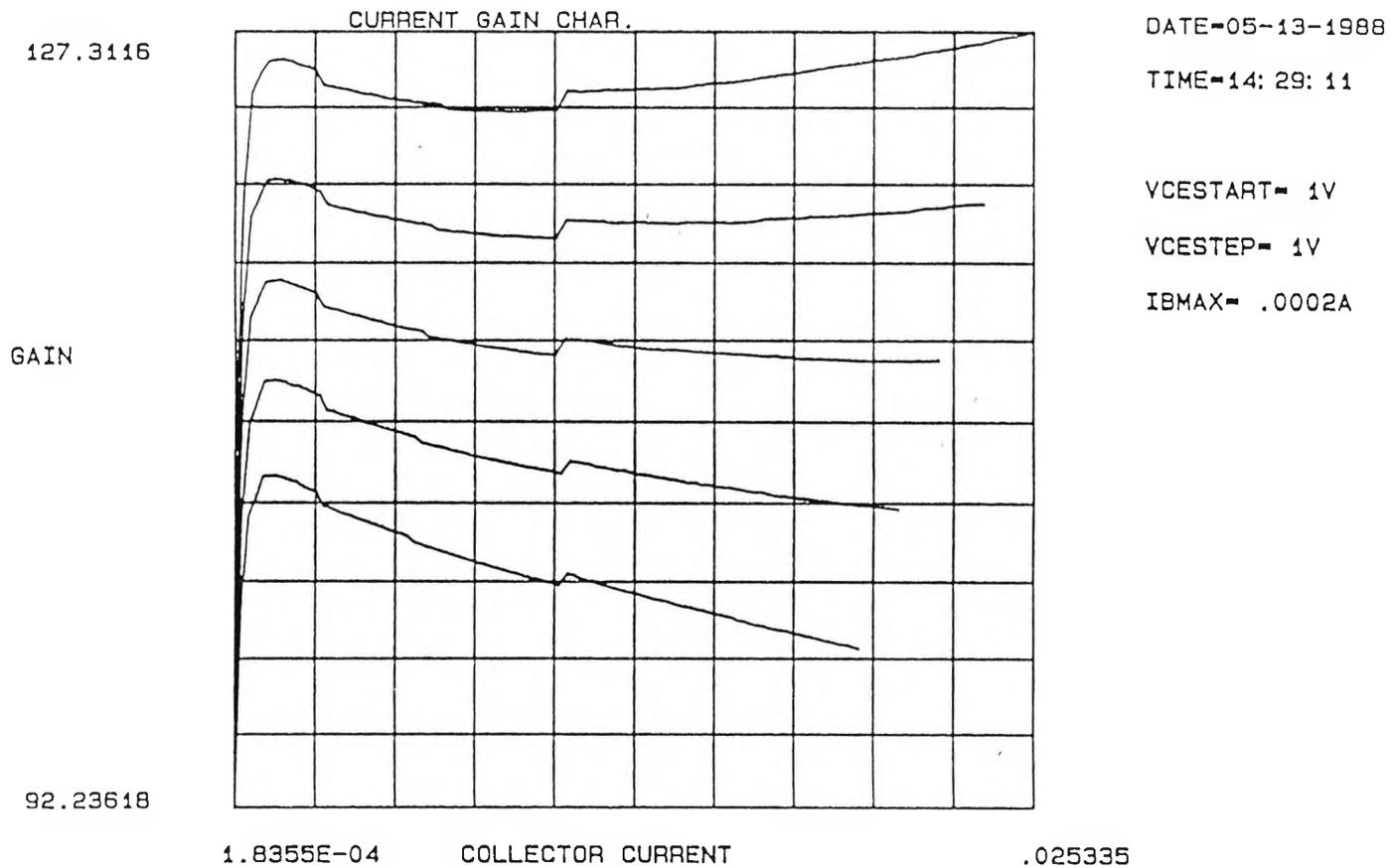
Fig 4 22 Current Gain Characteristics
