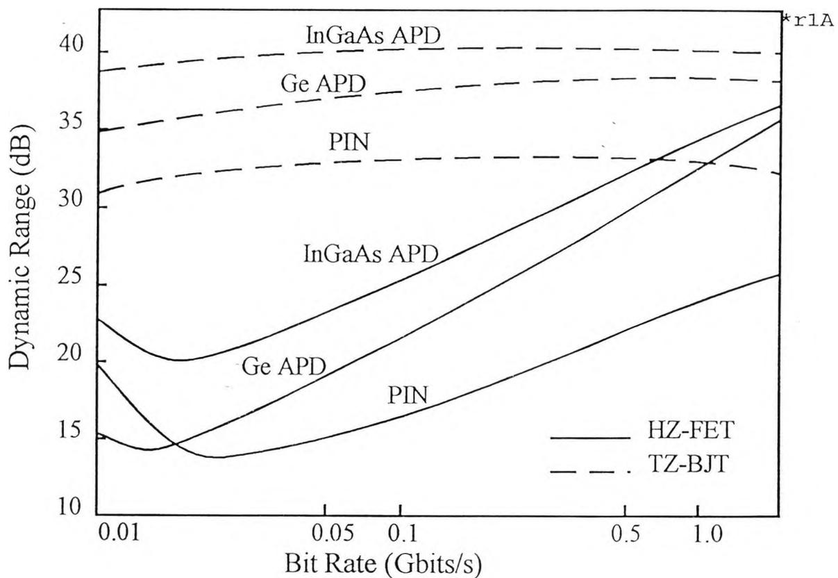
Figure 4.32 Bit range dependence of dynamic range for HZ and TZ designs
