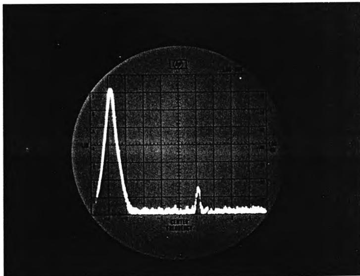
Fig. 7.5 Frequency spectrum of the output of the ADC-FOL-DAC system.
