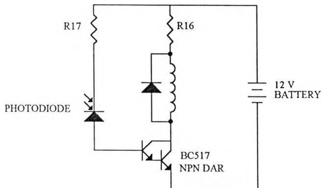
Fig H.3 Optically remote controlled relay circuit diagram
