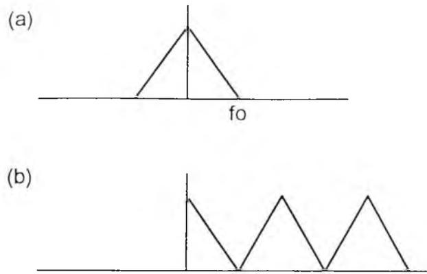
Figure 3.1 Spectrum of (a) Analogue signal (b) Sampled signal
