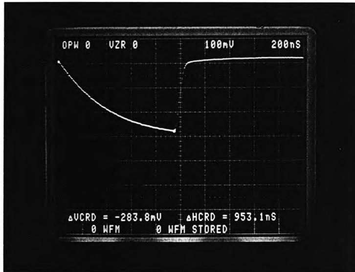
Fig. 7.11a Output of ADC-FOL-DAC; impulse wavefront of 283 mV and rise time of 953 ns.
