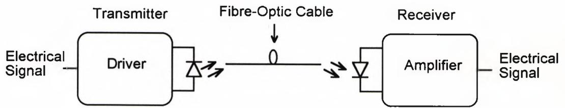
Figure 4.1 Block diagram of Fibre Optic Link
