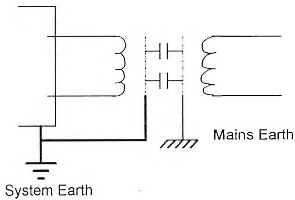
Figure 2.2 Capacitance between the screens of an isolating transformer
