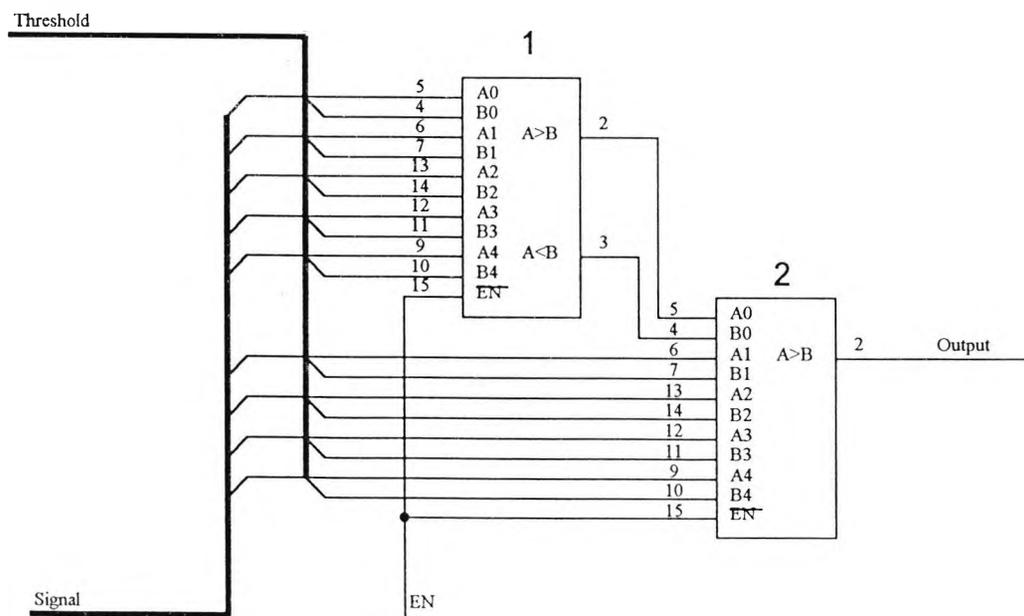
Fig 5.9 Signal Monitoring Circuit
