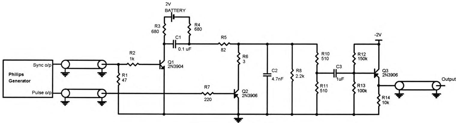
Fig. I.1 Chopped-Impulse Circuit Diagram
