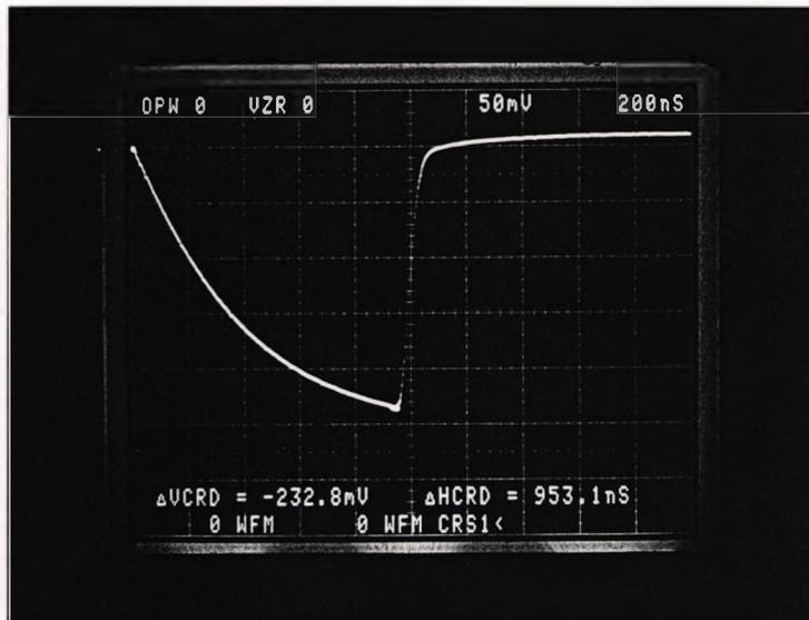
Fig. 7.10a Input to ADC; impulse wavefront of 233 mV peak and rise time of 953 ns
