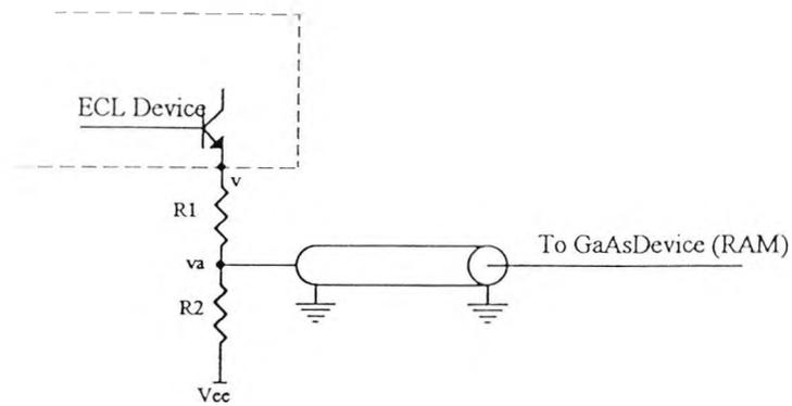
Fig 5.11 ECL-to-GaAs matching circuit
