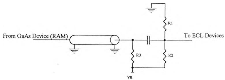
Fig 5.12 GaAs-to-ECL matching circuit
