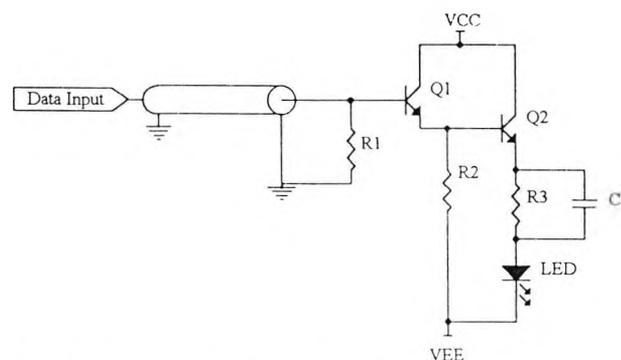
FIG. 4.11 Common collector LED driver
