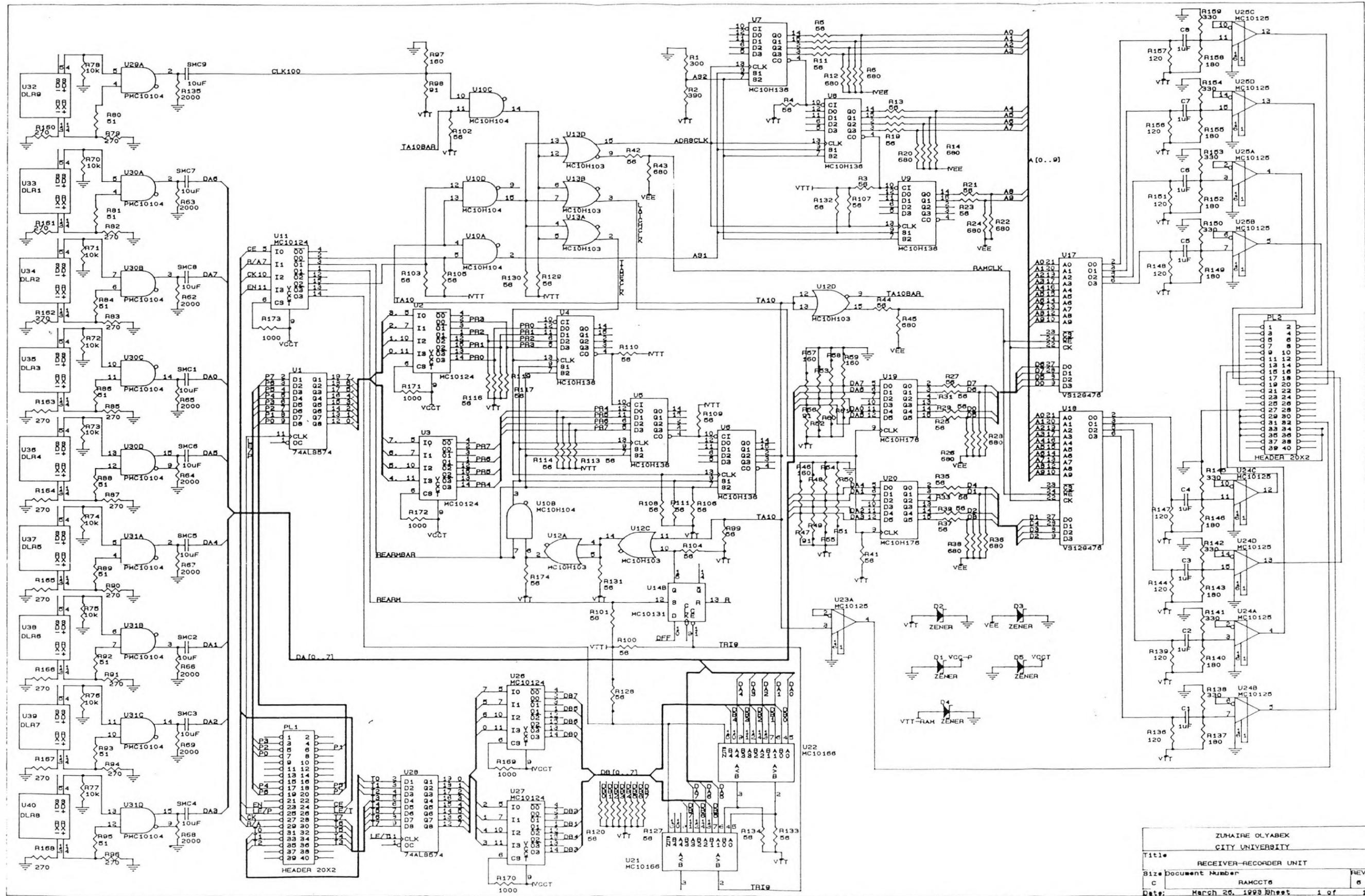
Fig 5.13(b) Complete Circuit Diagram of Recorder Unit
