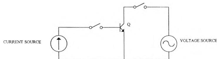
FIG. 4.21 BETA Measurement Arrangement
