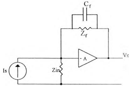
FIG. 4.33 Schematic Diagram of Transimpedance Configuration
