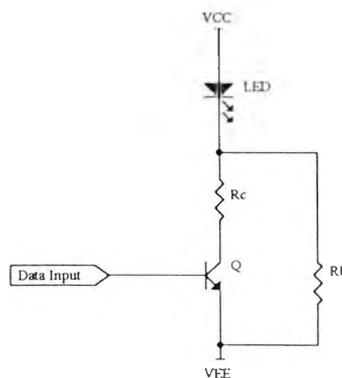
FIG. 4.13 Common emitter type LED driver
