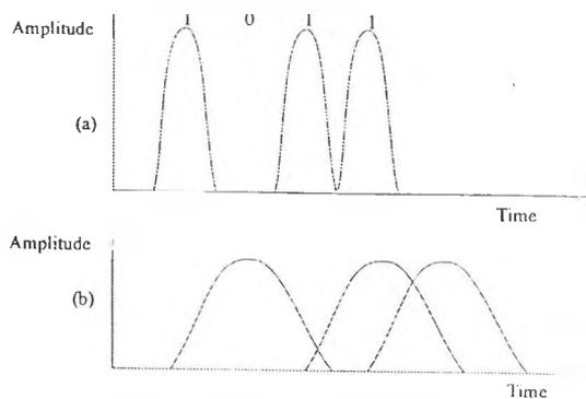
Figure 4.4 Illustration of ISI due to pulse broadening
