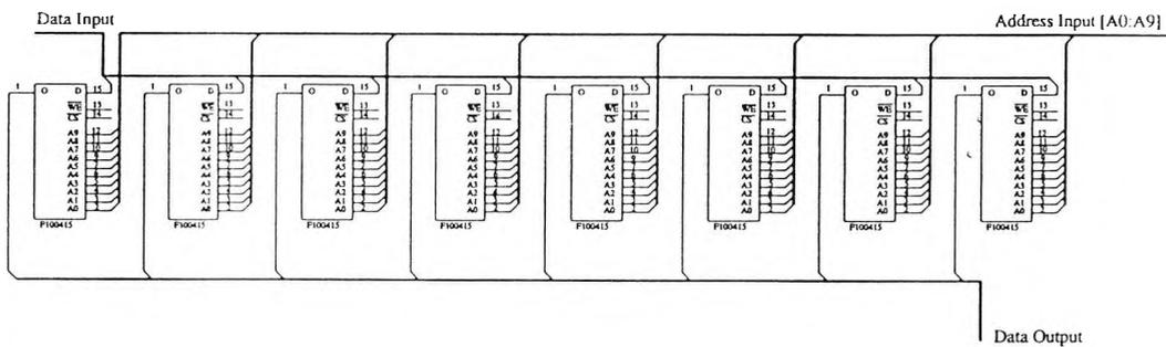
Fig 5.2 One set of RAMs for interleaved system
