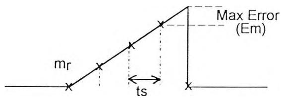
Figure 3.4 Chopped waveform showing worst-case sampling instances
