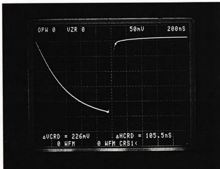
Fig. 7.10b Input to ADC; impulse chop time of 105 ns.
