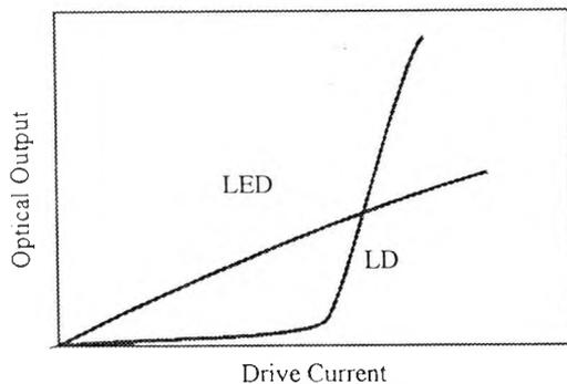
Figure 4.9 I/O Characteristics of LD and LED
