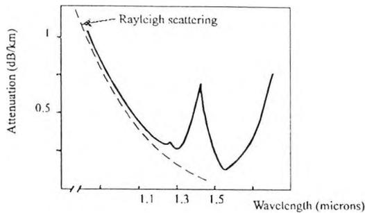
Figure 4.3 Attenuation spectrum of silica-based fibre
