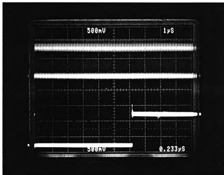
Fig. 7.17 The clock signal (upper trace) and the A6 signal (lower trace) as above, but on a wider time scale.
