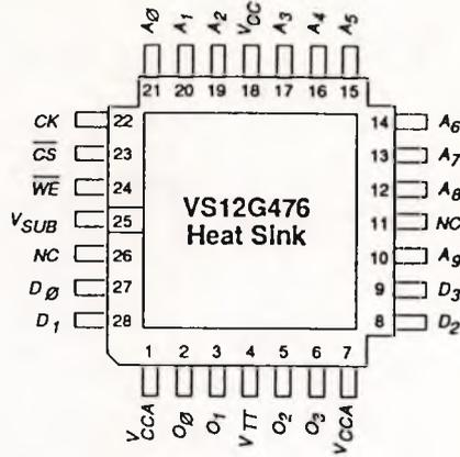
Connection Diagram (28-pin LDCC - Top View)
