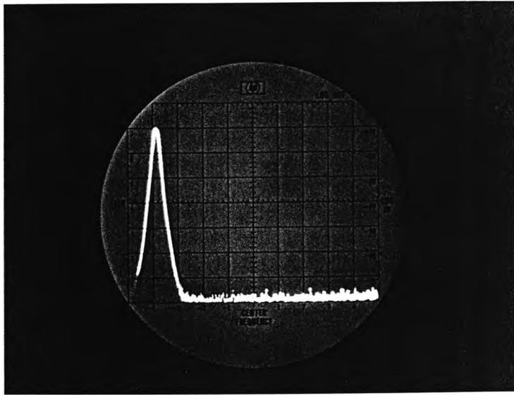
Fig. 7.4 Frequency spectrum of the output of the Ferrograph generator. The top and bottom grid lines at 0 dB and -70 dB respectively and the scale is 10 dB/div. The fundamental can be seen to be at -10 dB. Horizontal scale is 20 kHz/div.
