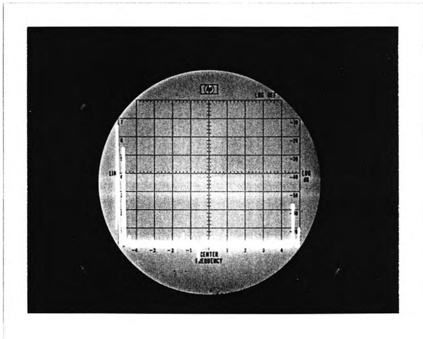
Fig. 7.7 Frequency spectrum of the output of the AC-FOL-DAC system over the frequency range of 0-100 MHz.
