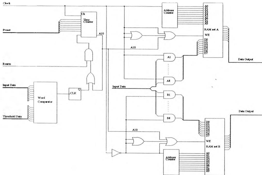
Fig 5.4 Block diagram for interleaved RAM system
