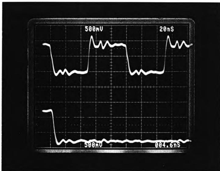
Fig. 7.16 The RAMCLK signal driving the clock input of the RAMs (upper trace) and the signal on the address line A6, during the 'write' mode, monitored on the oscilloscope (the Tek 7854). This shows that the A6 signal is stabilised half of a clock cycle before the rising edge of the clock.
