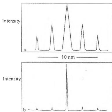
Figure 4.6 LD output spectrum, (a) multimode laser, (b) single mode laser.
