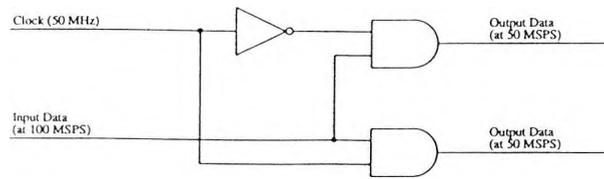
Fig 5.1 Demultiplexer circuit for interleaved RAM circuit
