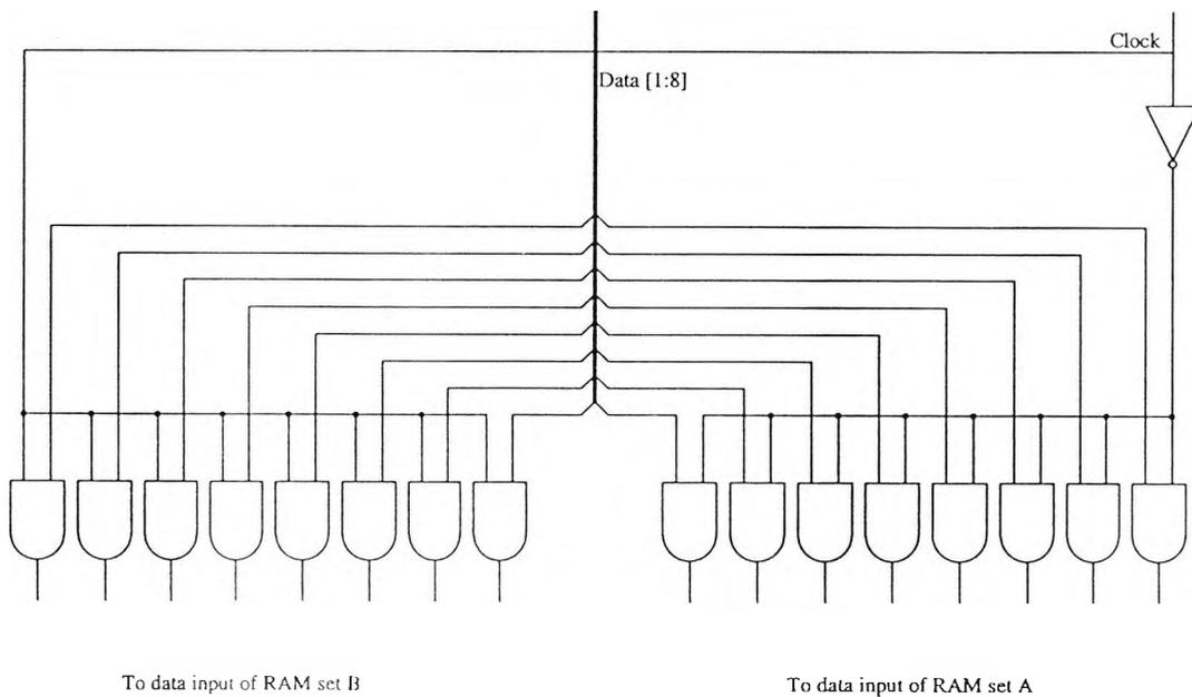
Fig 5.3 Demultiplexing gates circuit
