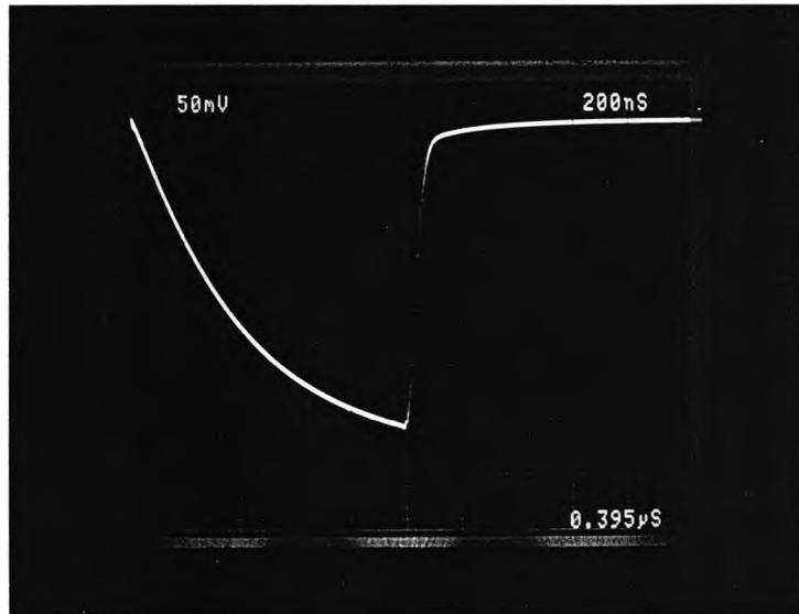
Fig. 7.8 Typical output of the chopped-impulse circuit with rise and chop times of about  $1\ \mu\text{s}$  and  $0.1\ \mu\text{s}$  respectively.
