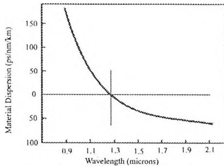
Figure 4.5 Material Dispersion as a function of wavelength for Silica Fibre
