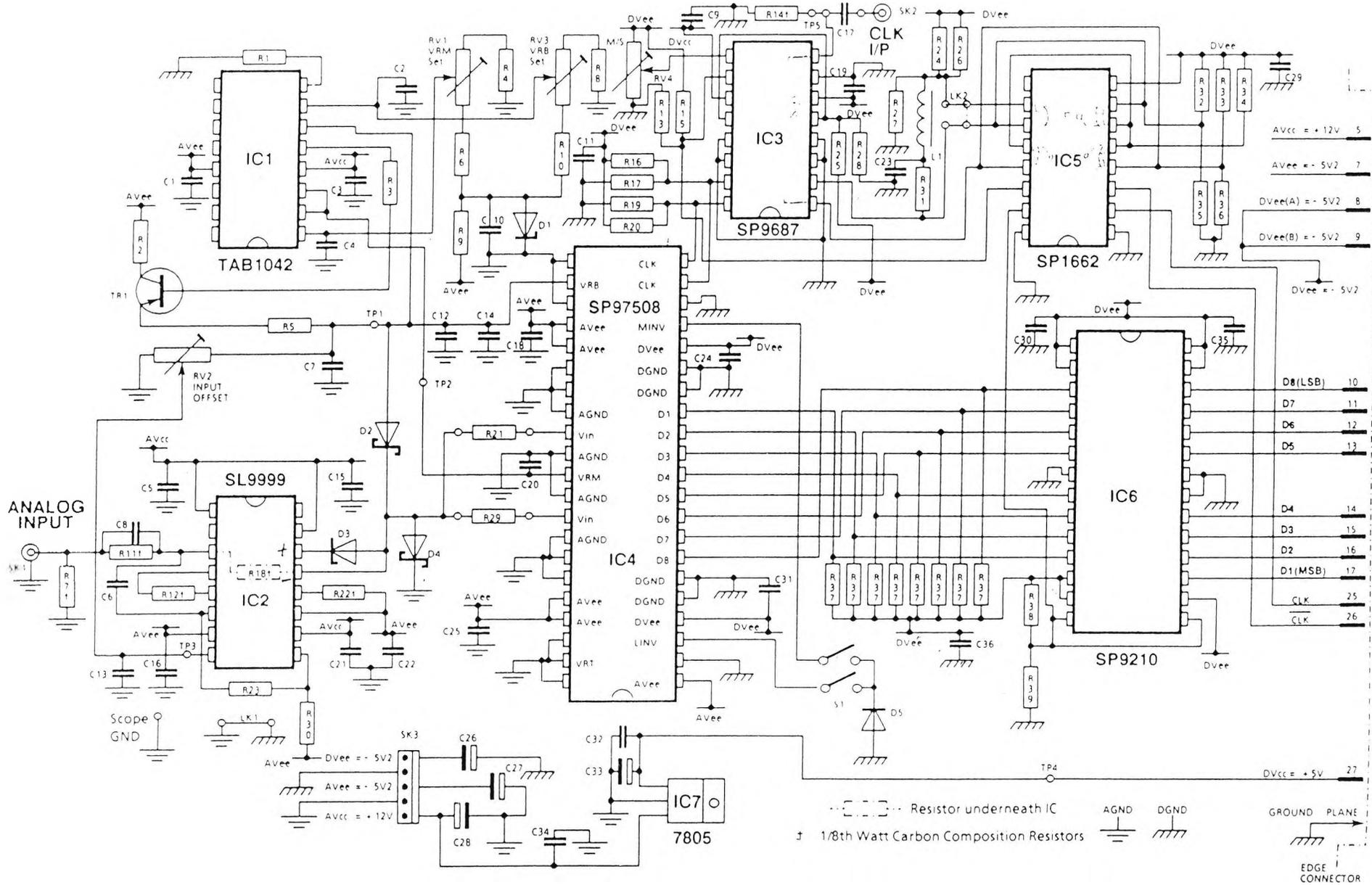
Fig D.1 SP97508 ADC Evaluation Board Circuit Diagram
