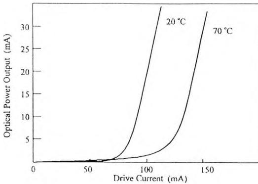
Figure 4.7 LD Output variation with temperature
