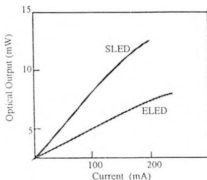
Figure 4.10 Emitted Power Profile of SLED and ELED
