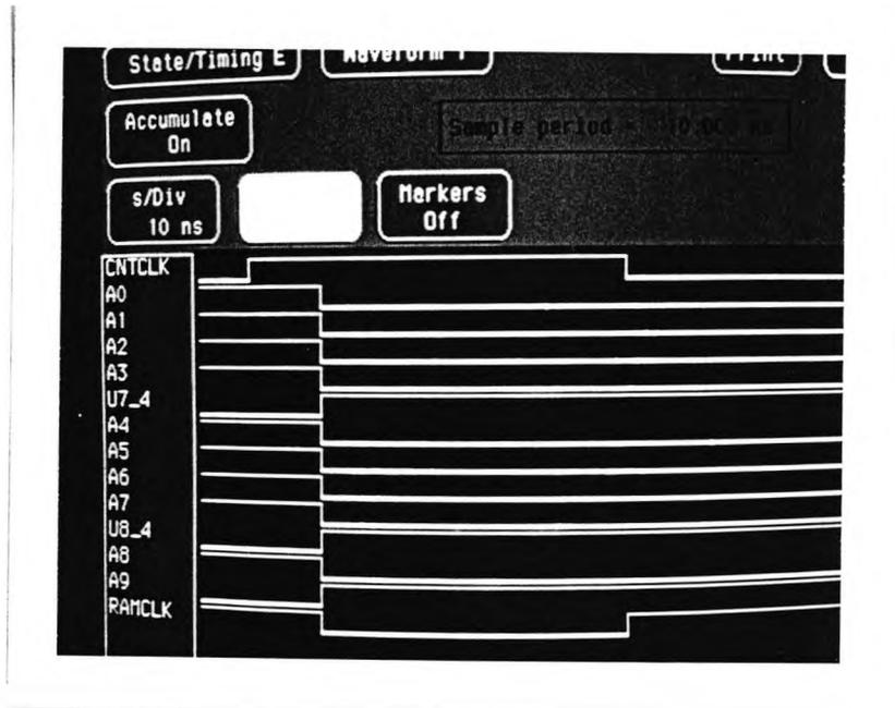
Fig. 7.14 Timing diagram of the address lines driving the RAMs while data was being recorded in the RAMs. In this instance the address lines A0-A9 are changing state from 01 1111 1111 to 10 0000 0000.
