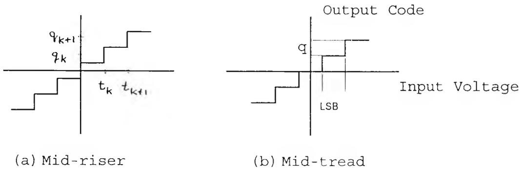
Figure 3.2 Mid-riser and Mid-tread characteristics
