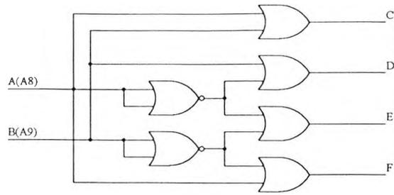
Fig 5.5 Address decoding circuit generating bit select outputs
