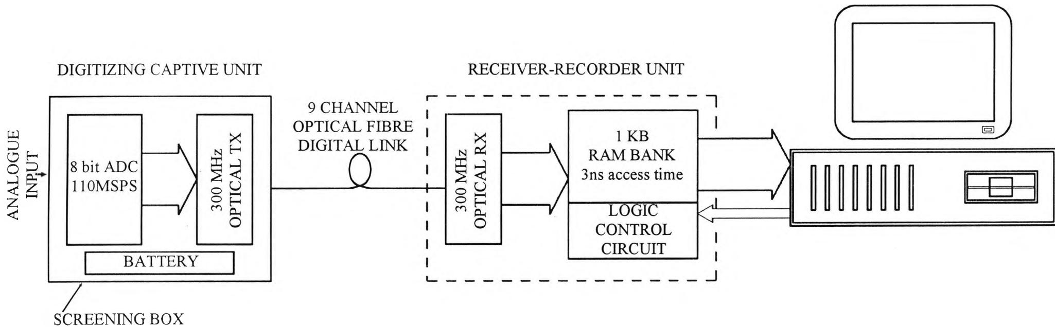
Fig 1.1 Block diagram of DOCTR
