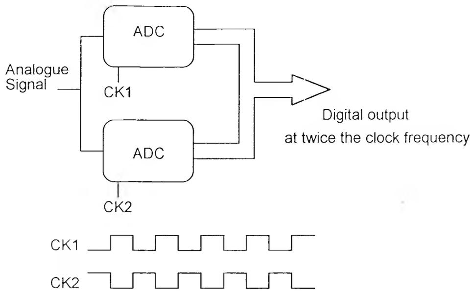
Figure 3.3 Interleaving techniques using two ADCs
