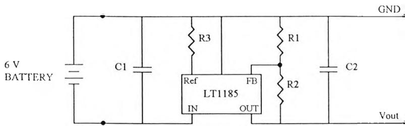
Fig H.1 Voltage regulator circuit diagram
