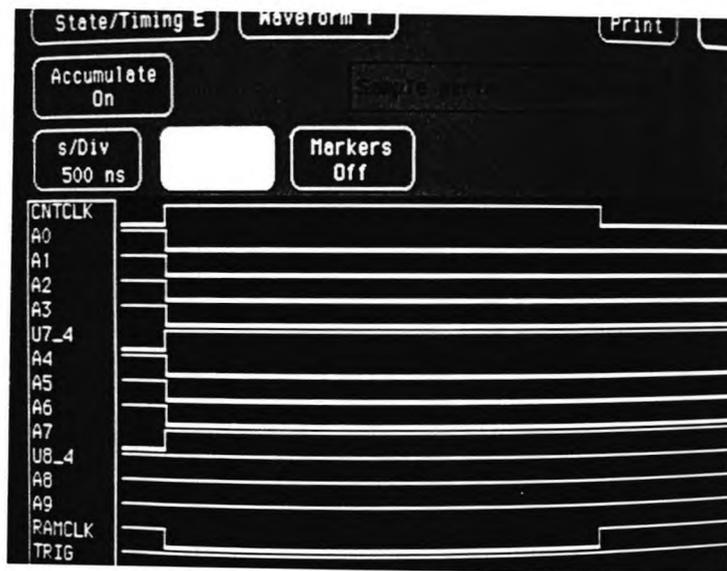
Fig. 7.18 The timing diagram of the RAM address inputs during the 'read' mode. The address lines A0-A9 changing from 11 0111 1111 to 11 1000 0000.
