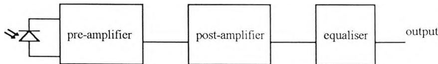
FIG. 4.30 Block Diagram of Optical Receiver
