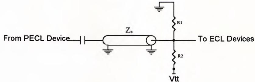
Figure A.1 Arrangement for matching PECL to ECL logic
