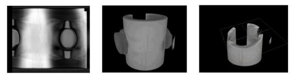
Figure 8. XCT scanning images of the specimen salted with sea salt
