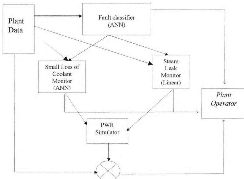
Figure 7.1 Block diagram of proposed Operators Advisory System
