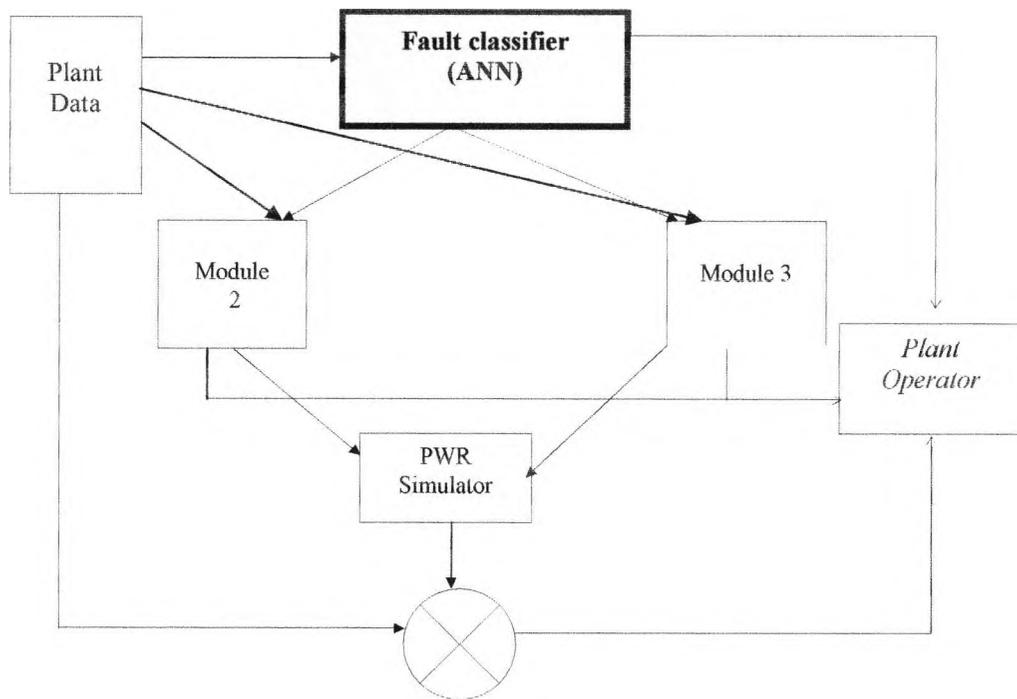
**Figure 4.2 Embedded Fault classifier in proposed OAS**
