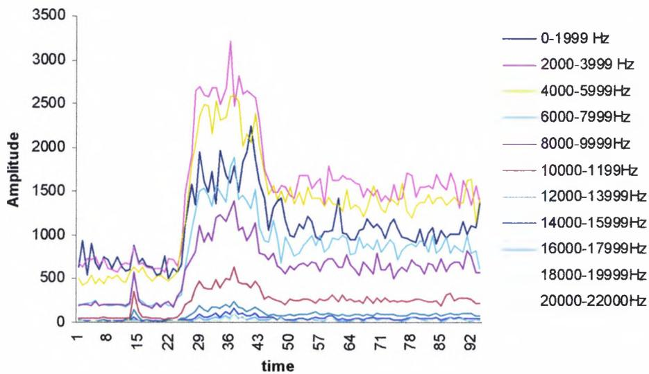
**Figure 6.14 Transition from first to second valve position**
