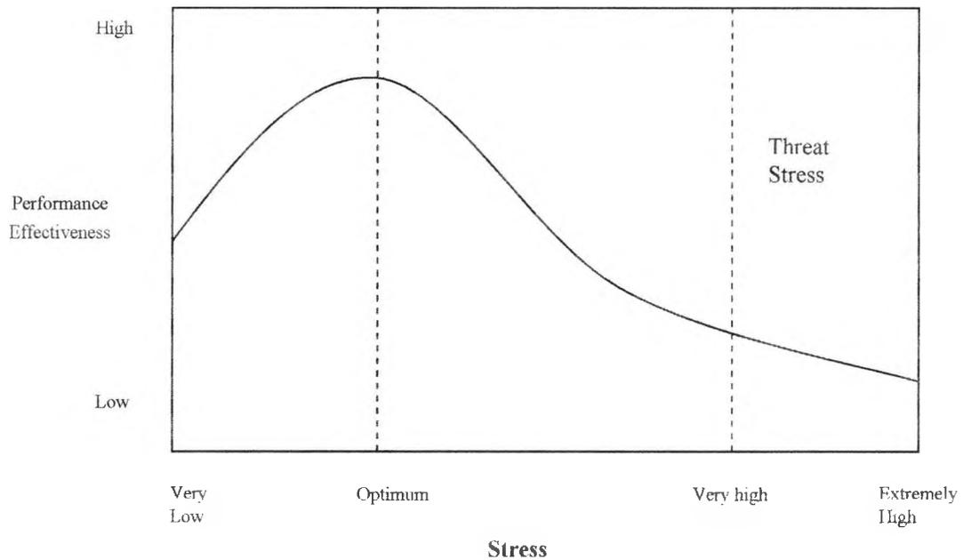
**Figure 3.2 the effect of stress on performance of plant operators**
