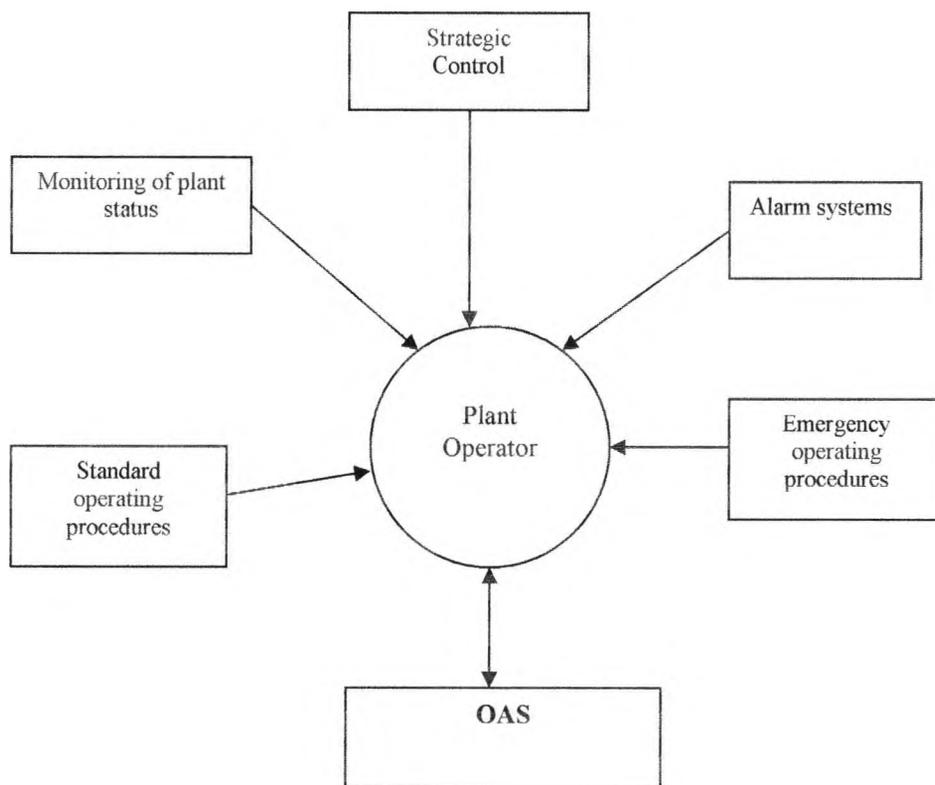
Figure 3.6 supervised control system with operator advisor
