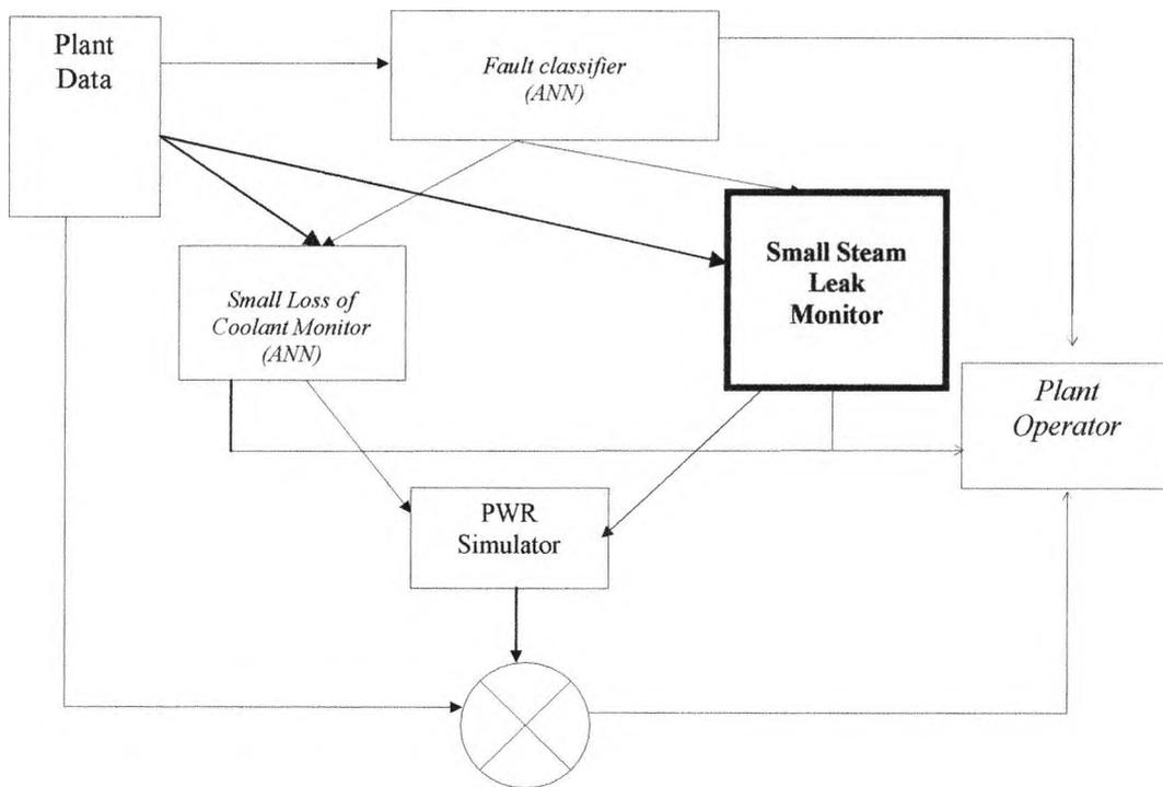
**Figure 6.1 Embedded Steam Leak Monitor in OAS**
