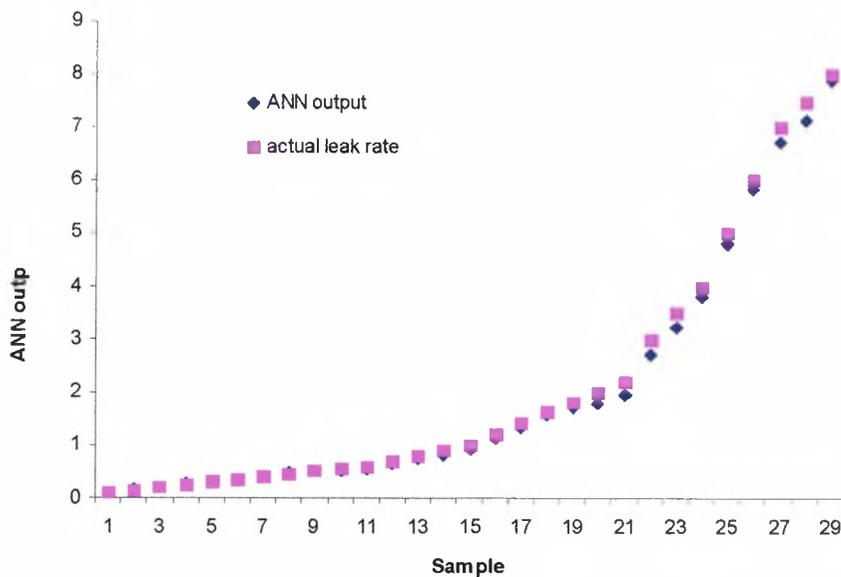
Figure 7.10 Estimated leak rate (LOCA)
