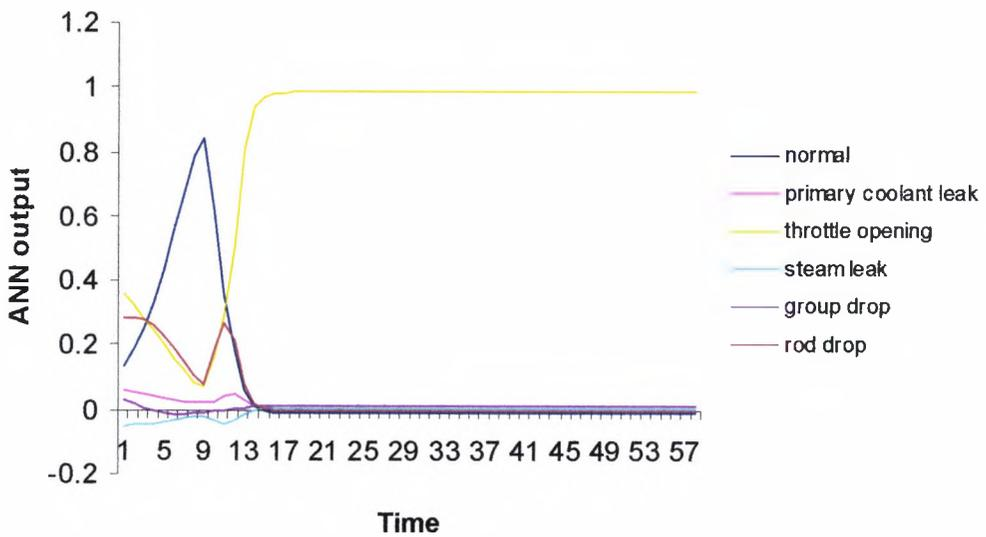
Figure 4.16 Throttle Opening Transient
