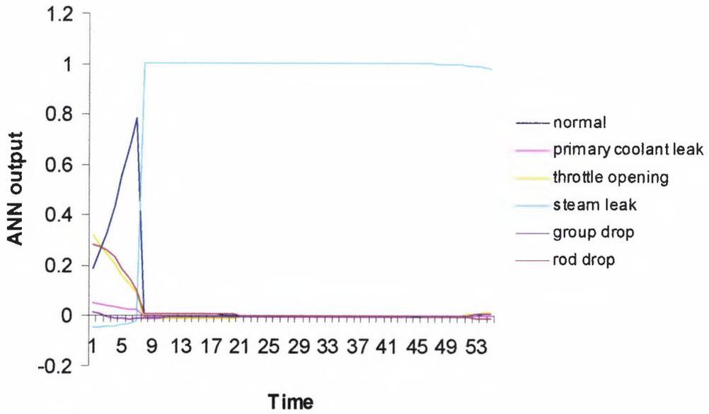
Figure 4.17 Steam Leak Transient
