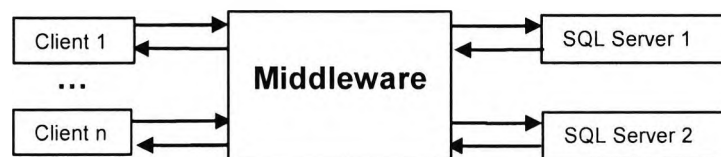
Fig. 3 - Fault-tolerant server node (FT-node) with two or more diverse SQL servers (in this case two: SQL Server 1 and SQL Server 2 ). The middleware “hides” the servers from the clients ( 1 to n ) for which the data storage appears as a single SQL server
