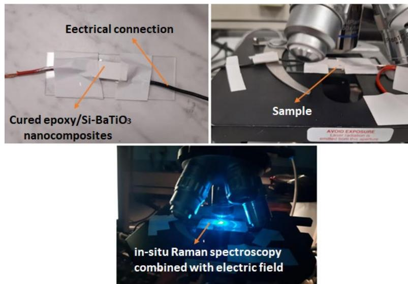
**Figure 5.** In-situ electric field equipped Raman spectroscopy of BaTiO<sub>3</sub>-epoxy nanocomposites.
