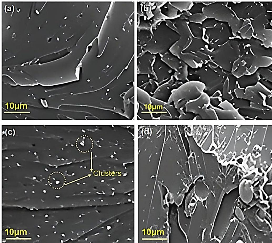
**Figure 6.** SEM images from the fracture surface of epoxy nanocomposites (taken from the former research in [9]): (a)-(c) images at 1 wt.%, 5 wt.% and 10wt% Si- BaTiO<sub>3</sub>, (d) untreated 10wt% BaTiO<sub>3</sub>.
