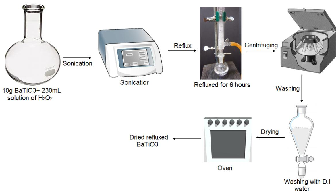
**Figure 1.** Schematic diagram of the Hydroxylation Process of BaTiO<sub>3</sub> nanoparticles (pre-treatment for adding of hydroxyl group (-OH) to the surface of BaTiO<sub>3</sub>).
