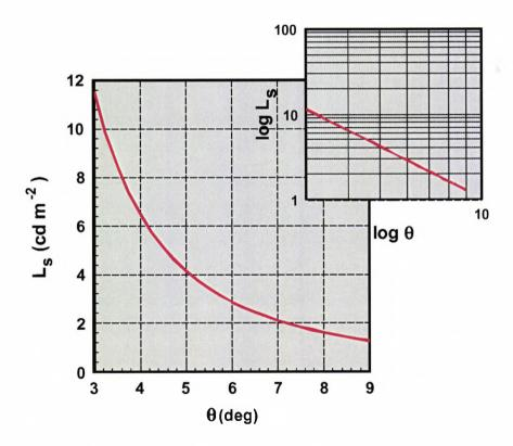
Figure 1-3: The theoretical straylight function showing how the luminance of scattered light varies with eccentricity
