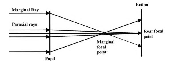
Figure 1-7: Longitudinal spherical aberration (positive) showing paraxial rays focusing on the retina and marginal rays focusing in front of the retina
