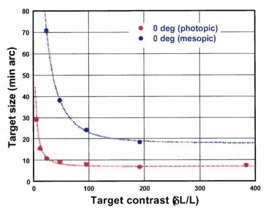
Figure 7-5: Foveal data showing the relationship between target size and target contrast, under both photopic and mesopic conditions.
