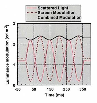
Figure 4-2: Nulling of the scattered light by modulation of the screen luminance
