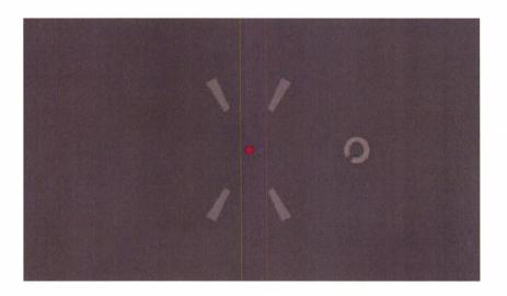
Figure 7-2: Stimulus configuration employed by the CAA test. The picture shows the stimulus at +2.5° eccentricity together with the central fixation target and fixation guides
