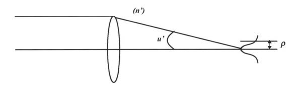
Figure 1-1: Calculation of the Airy disc diameter to the first dark ring
