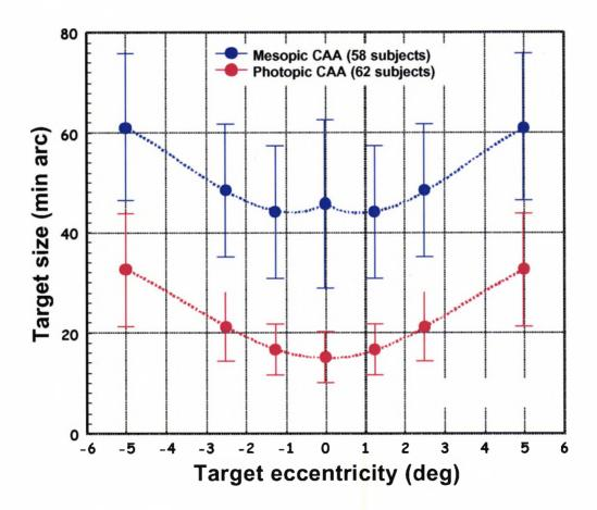
Figure 7-7: Target size thresholds for gap acuity with eccentricity measured under photopic (24% contrast) and mesopic (48% contrast) conditions.
