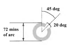
Figure 3-2: Dimensions of Landolt ring target
