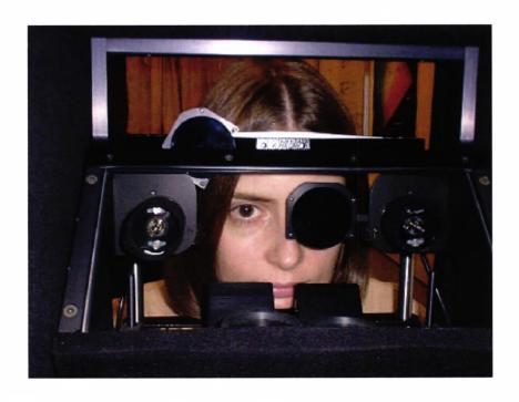
Figure 3-1: Experimental set-up employed throughout the study, showing the subject viewing the monitor through the P\_SCAN 100 system with the left eye occluded
