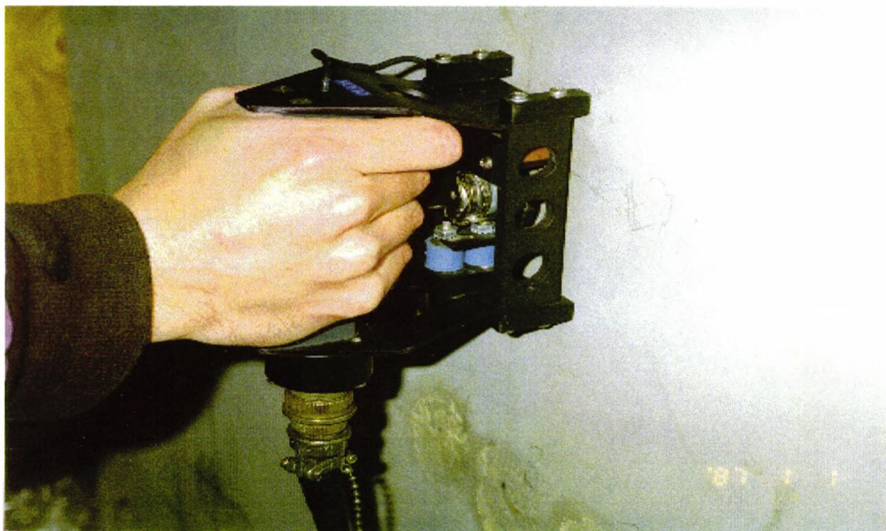
Figure 3.2: Impact echo testing on a specimen wall
