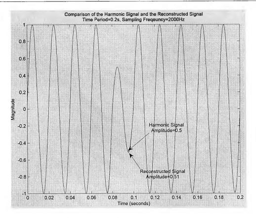
Fig. 9.3 Synthesized waveform vs. reconstructed waveform (sag)
