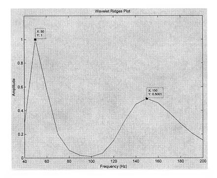
Fig. 6.15 Wavelet ridges plot for 50Hz and 150Hz ( $f_s = 450$ Hz, T = 0.2s) The instantaneous phases estimated at 50Hz and 150Hz are shown in Fig. 6.16(a) and Fig. 6.16(b) respectively. The estimated phases obtained from the wavelet coefficients lie between  $\pm \pi$ . It can be seen in Fig. 6.16 that there are abrupt phase variations near the start and the end of the phase plots. This is due to the edge effect mentioned earlier and to be discussed in Section 7.9.
