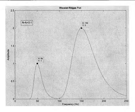
Fig. 7.5 Wavelet ridges plot for 50Hz and 150Hz
