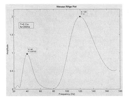
Fig. 6.13 Wavelet ridges plot for 40Hz and 120Hz ( $f_s = 350$ Hz, T = 0.11s)
