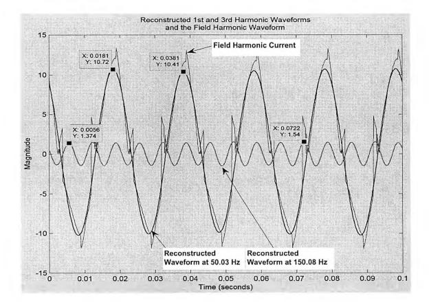
Fig. 9.13 Field harmonic signal vs. reconstructed fundamental & 3<sup>rd</sup> harmonic waveform
