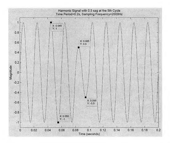
Fig. 9.2 Waveform of synthesized signal with one cycle of sag
