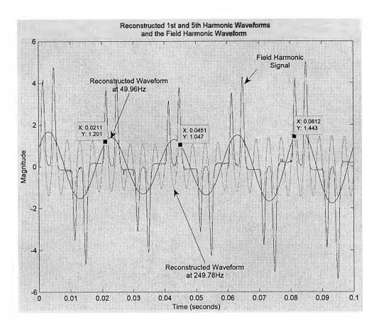
Fig. 9.12 Field harmonic signal vs. reconstructed fundamental & 5<sup>th</sup> harmonic waveform
