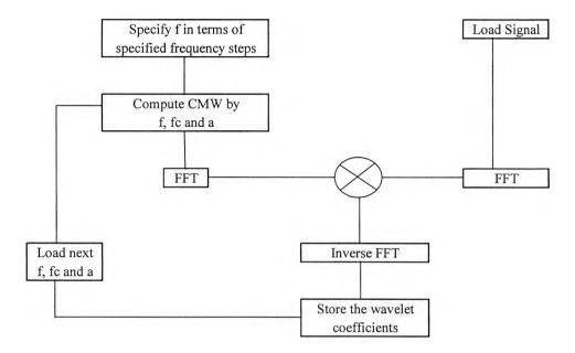
Fig. 7.1 Flow chart for the computation of wavelet coefficients by FFT
