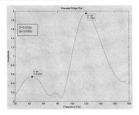
Fig. 6.14 Wavelet ridges plot for 40Hz and 120Hz ( $f_s = 350$ Hz, T = 0.036s)
