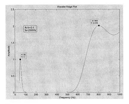
Fig. 6.8 Wavelet ridges plot for 50Hz and 800Hz ( $f_s = 2000Hz$ )
