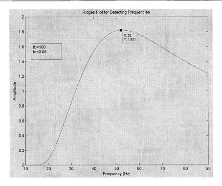
Fig. 6.7 Wavelet ridges plot for 40Hz and 60Hz ( $f_c \sqrt{f_b} = 0.5$ )
