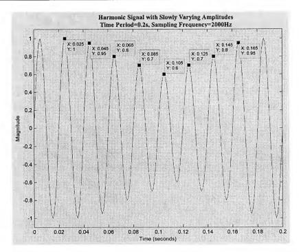
Fig. 9.4 Waveform of synthesized signal with slowly-varying amplitudes
