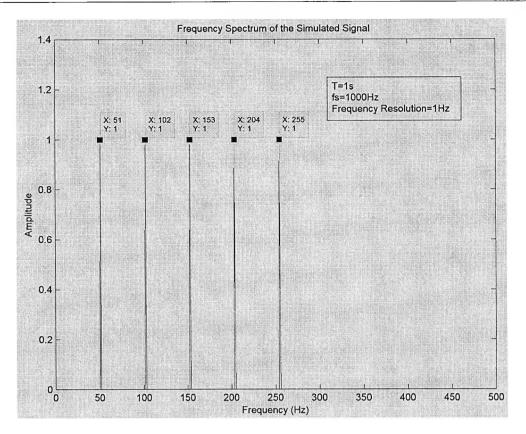
Fig. 4.3 Frequency spectrum by FFT with fine  $\Delta f$
