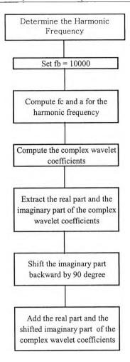
Fig. 9.1 Flow chart of the WT-based dynamic waveform reconstruction algorithm
