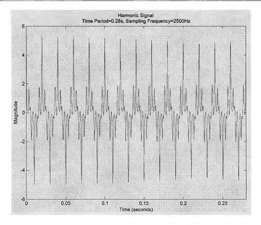
Fig. 8.10 Waveform of synthesized harmonics signal
