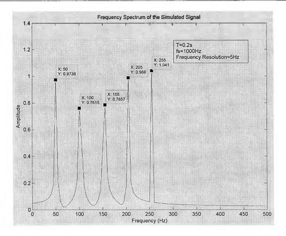
Fig. 4.2 Frequency spectrum by FFT with coarse  $\Delta f$
