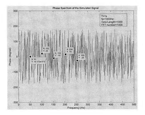
Fig. 4.9 Phase spectrum by FFT (fft no. = N & using Hamming window)
