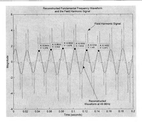
Fig. 9.11 Field harmonic signal vs. reconstructed waveform
