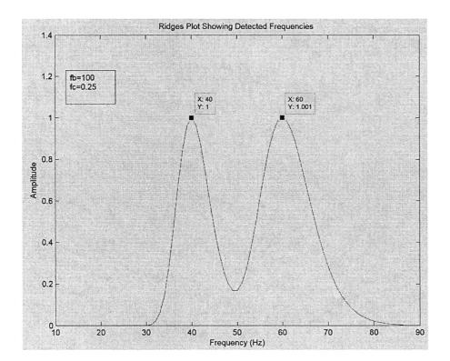
Fig. 6.4 Wavelet ridges plot for 40Hz and 60Hz ( $f_c\sqrt{f_b} = 2.415$ )
