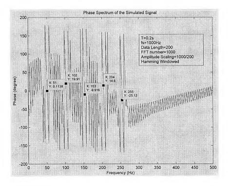
Fig. 4.8 Phase spectrum by FFT (fft no. > N & using Hamming window)
