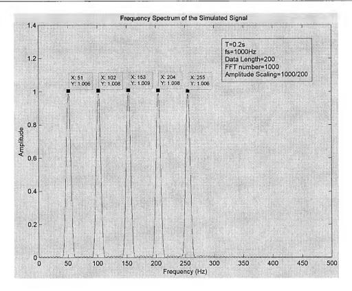
Fig. 4.6 Frequency spectrum by FFT (fft no. > N & using Hamming window)
