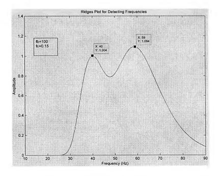
Fig. 6.6 Wavelet ridges plot for 40Hz and 60Hz (fc $\sqrt{f_b}$  = 1.5)
