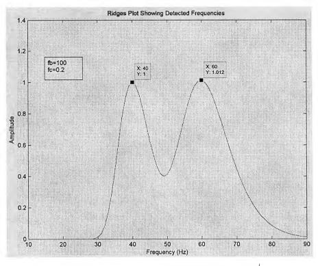
Fig. 6.5 Wavelet ridges plot for 40Hz and 60Hz (f\_c $\sqrt{f_b}$  = 2)
