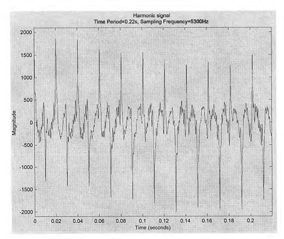
Fig. 8.7 Waveform of synthesized inter-harmonics signal
