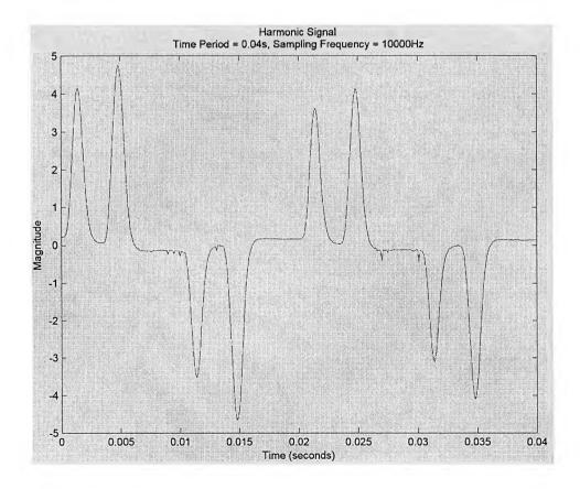
Fig. 8.12 Waveform of two cycles of VSD input current
