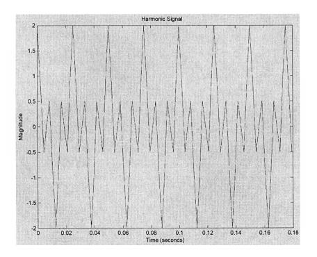
Fig. 6.11 Simulated signal (harmonics at 40Hz & 120Hz)
