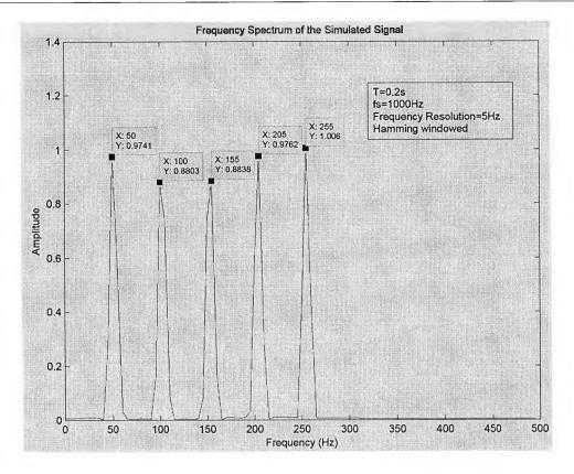
Fig. 4.4 Frequency spectrum by FFT (using Hamming window)
