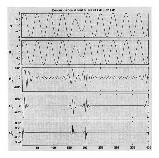
Fig. 9.8 Reconstructed waveform at the approximation (sag at the 5<sup>th</sup> cycle)
