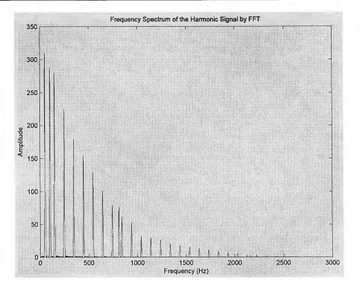
Fig. 8.9 Frequency spectrum by FFT of synthesized inter-harmonics signal
