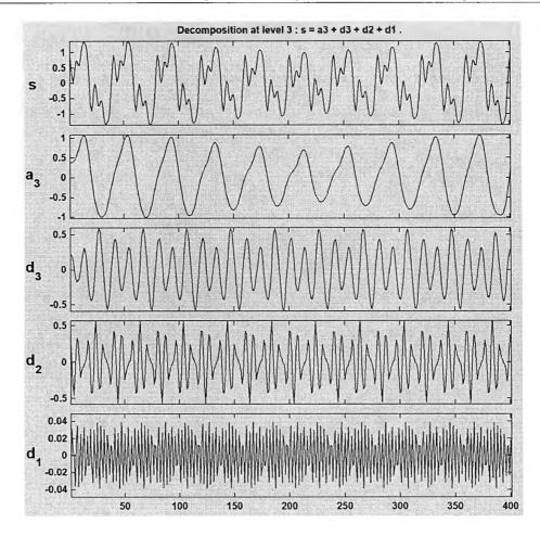
Fig. 9.10 Reconstructed fundamental waveform at the approximation (slowly-varying amplitudes)
