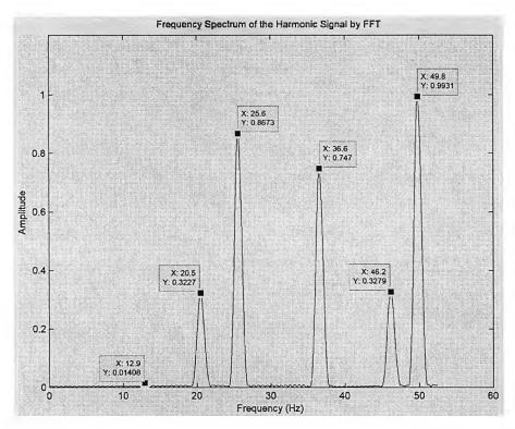
Fig. 8.5 Frequency spectrum by FFT of synthesized sub-harmonics signal
