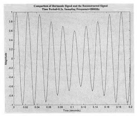
Fig. 9.5 Synthesized waveform vs. reconstructed waveform (slowly-varying amplitudes)
