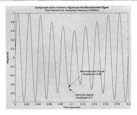
Fig. 9.7 Synthesized waveform vs. reconstructed fundamental waveform (slowly-varying amplitudes)
