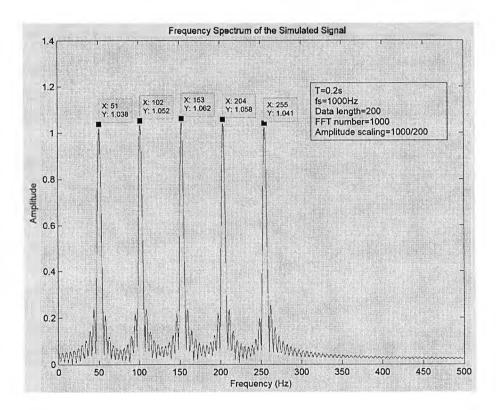
Fig. 4.5 Frequency spectrum by FFT (fft no. > N)
