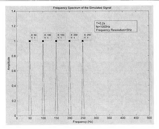
Fig. 4.1 Frequency spectrum by FFT
