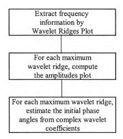
Fig. 7.4 Flow chart for estimating frequency, amplitude and initial phase
