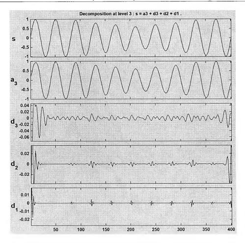
Fig. 9.9 Reconstructed waveform at the approximation (slowly-varying amplitudes)
