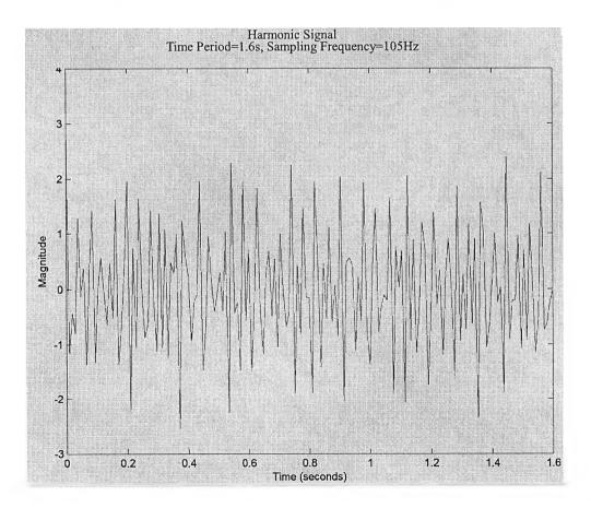
Fig. 8.1 Waveform of synthesized sub-harmonics signal
