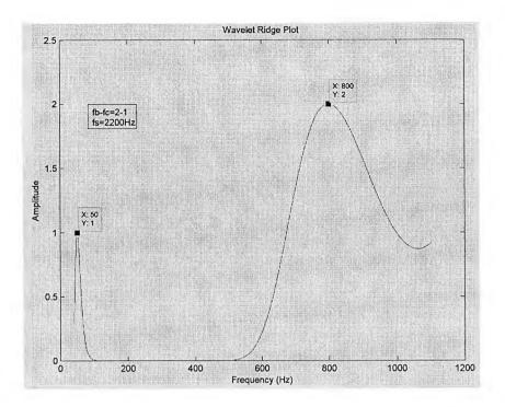
Fig. 6.9 Wavelet ridges plot for 50Hz and 800Hz ( $f_s = 2200Hz$ )
