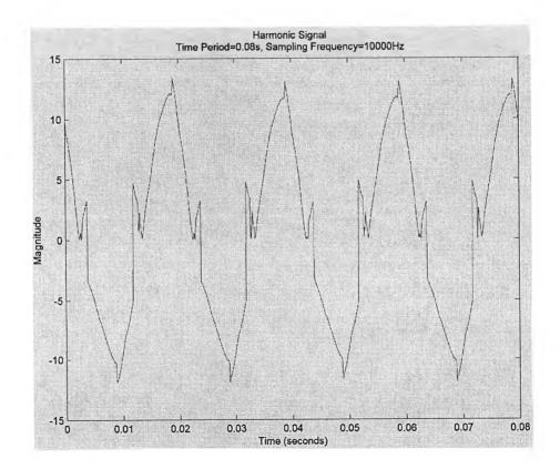
Fig. 8.14 Waveform of four cycles of single-phase input current
