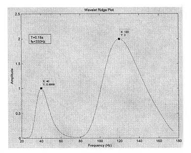
Fig. 6.12 Wavelet ridges plot for 40Hz and 120Hz ( $f_s = 350$ Hz, T = 0.18s)
