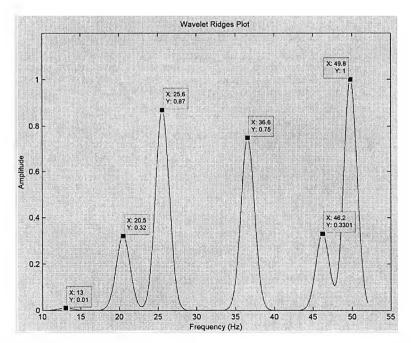
Fig. 8.2 Wavelet ridges plot of synthesized sub-harmonics signal
