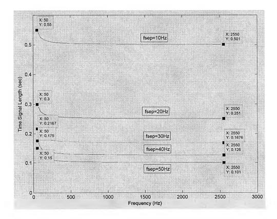
Fig. 7.2 Relationship between signal length and frequency separation
