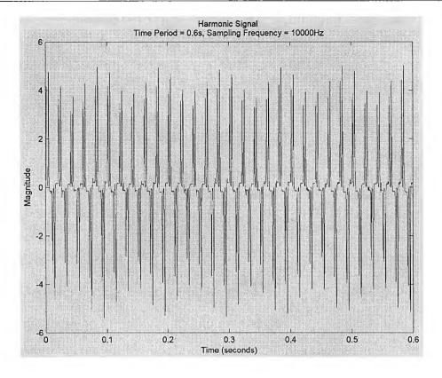
Fig. 8.11 Waveform of VSD input current (T = 0.6s)
