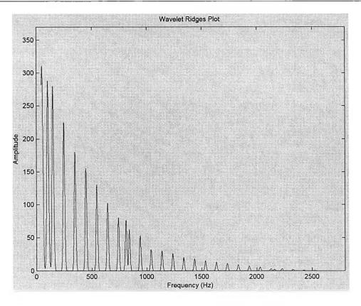
Fig. 8.8 Wavelet ridges plot of synthesized inter-harmonics signal
