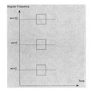
Fig. 5.4 Heisenberg boxes of the CMW for different centre frequencies
