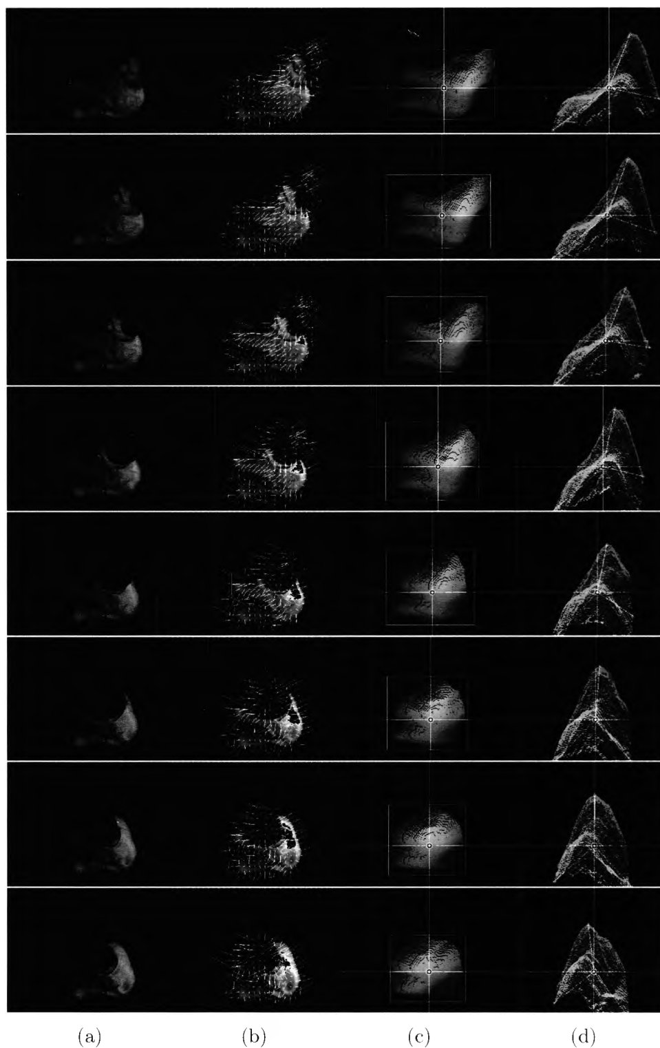
Figure 4.11: An example sequence of the 3D surface reconstructed from an adult class: (a) the original input sequence, (b) the needle maps, (c) and (d) the sequence of the reconstructed surface viewed from the top and rotated 90 degree, respectively.
