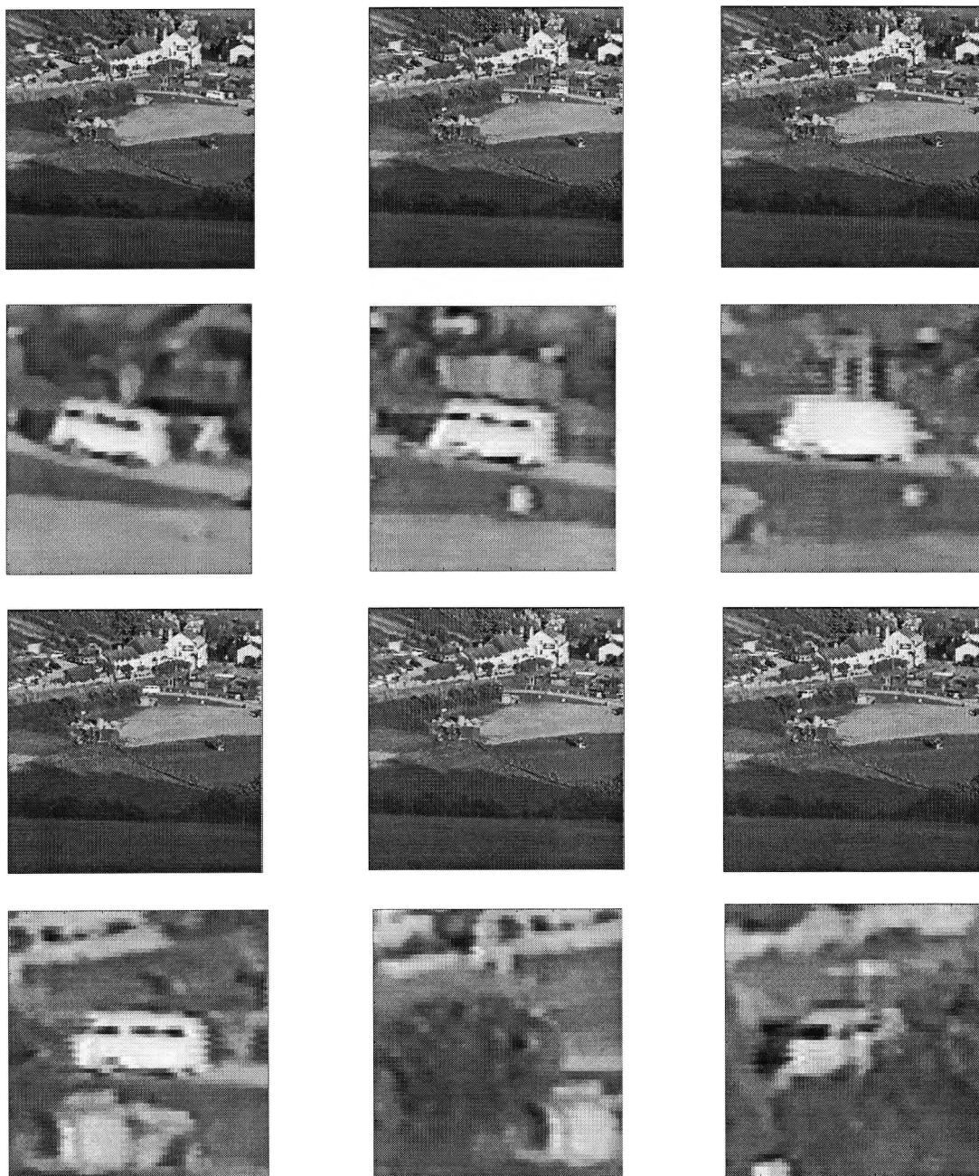
Figure 5.7 A six frame clip from an image sequence of over 90 frames. The top three images show the vehicle moving in a well defined manner left to right and up a slight gradient. The next three images show enlarged areas of the original image where the vehicle is moving. The following three images show the vehicle turning left and then becoming fully and then partially occluded behind a hedge. The last three images show the corresponding enlarged portions of the original image depicting this motion.
