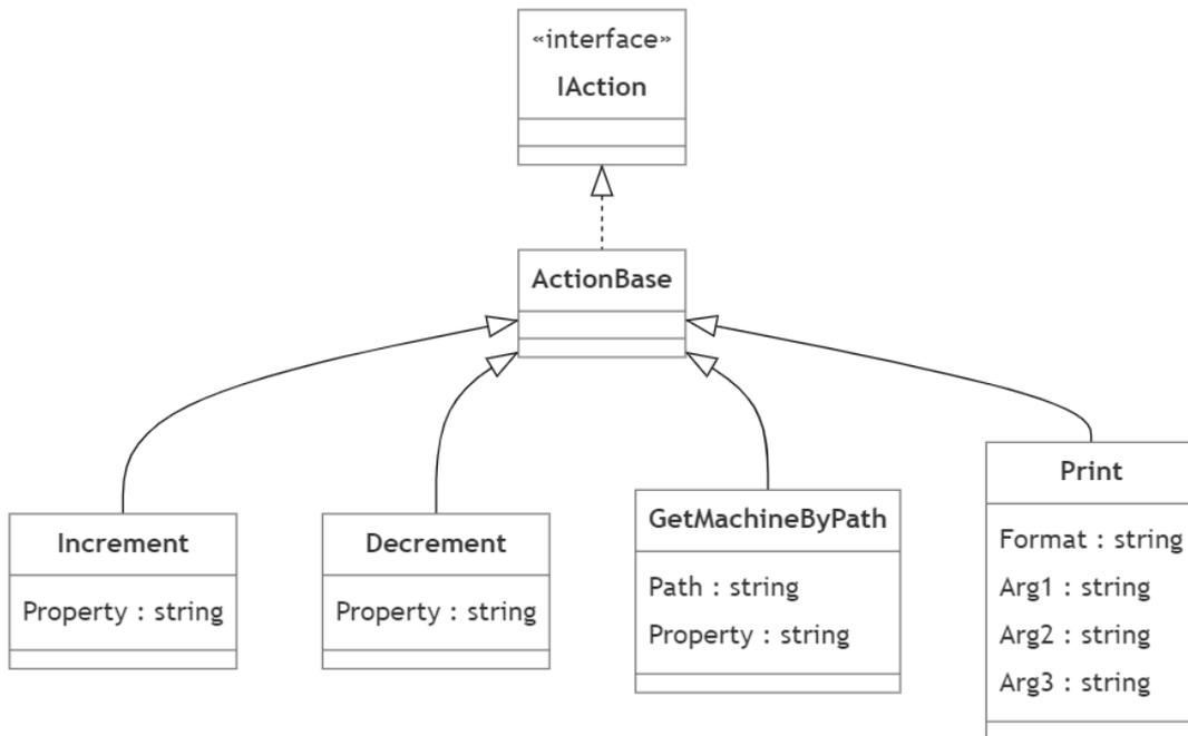
Fig. 4.8. Implementations of *IAction* in the definitions package.
