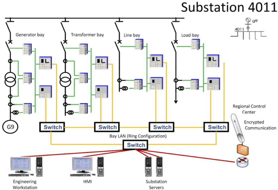
Figure A.3: Structure of the substation 4011.
