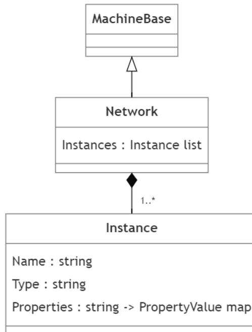
Fig. 4.3. Network and Instance classes from the definitions package.
