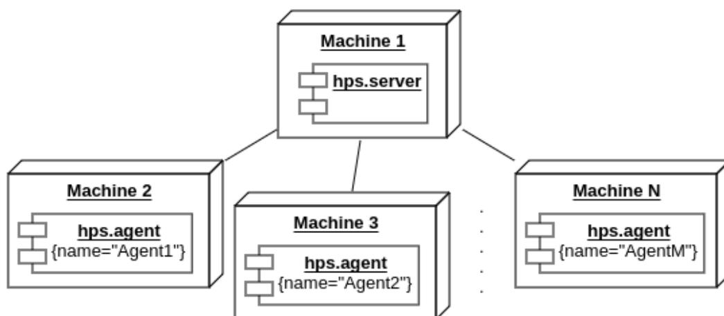
Figure 4.13: Deployment diagram of HPS server and agents.
