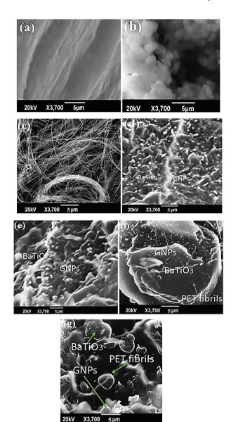
Figure 18. SEM images, a) Polypropylene (PP); b) Polypropylene (PP)/polyethylene terephthalate (PET) blend after surface extraction of polypropylene (PP) by hot xylene (B); c) polypropylene (PP)/polyethylene terephthalate (PET) in situ fibrils composites after surface extraction of polypropylene by hot xylene (FC), d) GBNC1 cryo- fractured surfaces, e) GBNC3 cryo-fractured surfaces, f) GBFNC1 cryo- fractured surfaces, g) GBNFC3 cryo-fractured surfaces.
