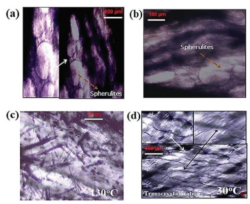
**Figure 7.** Polarized optical microscopy (POM) microstructure of a) PP/PET Blend (B) at 30 °C as in form of spherulites (Spherical ring), b) PP/PET-GNP-BaTiO<sub>3</sub> nanocomposites (GBNC1) at 30 °C as in form of spherulites (Spherical ring), c) PP/PET-GNP-BaTiO<sub>3</sub> fibrils nanocomposites (GBFNC1) at 130 °C as in form of transcrystalline growth, d) GBFNC1 at 30 °C as in form of transcrystalline growth.
