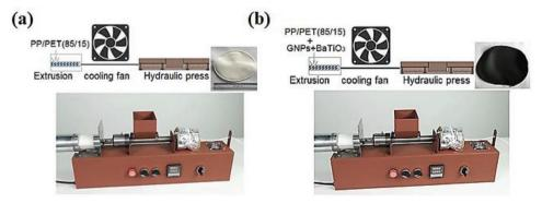
Figure 2. a) The exploratory setup for blends (B), b) Experimental setup for GNPs and BaTiO<sub>3</sub> based nanocomposites (GBNC).
