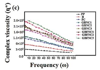
**Figure 14.** a) Variation of storage modulus with frequency(hertz (Hz)), b) Variation of loss modulus with frequency(hertz (Hz)), c) Variation of complex viscosity with frequency(hertz (Hz)).
