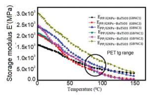
**Figure 12.** Analysis of storage modulus of GNPs+BaTiO<sub>3</sub> nanocomposites and in situ GNPs+BaTiO<sub>3</sub> polyethylene terephthalate (PET) fibrils nanocomposites with varying the phr of GNPs+BaTiO<sub>3</sub> through two population approach.
