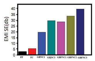
**Figure 19.** Electromagnetic shielding effectiveness of polypropylene (PP), FC, GBNC1, GBFNC3, GBFNC1, GBFNC3.
