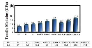
Figure 15. Comparatives study of the a) Tensile strength, b) Tensile modulus of prepared samples.
