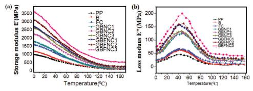
Figure 11. Variation of a) storage modulus, b) Loss modulus of GNPs+BaTiO<sub>3</sub> nanocomposites and in situ GNPs+BaTiO<sub>3</sub> polyethylene terephthalate (PET) fibrils nanocomposites with varying the phr of GNPs+BaTiO<sub>3</sub>.
