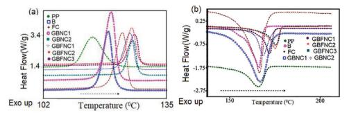
Figure 8. a) Crystallization, b) melting behavior of polypropylene (PP) in B, FC, GBNC1, GBNC2, GBFNC1, GBFNC2, and GBFNC3 (Exo up tends to exothermic process).
