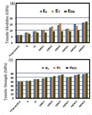
**Figure 16.** A Comparatives study of the experimental and theoretical for a) tensile moduli and b) strength.
