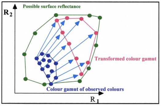
Figure 5.8 The changes of observed colours in the colour space when the Crule algorithm is applied.
