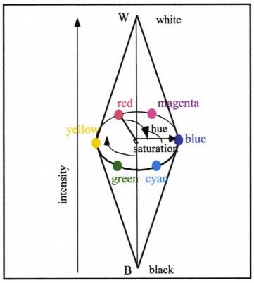
Figure 2.4 (I)Intensity, (S)Saturation, (H)Hue colour Space.
