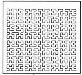
Figure 4.8  $H_s^2$  scan, 2-dimensional Peano Scan with the resolution 32.
