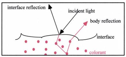
Figure 2.5 Reflected light from a dielectric material
