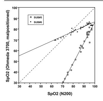
**Fig. 4** SpO<sub>2</sub> values for malpositioned Ohmeda 3700, earlobe versus control SpO<sub>2</sub> values; single-subject data showing two individuals and their separate linear regressions. Single-subject data fall much closer to regression lines than pooled data (Fig. 4), but the regressions for different individuals vary widely. Reproduced (with permission) from Barker et al. study [14]
