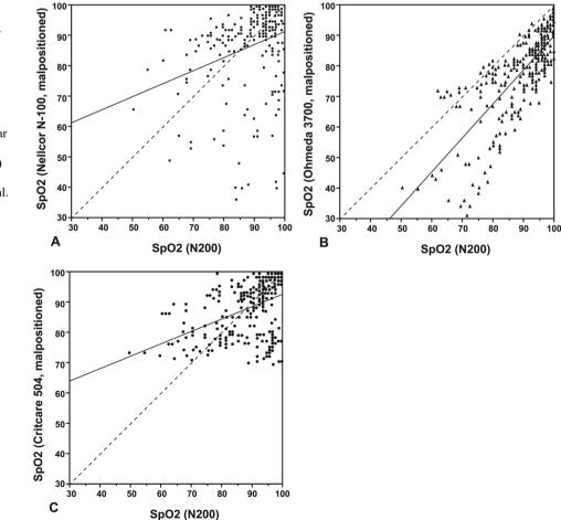
**Fig. 3** SpO<sub>2</sub> values from three pulse oximeters with malpositioned sensors versus simultaneous SpO<sub>2</sub> values of properly positioned control oximeter (Nellcor N-200, finger). Pooled data for 12 subjects are shown for. (**A**) Nellcor N-100, finger; (**B**) Ohmeda 3700, earlobe; and (**C**) Criticare 504, earlobe. Linear regression best-fit (solid-line) and line of identity (dashed line) are shown. Reproduced (with permission) from the Barker et al. study [14]
