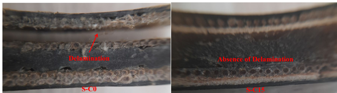
Fig. 7 Damage due to flexural loading
