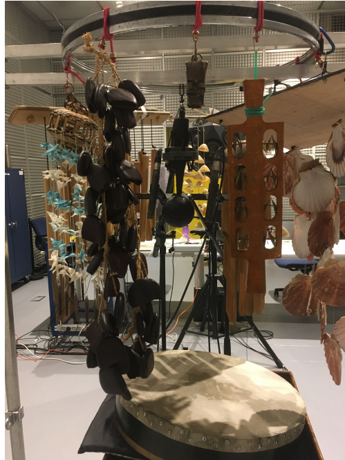
Figure 2. Percussion setup for Prestidigitation showing the Eigenmike in the center and the IKO in the background.
