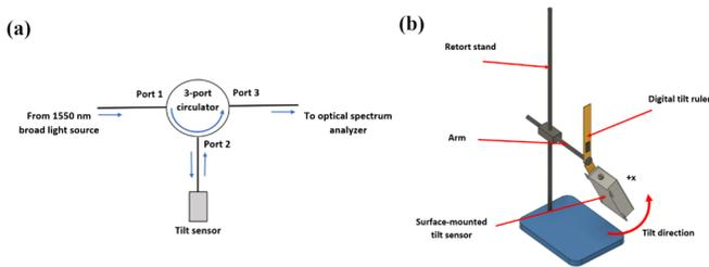
Fig. 4. (a) Schematic of the sensor's interrogation setup and (b) illustration of the tilt calibration procedure.
