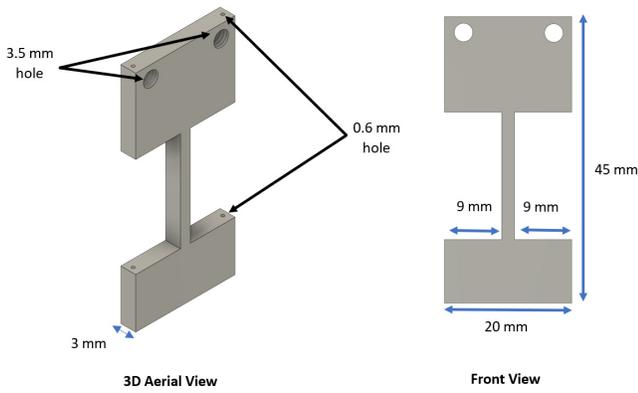
Fig. 1. Actuator design.
