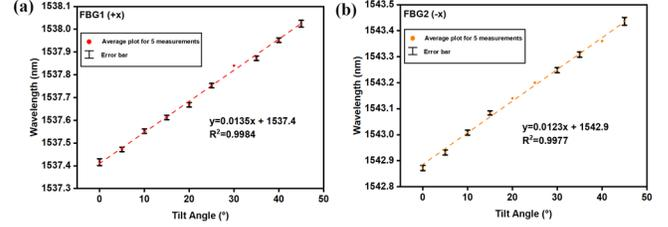
Fig. 9. Linear response with their respective error bars for (a) FBG1 and (b) FBG2 during the tilt calibration of the tilt sensor.
