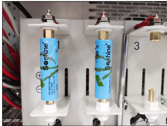
Figure 2. Photograph of the battery cycling set-up, with embedded FBG-based sensor system installed inside the BTS 4000 environmental chamber.
