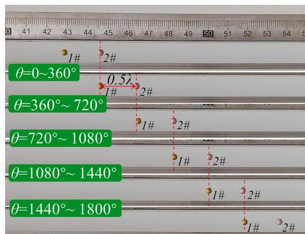
Fig. 10. Photograph of experiments showing simultaneous transportation of two polystyrene spheres by adjusting the value of  $\theta$  (where 3 mm diameter,  $f = 18.214$  kHz,  $V_{\text{peak-peak}} = 80$  V).
