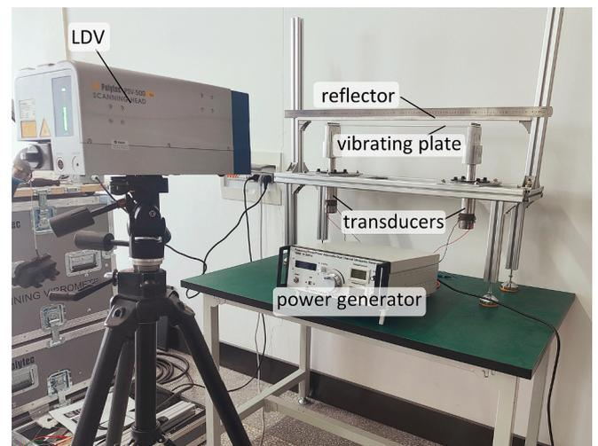
Fig. 5. Photograph of the experimental equipment used for measuring acoustic field and for transporting small balls.
