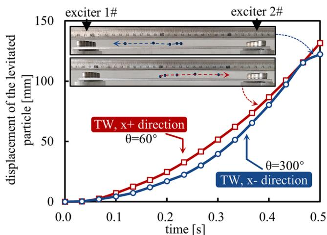
Fig. 7. Relationship between the transport position of the polystyrene spheres and time in the TW mode (where  $\theta = 60^\circ$  and  $300^\circ$ ,  $f = 18407$  Hz, and  $V_{\text{peak-peak}} = 120$  V). (This video is available as supplementary video 001 and video 002).
