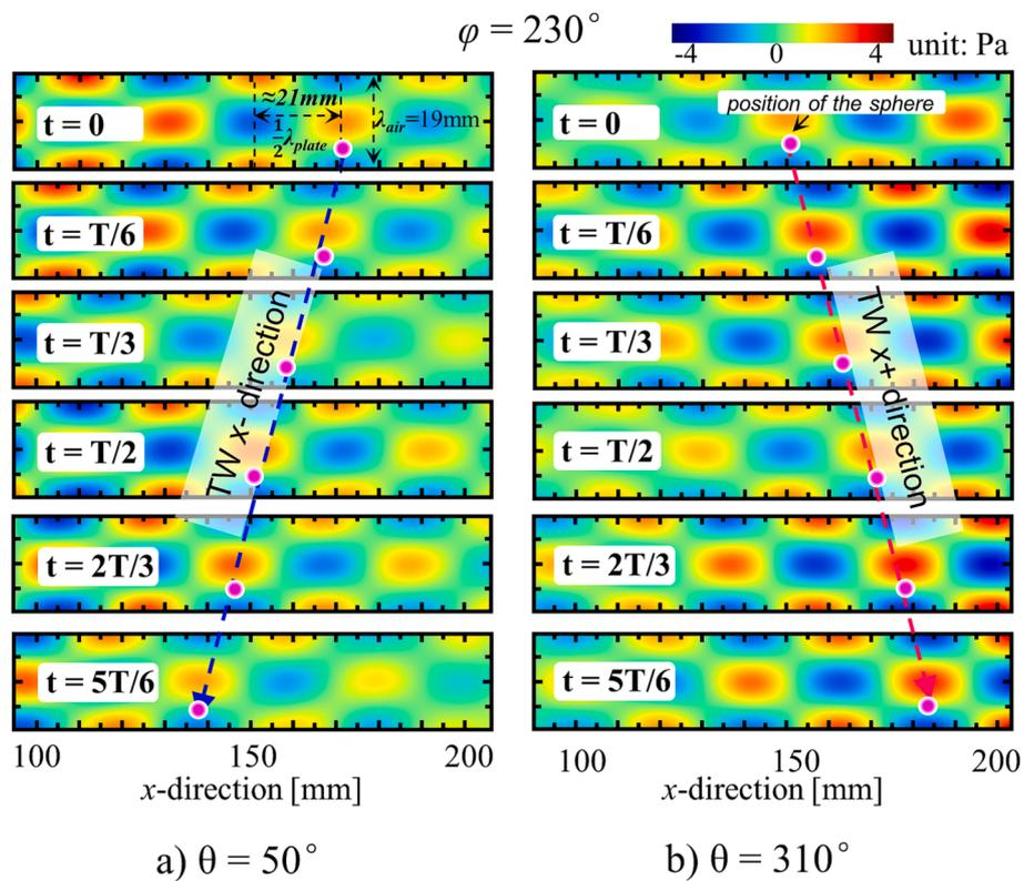
Fig. 3. FEA results of the TW acoustic field in the  $x +$  and  $x -$  direction under specific temporal phase shift  $\theta_1 = 50^\circ$  and  $\theta_2 = 310^\circ$ , respectively ( $f = 18.0$  kHz).
