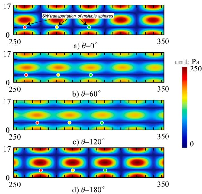
Fig. 4. FEA results of the SW acoustic field, where the nodes move to the  $x +$  direction ( $f = 18.0$  kHz, and  $\theta$  was changed from  $0^\circ$  to  $180^\circ$ , with an interval of  $60^\circ$  used).
