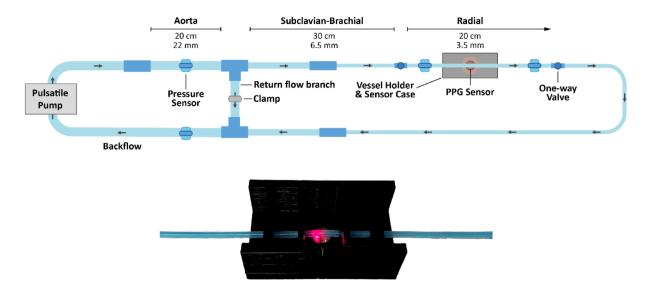
**Figure 1.** Schematic diagram of in-vitro setup (top) and photo of custom vessel held in PPG sensor case (bottom).
