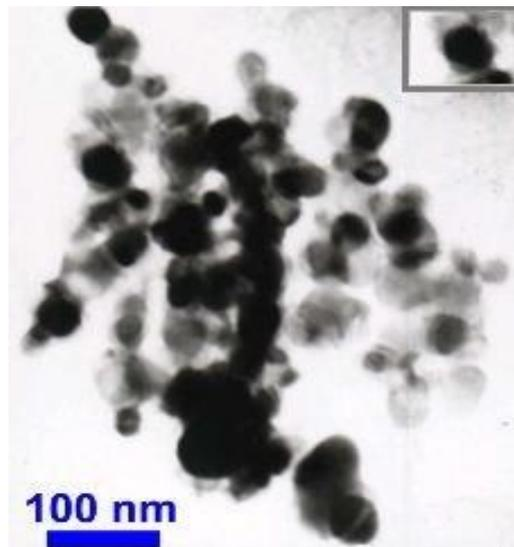
**Fig.3 TEM picture of CuO nanoparticles**
