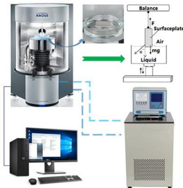
**Fig.2 Diagram of the solution surface tension test system**
