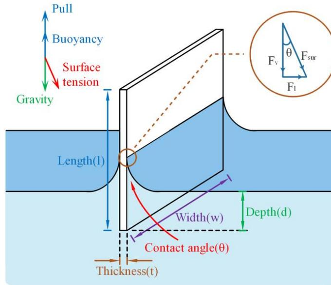
**Fig.1 Principle of the surface tension measurement**
