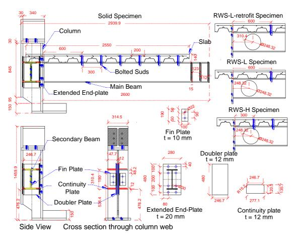
Figure 2. Dimensions of test specimens (mm)
