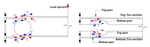
Figure 5.Illustration of the behaviour of Tee-sections.
