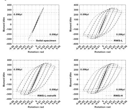
Figure 4. Hysteretic curve of the specimens.
