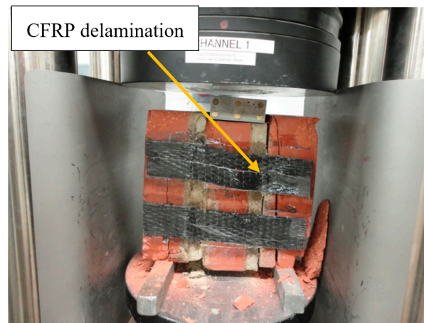
Figure 15. CFRP strips on two sides.
