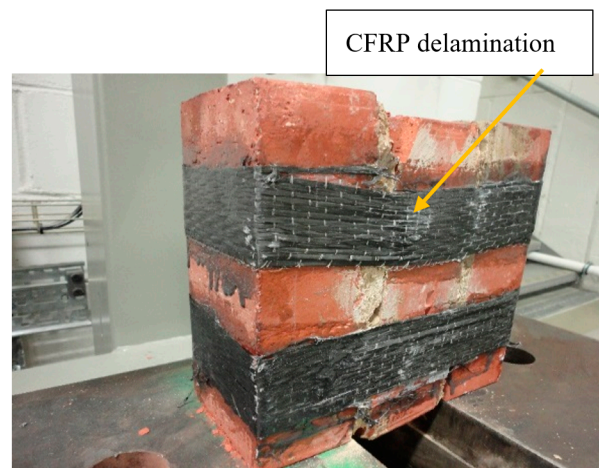
Figure 23. CFRP strips on four sides.
