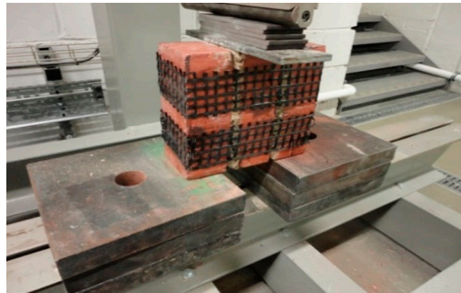
Figure 25. CFRP net strips on four sides.
