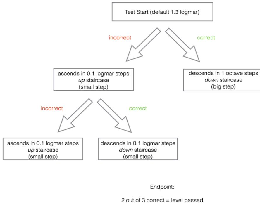
Figure 5.5: Flow chart explaining the staircase method followed in Peekaboo vision application
