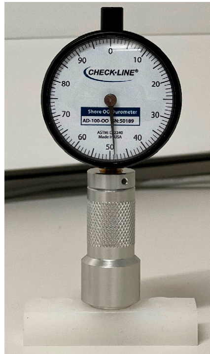
Figure 4. Measuring the hardness of silicone tissue using a Shore-OO Durometer.
