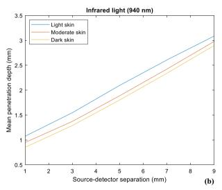
**Figure 9.** Mean photon penetration depth for light, moderate, and dark skin across a source-detector separation range of 1–9 mm at (a) 660 nm and (b) 940 nm.
