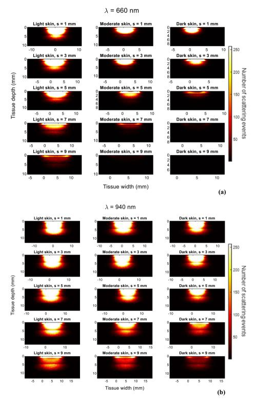
**Figure 7.** Photon propagation profiles of detected photons in reflectance PPG for light, moderate, and dark skin using a (a) 660 nm light source and (b) 940 nm light source across a source-detector separation range of 1–9 mm. Brighter regions illustrate the high density of scattering events.
