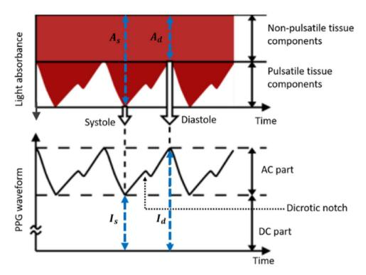
**Figure 3.** Schematic of the PPG waveform produced as a result of light absorbance during systole and diastole ( $A_s$  and  $A_d$ ). The corresponding light intensities are denoted by  $I_s$  and  $I_d$ , used for the calculation of the pulsatile AC component and non-pulsatile DC component from the Monte Carlo simulation.
