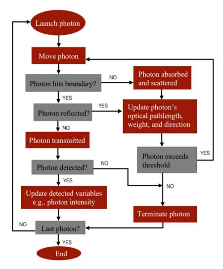
**Figure 1.** Monte Carlo algorithm adapted from <sup>12,29,30</sup>, which governs the movement of photons between the source and detector in both transmittance and reflectance PPG modes.
