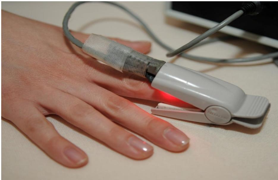
**Figure 6.13: Photograph showing the finger PPG sensor on a volunteers' index finger for evaluation.**
