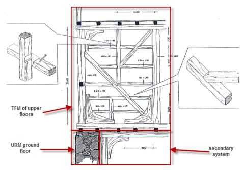
Figure 1. Connection of TFM super-structure with the URM ground floor and the secondary system (after [2]).
