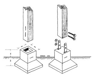
Figure 2. Stone foundations of timber posts of the secondary system of Lefkas' buildings (after [7]).
