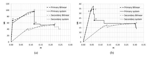
Figure 5. Pushover curves of the primary and secondary system of 'Berykiou' TFM building with: (a) full restraints and (b) flexible supports (SSI).
