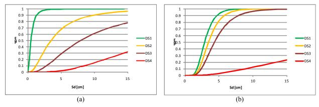
Figure 6. Fragility curves for 3storeys TFM buildings in Lefkas island on: (a) fully restrained and (b) flexible foundation (SSI).
