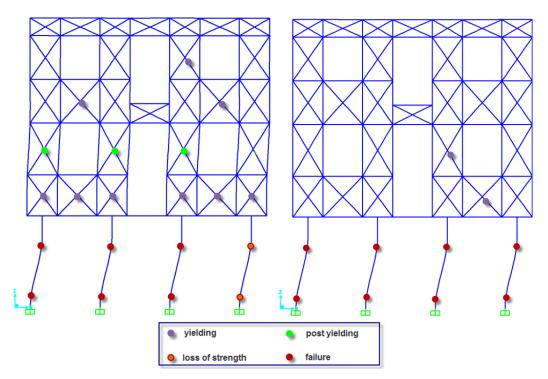
Figure 4. Failure mechanism of the primary (left) and the secondary (right) system of Berykiou TF building.
