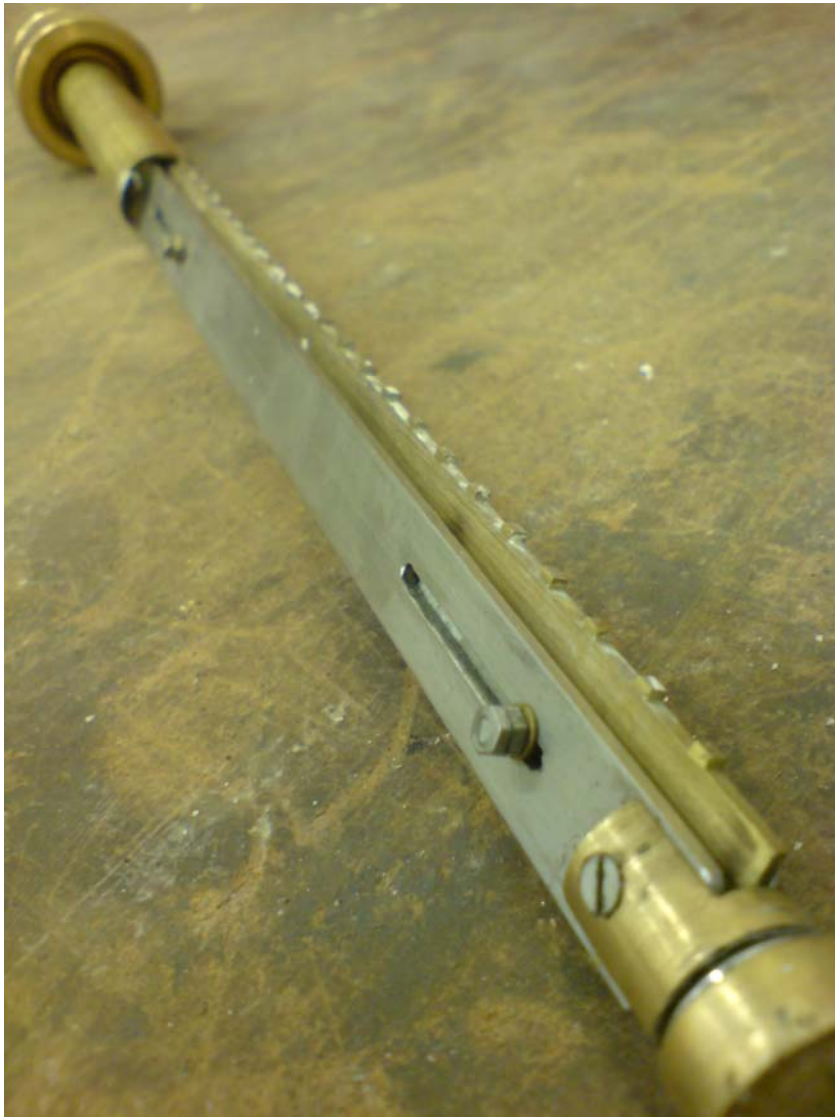
Figure 4.8 Photograph of complete rib-cutting tool
