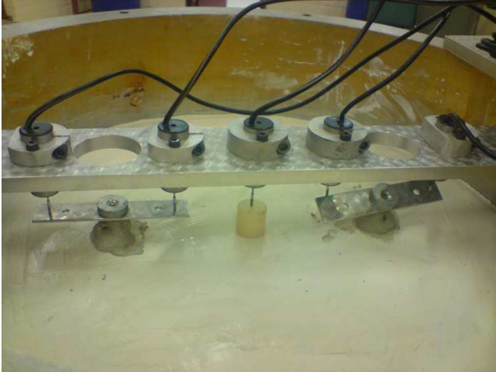
Figure 6.22 Photograph showing pile heads after test JW03
