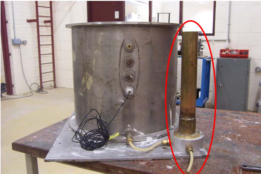
Figure 4.18 Photograph showing the variable standpipe
