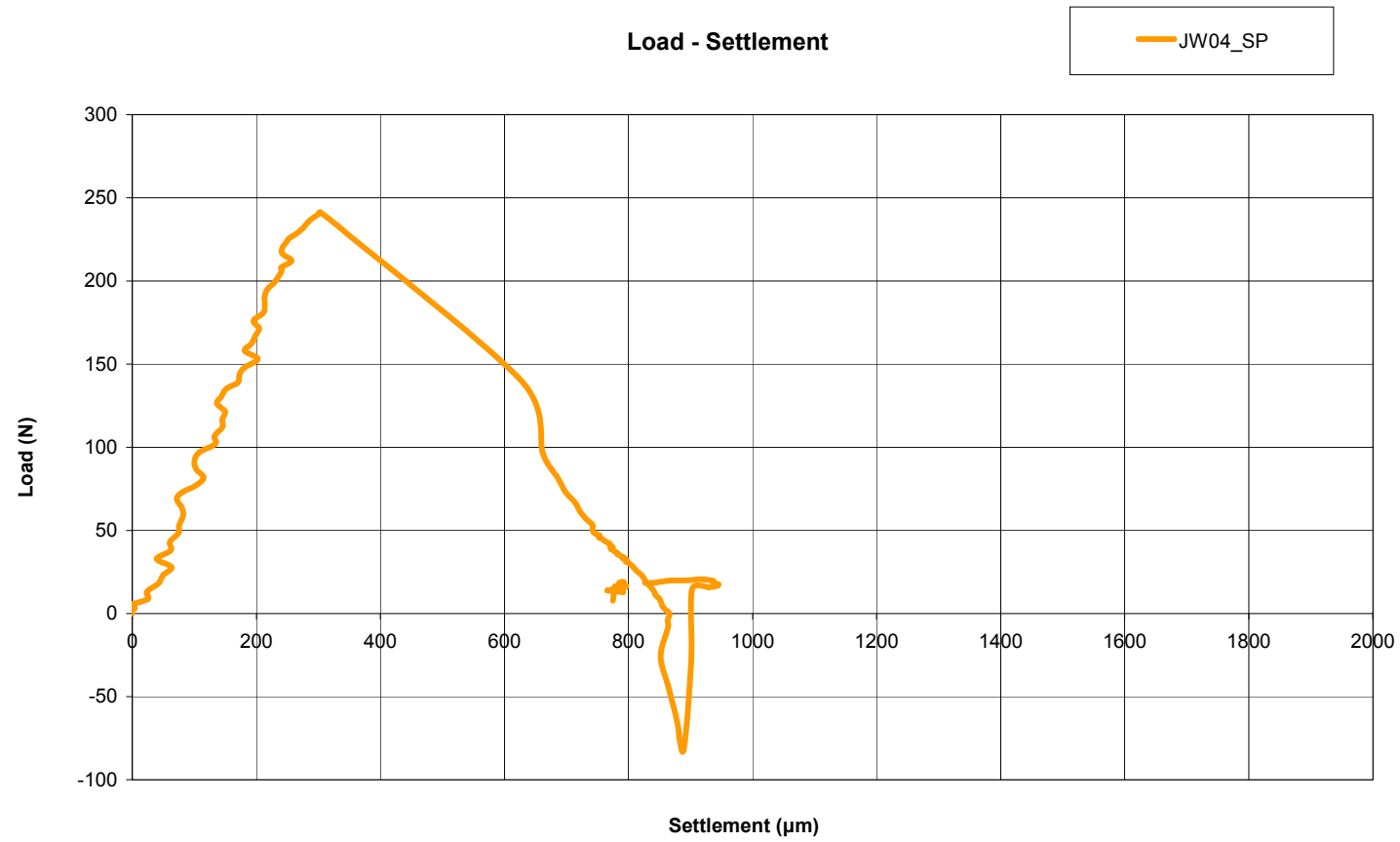
Figure 6.27 Test JW04: Load-Settlement Graph
