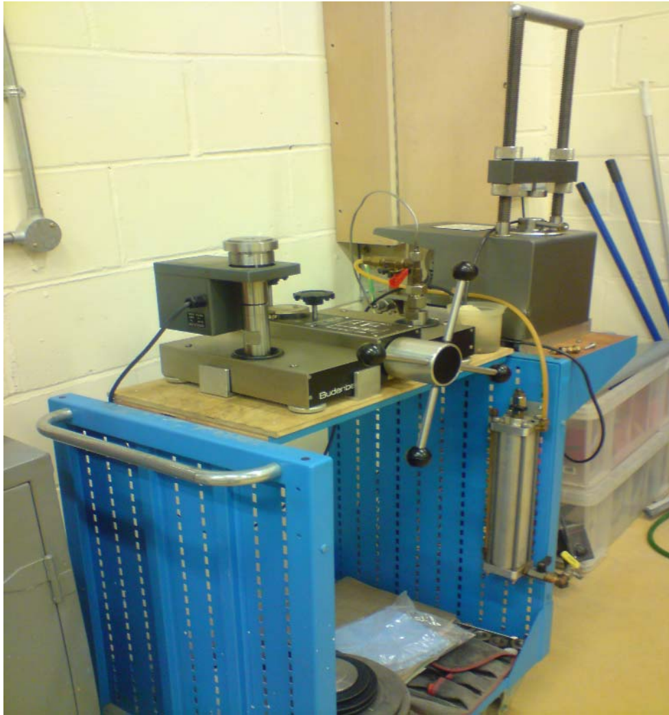
Figure 5.3 Photograph of the Budenburg for calibration of the load cells
