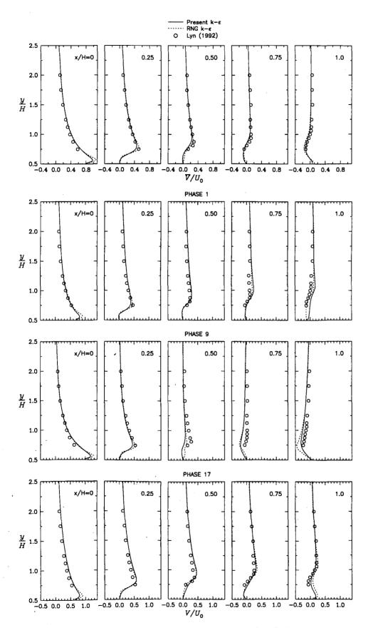
Figure 5.22: Computed and measured time-averaged and phase-averaged (phases 1, 9 and 17) lateral velocity profiles at several lateral cross-sections along the top face of a square cylinder.
