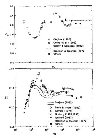
Figure 1.3: Vortex shedding parameters vs. *Re* for a smooth square cylinder in a uniform low-turbulence stream: the mean drag coefficient (top) and Strouhal number (bottom). Single *Re*-number results marked as 'others': Pocha (1971), Lee (1975), Bearman and Obasaju (1982), Obasaju (1983), Sarpkaya and Ihrig (1986), Durao et al. (1988) and Lyn (1992).
