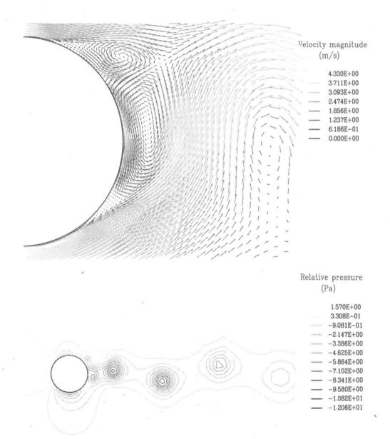
Figure 5.25: Flow past a circular cylinder at  $Re = 1.4 \times 10^5$ . Velocity vectors (top) and pressure contours (bottom) as computed by the unsteady  $k - \epsilon$  model at  $t^* = 117.6$  (minimum  $C_L$ ).
