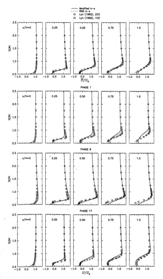
Figure 5.21: Computed and measured time-averaged and phase-averaged (phases 1, 9 and 17) axial velocity profiles at several lateral cross-sections along the top face of a square cylinder.
