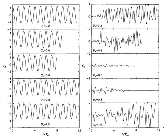
Figure 4.37: Circular cylinder in current plus oscillations. Time histories of the drag (left) and lift (right) coefficients as a function of velocity ratio.
