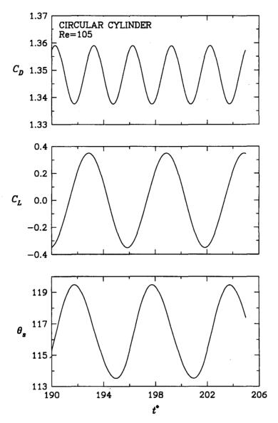
Figure 4.13: Developed vortex shedding from a circular cylinder at Re = 105: the drag coefficient (top), lift coefficient (middle), and angle of separation (bottom).
