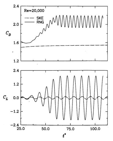
Figure 5.3: Turbulent flow past a square cylinder at Re = 20,000. Time evolution of the drag (top) and lift (bottom) coefficients as predicted by the standard and RNG  $k - \epsilon$  models (grid  $D1 - 139 \times 122(a)$ , SMART scheme).
