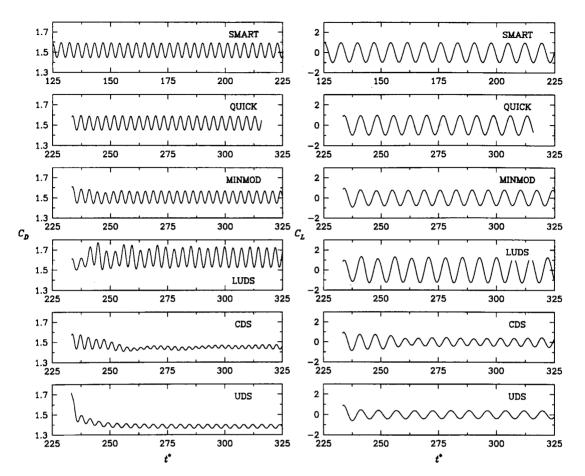
Figure 4.16: Flow past a square cylinder at Re = 250. Time history of the drag (left) and lift (right) coefficient as obtained with various convective schemes (grid D1-136x118,  $\Delta t^* = 3.89 \times 10^{-3}$ ).
