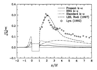
Figure 5.6: Effects of the  $k - \epsilon$  turbulence models on the time-averaged centreline distribution of the turbulent kinetic energy for the flow past a square cylinder at Re = 20000.
