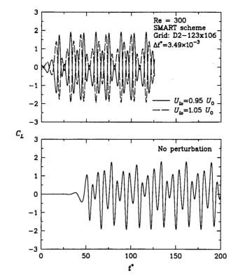
Figure 4.24: Flow around a square cylinder at Re = 300. Time traces of the lift coefficient as calculated with two initial perturbations (top) and without it (below).
