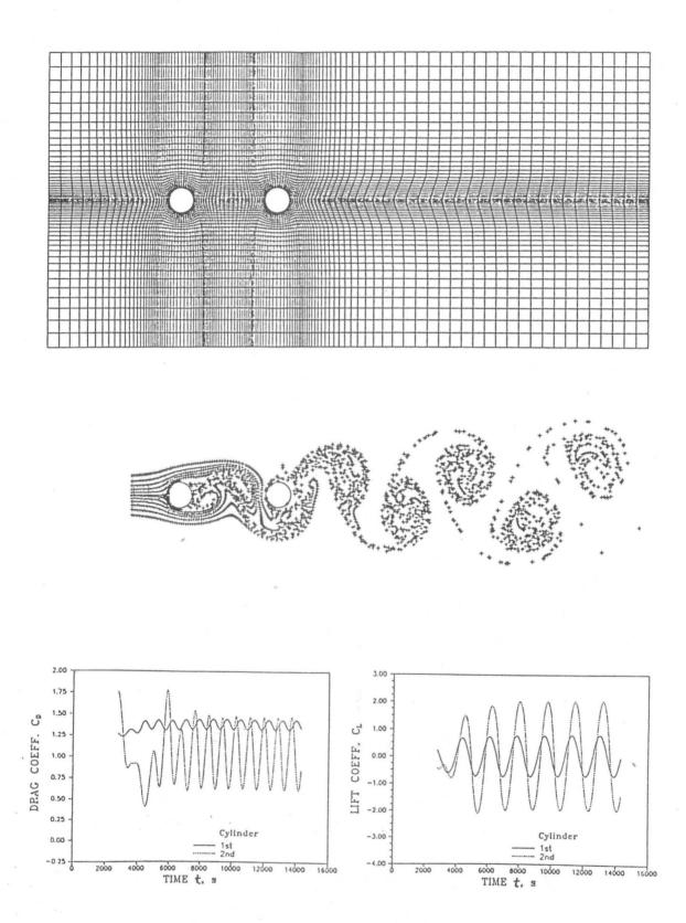
Figure 4.31: Two circular cylinders in line with the spacing ratio L/D = 4: the grid (top), streaklines for Re = 200 (middle) and time histories of the drag and lift coefficients also at Re = 200 (bottom).
