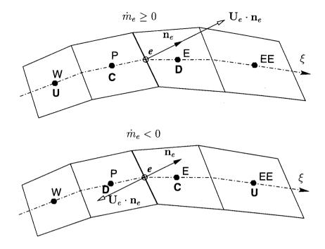
Figure 3.2: Definition of upstream, central and downstream cells.
