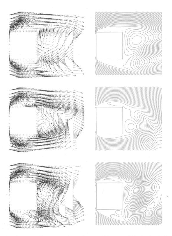
Figure 4.23: Velocity vectors and streamlines around a square cylinder showing the flow reattachment at the cylinder sides: (top) Re = 300, (middle) Re = 500, and (bottom) Re = 1000 (grid D1-136x118, SMART scheme).
