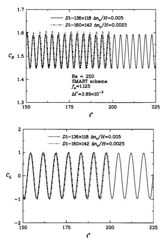
Figure 4.19: Flow past a square cylinder at Re = 250. Effect of the near-wall distance on the drag coefficient (above) and the lift coefficient (below).
