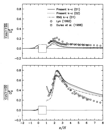
Figure 5.17: Centreline distributions of predicted and measured time-mean apparent normal Reynolds stresses in x (top) and y (bottom) directions (Re = 20000).
