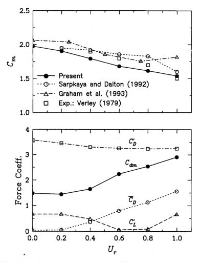
Figure 4.38: Circular cylinder in current plus oscillations. Morison's inertia coefficient (top) and other force coefficients (bottom) as obtained with Kc = 4 and  $\beta = 200$  (present results: grid 98 × 64,  $\Delta t^* = 2.5 \cdot 10^{-3}$ , SMART scheme).
