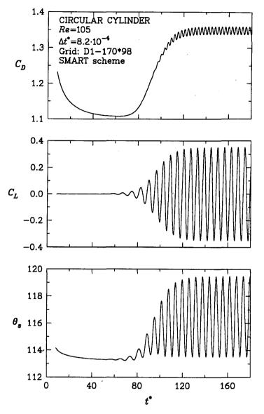
Figure 4.5: Time histories for the flow past a circular cylinder at Re = 105: drag coefficient (top), lift coefficient (middle), and angle of separation (bottom).
