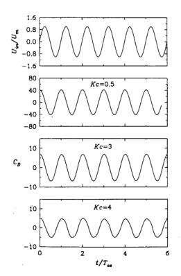
Figure 4.34: Circular cylinder in pure oscillatory flows. Computed drag coefficients versus time at Kc = 0.5, 3, and 4 and  $\beta = 196$  (the top curve shows the inlet velocity variation).
