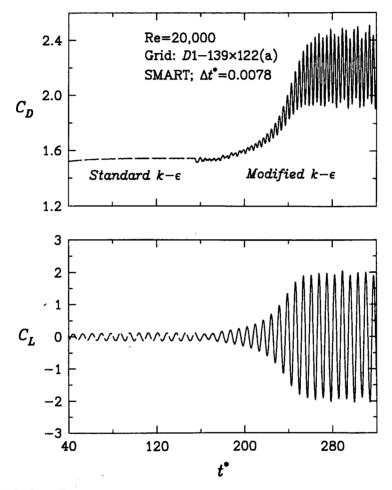
Figure 5.5: Turbulent flow past a square cylinder at Re = 20,000. Time evolution of the drag (top) and lift (bottom) coefficients as predicted by the  $k - \epsilon$  model before and after the unsteady modification.
