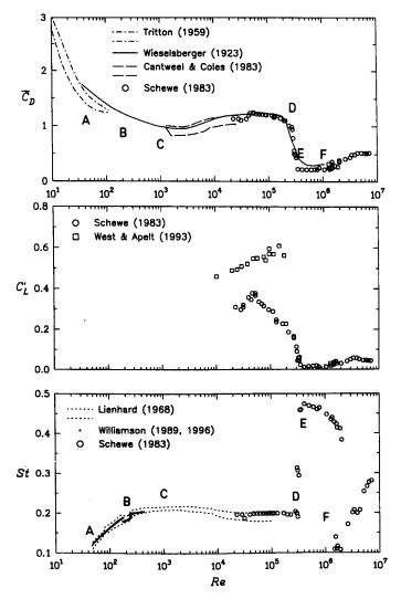
Figure 1.2: Vortex shedding parameters vs. *Re* for a smooth circular cylinder in a uniform low-turbulence stream: the mean drag coefficient (top), r.m.s. lift coefficient (middle) and Strouhal number (bottom).
