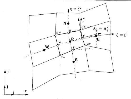
Figure 3.1: A typical control volume and the points-of-compass notation used for the cell-centred two-dimensional structured grid ( $\bullet$ , locations of variables solved for;  $\circ$ , locations where fluxes are required).
