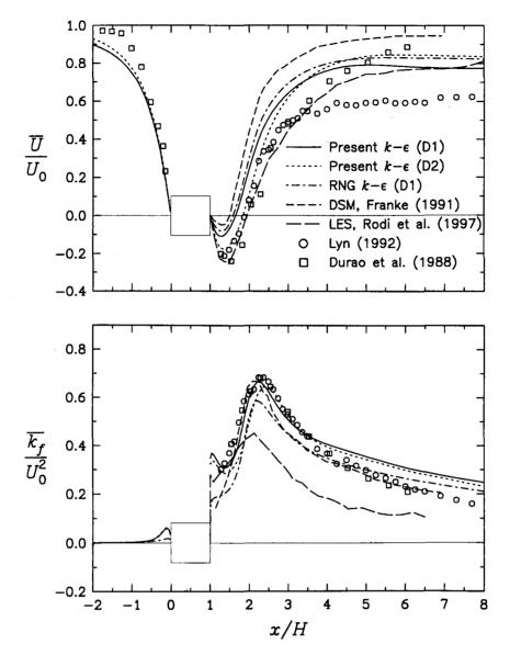
Figure 5.16: Predicted and measured time-averaged velocity (top) and total fluctuating kinetic energy (bottom) along the centreline (Re = 20000).
