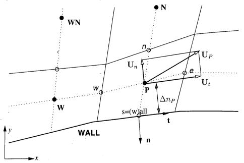
Figure 3.5: Application of the wall boundary conditions.
