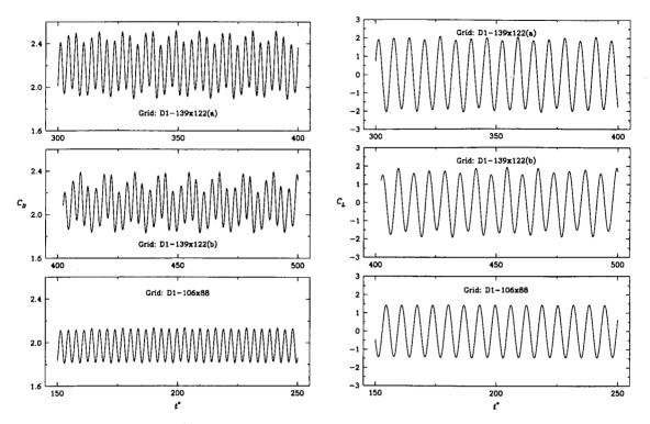
Figure 5.11: Turbulent flow around a square cylinder at Re = 20000. Time traces of the drag (left) and lift (right) coefficients as obtained on three different numerical grids (the present  $k - \epsilon$  model with the SMART scheme and  $\Delta t^* = 0.0078$ ).
