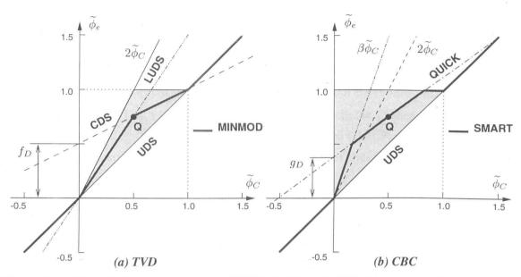
Figure 3.4: Graphical representation of TVD (left) and CBC (right) criteria and NVD characteristics of some bounded schemes.
