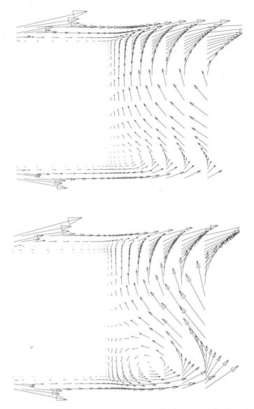
Figure 4.21: Velocity vectors around a square cylinder as calculated at two Reynolds numbers: (top) Re = 100, (bottom) Re = 150 (grid D1-136x118, SMART scheme).
