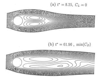
Figure 4.6: Streamline patterns for the flow past a circular cylinder at Re = 105: (a) symmetrical wake at  $t^* = 8.25$ ; (b) asymmetrical vortices at the instant  $t^* = 61.96$  when the drag coefficient has a minimum value (see also Fig. 4.5).
