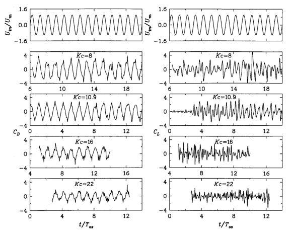
Figure 4.35: Circular cylinder in pure oscillatory flows. Computed drag (left) and lift (right) coefficients versus time at various higher Kc-numbers for  $\beta = 196$  (top curves show the inlet velocity variation).
