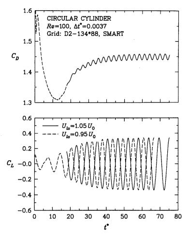
Figure 4.4: Circular cylinder at Re = 100. Time histories of the drag coefficient (top) and lift coefficient (bottom) as obtained with two initial asymmetric perturbations.
