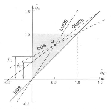
Figure 3.3: NVD diagram for several convective schemes.
