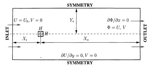
Figure 4.1: Typical solution domain and boundary conditions.
