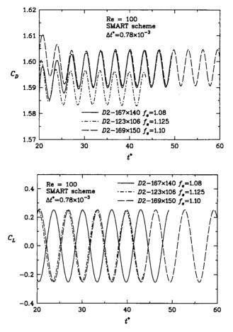
Figure 4.18: Flow past a square cylinder at Re = 100. Effect of the grid expansion on the drag coefficient (above) and lift coefficient (below).
