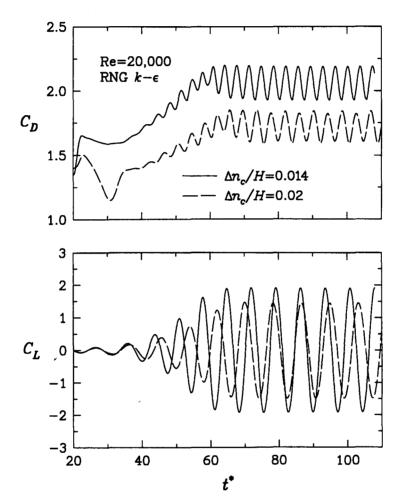
Figure 5.4: Turbulent flow past a square cylinder at Re = 20,000. Time evolution of the drag (top) and lift (bottom) coefficients as predicted by RNG  $k - \epsilon$  model with two near-wall cell distances (grids  $D1 - 139 \times 122(a, b)$ , SMART scheme).
