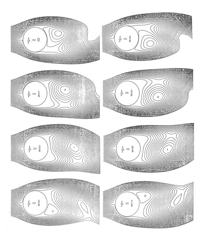
Figure 4.9: Periodic vortex shedding from a circular cylinder at Re = 105. Streamlines in the near wake representing a complete shedding cycle (successive plots at intervals of T/8).
