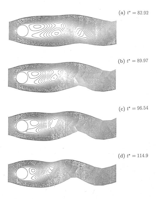
Figure 4.8: Development of vortex shedding past a circular cylinder at Re = 105. Streamline patterns obtained at moments when the lift coefficient has maximum values illustrate reduction of the recirculation region and disappearance of two coexisting shed vortices. LAMINAR FLOW PREDICTIONS 4.3 Periodic Vortex Shedding: Common Features
