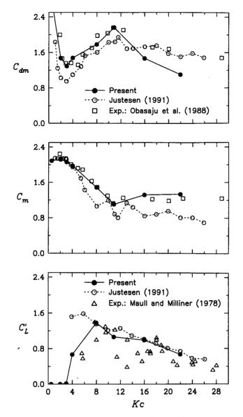
Figure 4.36: Circular cylinder in pure oscillatory flows. Comparisons of Morison's drag (top) and inertia (middle) coefficients and the root-mean-square lift coefficient (bottom).
