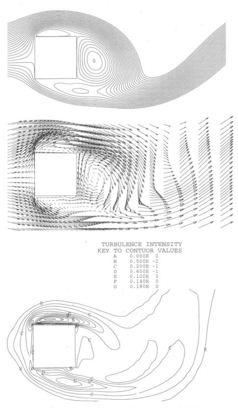
Figure 5.14: Instantaneous streamlines (top), velocity vectors (middle) and turbulent kinetic energy contours (bottom) as computed by the present  $k - \epsilon$  model at the phase corresponding to the maximum  $C_L$ .
