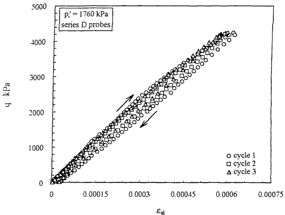
Figure 6.21 Stress-strain relationships from undrained loading probes performed on the silica sandstone ( $q_{\max} = 4200$  kPa).
