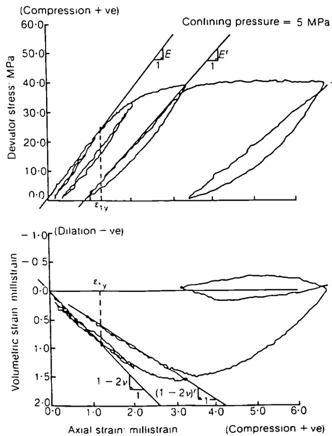
Figure 2.31 Determinations of the yield point for an oolitic limestone (after Elliott and Brown, 1985).
