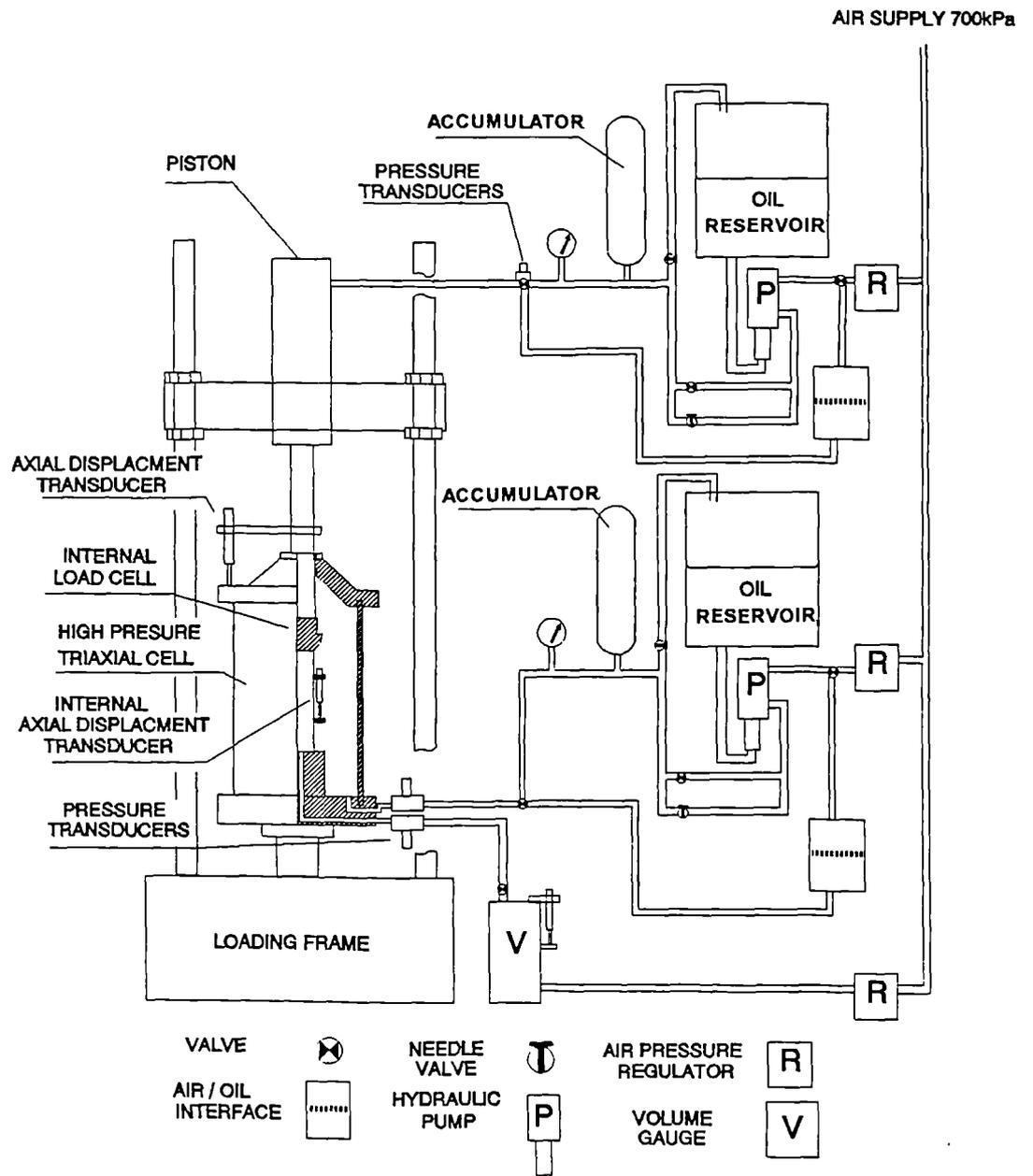
Figure 3.3 Schematic diagram of the 10 MPa triaxial system after modifications.
