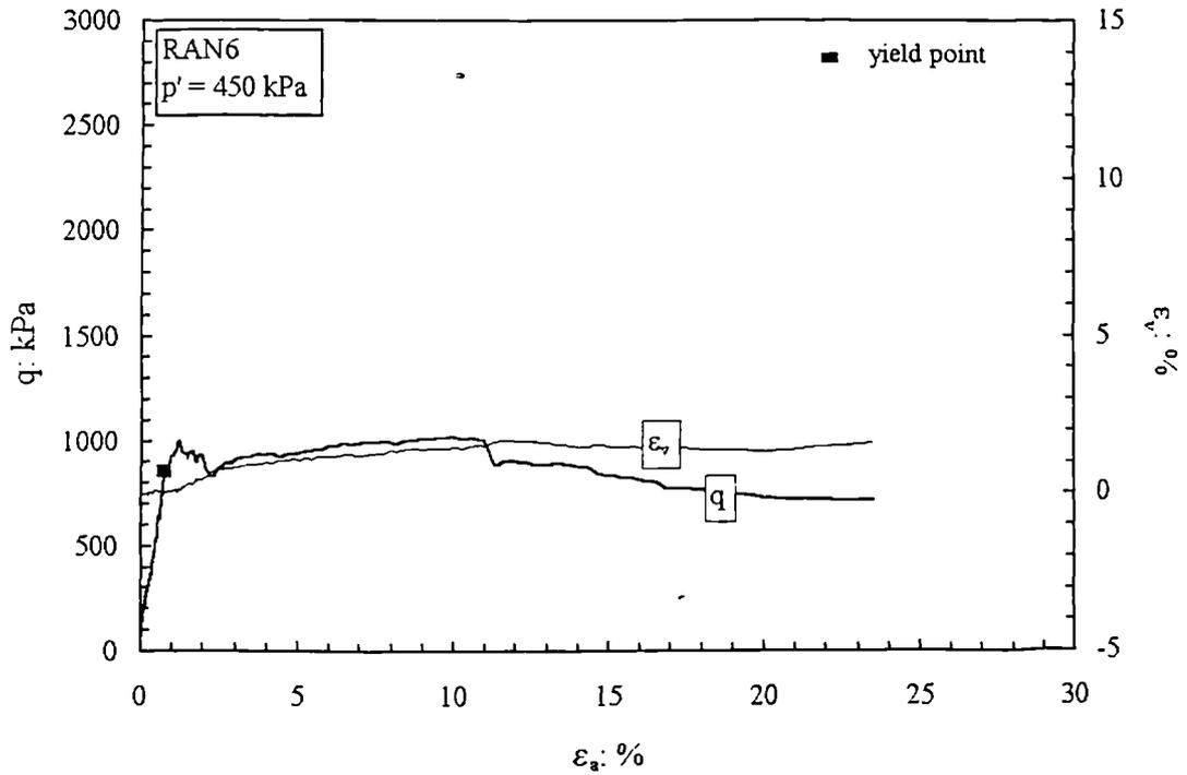
Figure 5.5 Stress-strain curve from a drained constant  $p'$  test performed on the calcarenite at low confining pressures (after Coop and Atkinson, 1993).
