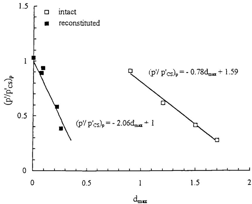
Figure 7.16 Normalized states at peak for reconstituted and intact samples of silica sandstone referred to the CSL of the reconstituted soil.
