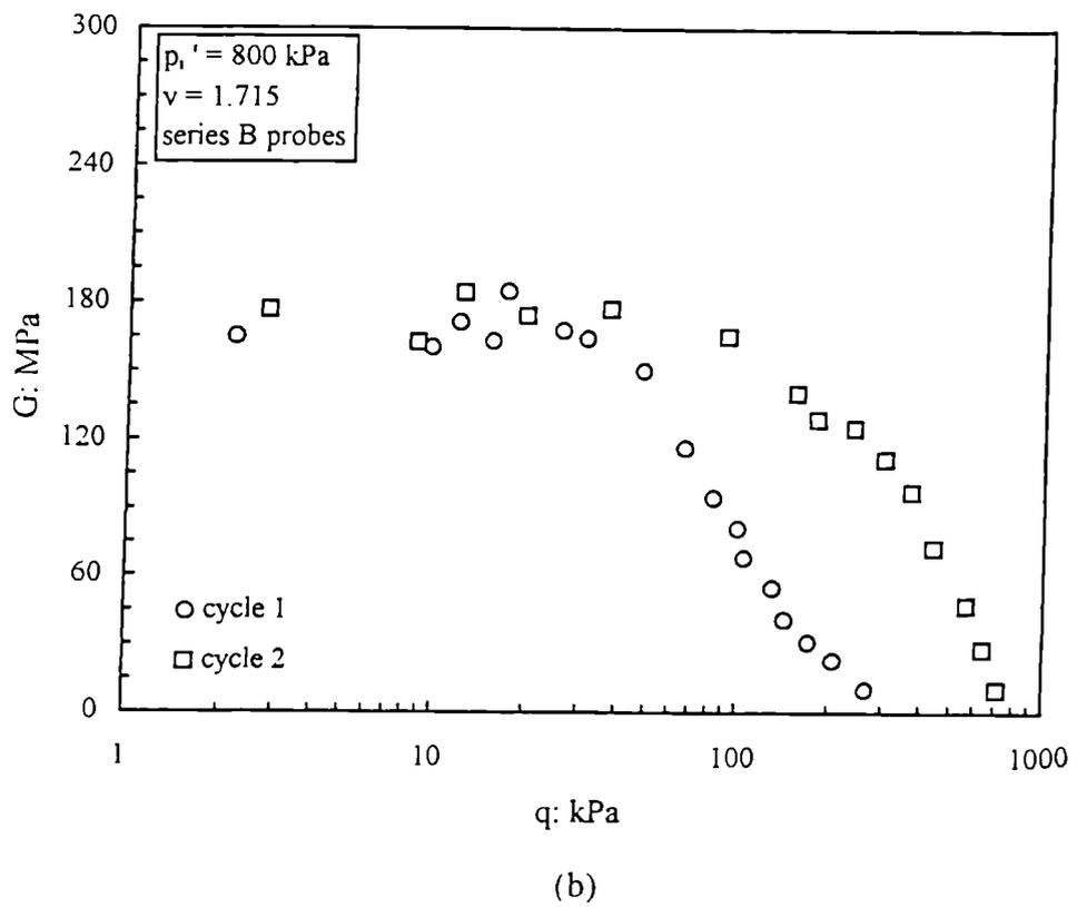
Figure 5.23 Variation of the tangent shear moduli with deviator stress from undrained loading probes on a reconstituted sample of calcarenite performed for different values of  $p_i'$ .
