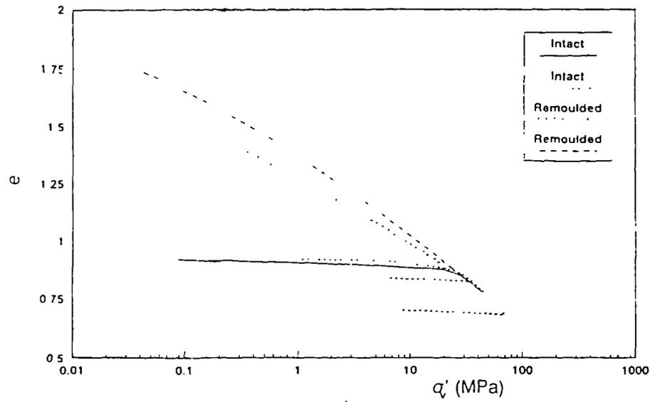
Figure 2.24 One-dimensional compression for intact and reconstituted samples of a fine grained tuff (after Aversa, 1991).
