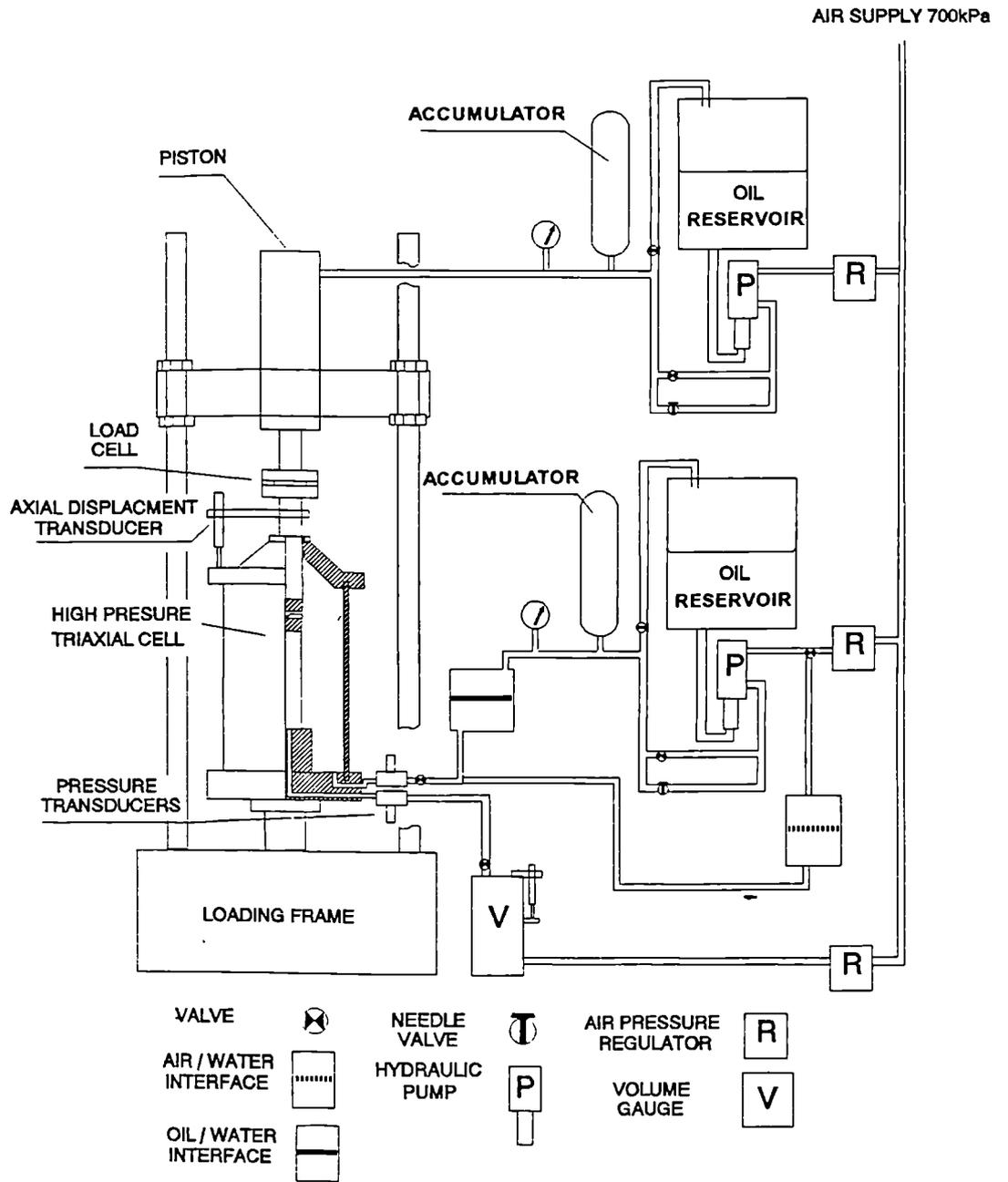
Figure 3.1 Schematic diagram of the high pressure system.
