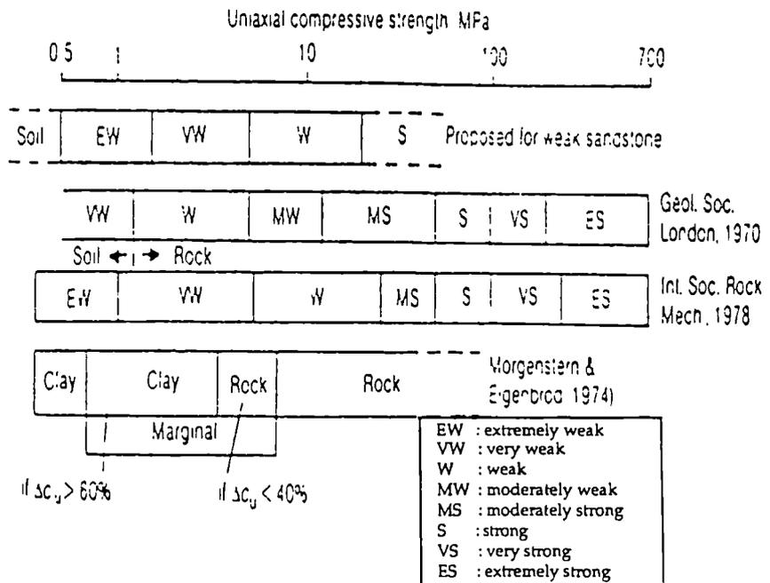
Figure 2.21 Some classification systems of soils and rocks (after Dobereiner and De Freitas, 1986).
