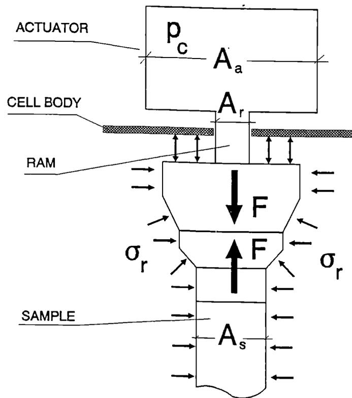
Figure 3.2 Schematic diagram of the axial loading system.
