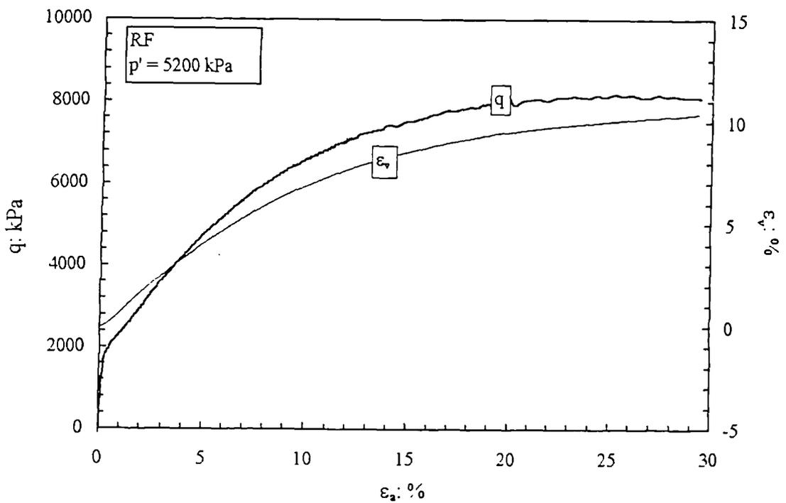
Figure 5.11 Stress-strain curve from a drained constant  $p'$  tests performed on reconstituted soil of calcarenite at high confining pressures.
