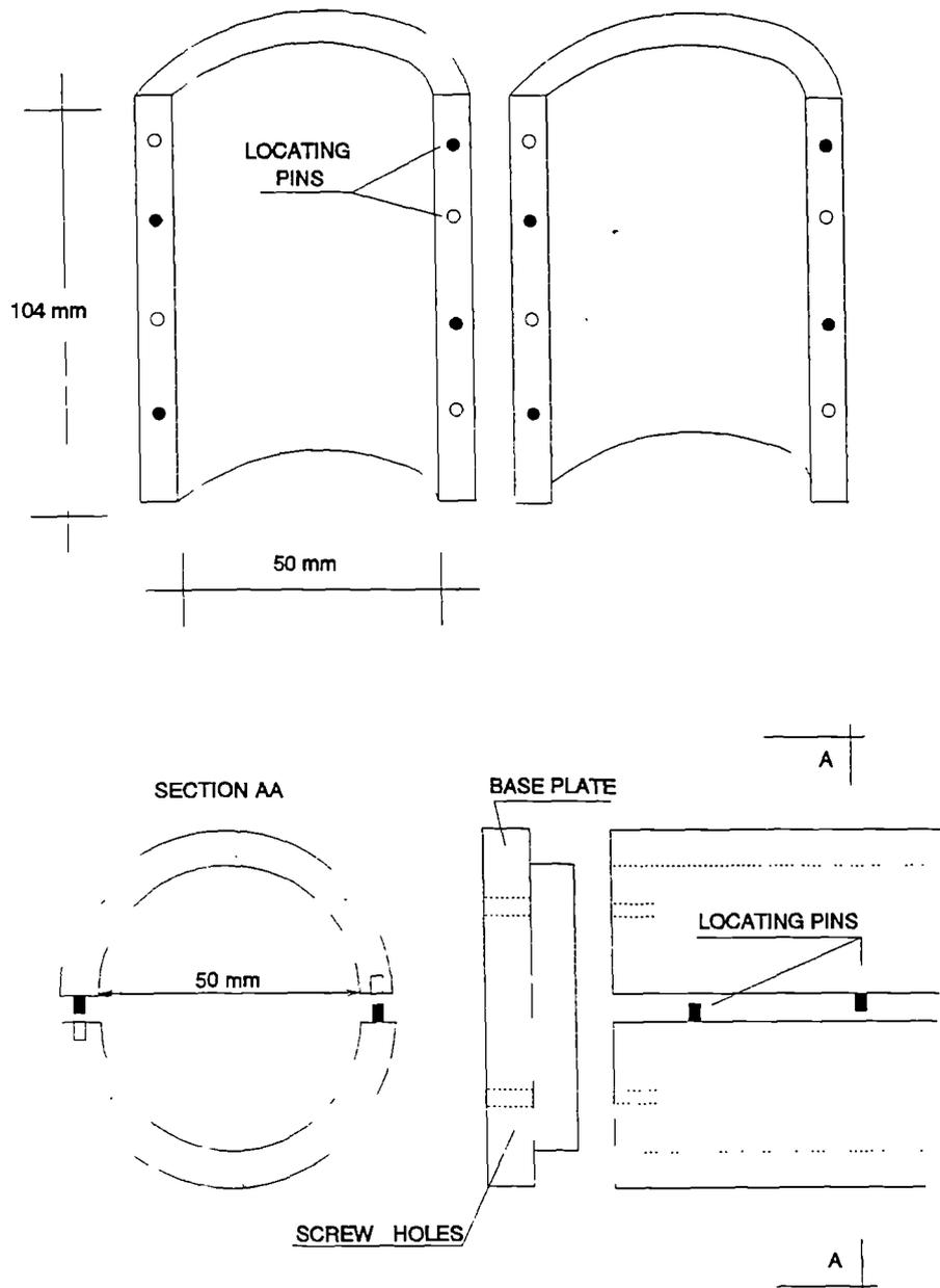
Figure 3.13 Mould for trimming the ends of the sample.
