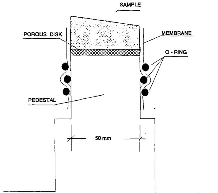
Figure 3.18 Configuration of 'O'-rings to seal the sample.
