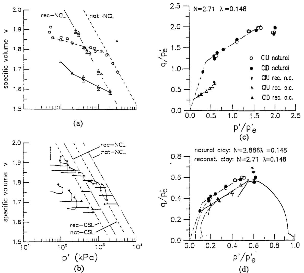
Figure 2.12 Comparison between natural and reconstituted Vallerica clay: (a) isotropic compression; (b) stress-volume paths during shearing; (c) peak states normalized by a  $p_e'$  taken on the reconstituted NCL; (d) peak states normalized by a  $p_e'$  taken on the appropriate NCL (after Rampello et al., 1993).
