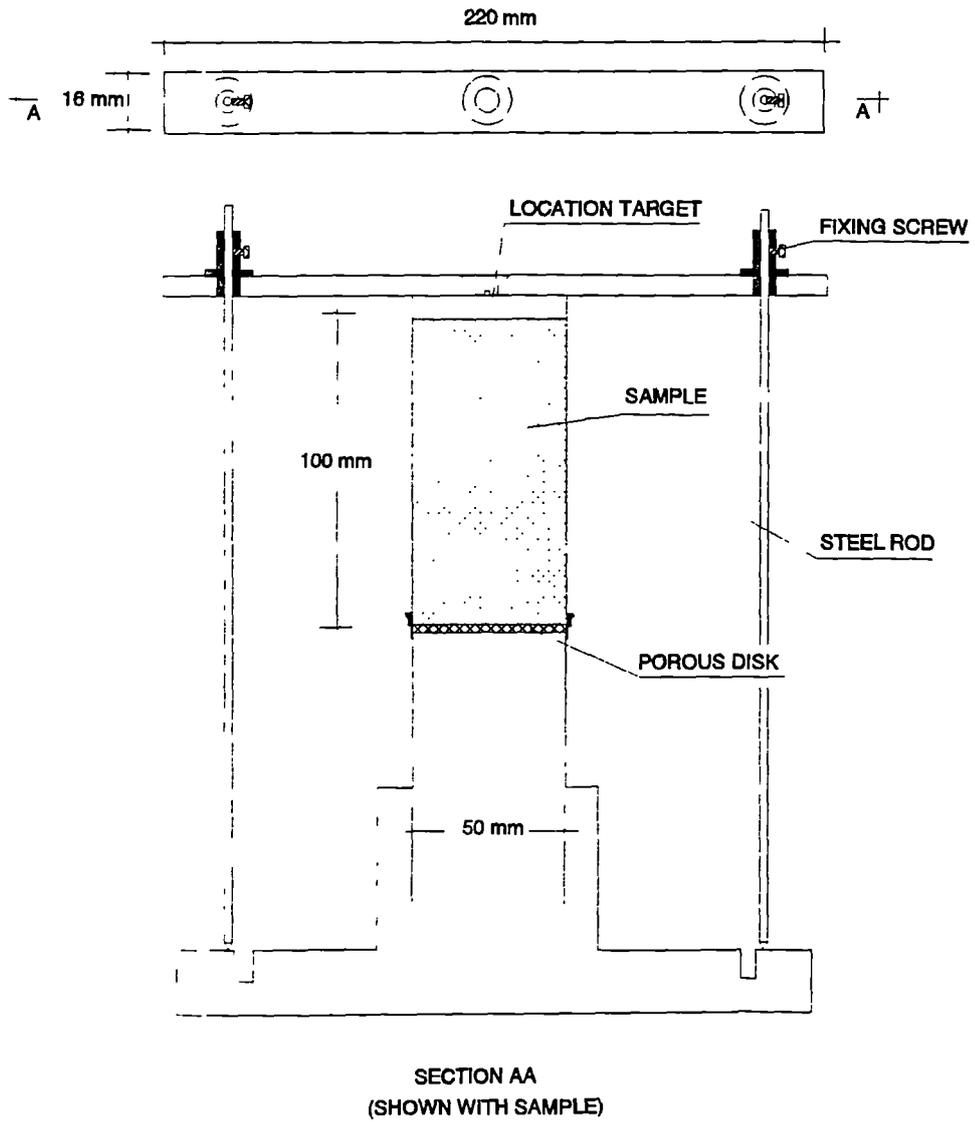
Figure 3.16 Device to check the perpendicularity of the ends of the sample with respect to the apparatus axes.
