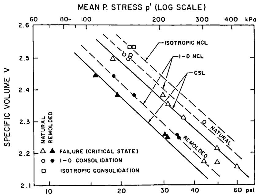
Figure 2.5b Loci of isotropic and one-dimensional preconsolidation pressures ( $\sigma'_{vc}$  in Figure 2.5a) and critical states for Winnipeg clay (after Graham and Li, 1985).
