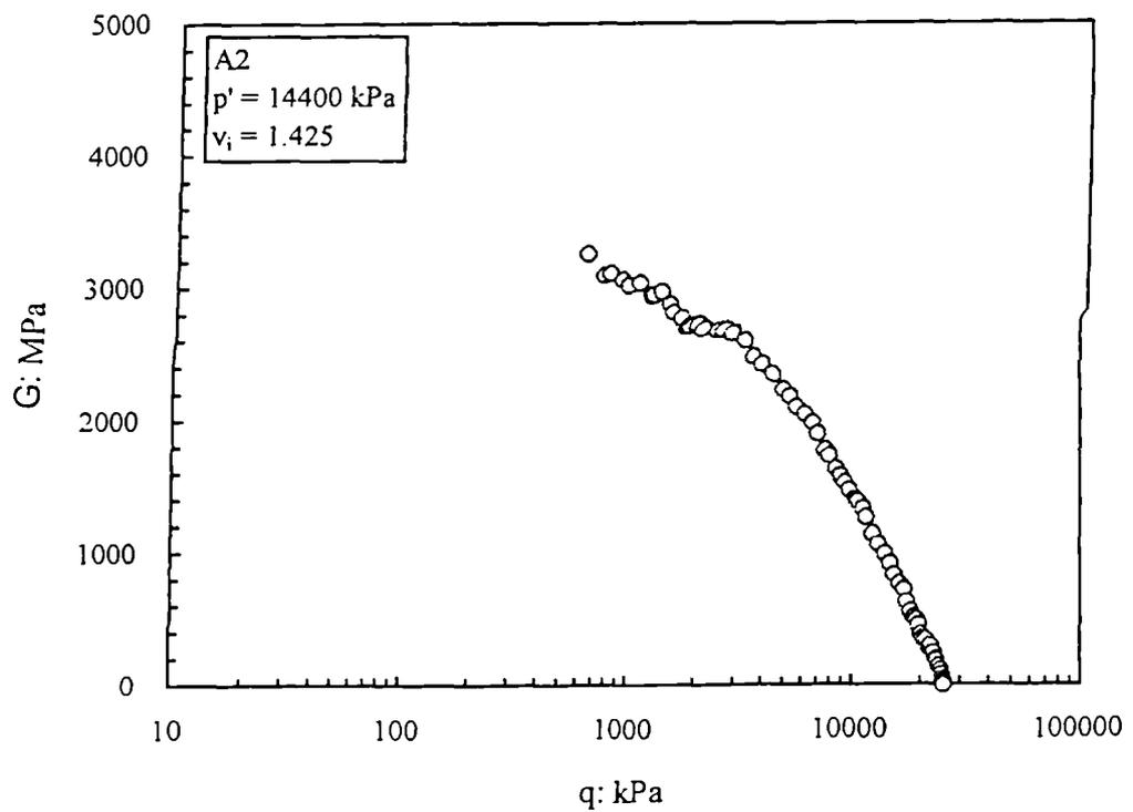
Figure 6.16 Tangent shear modulus as a function of deviator stress for a constant  $p'$  stress path tests performed at high confining pressures.
