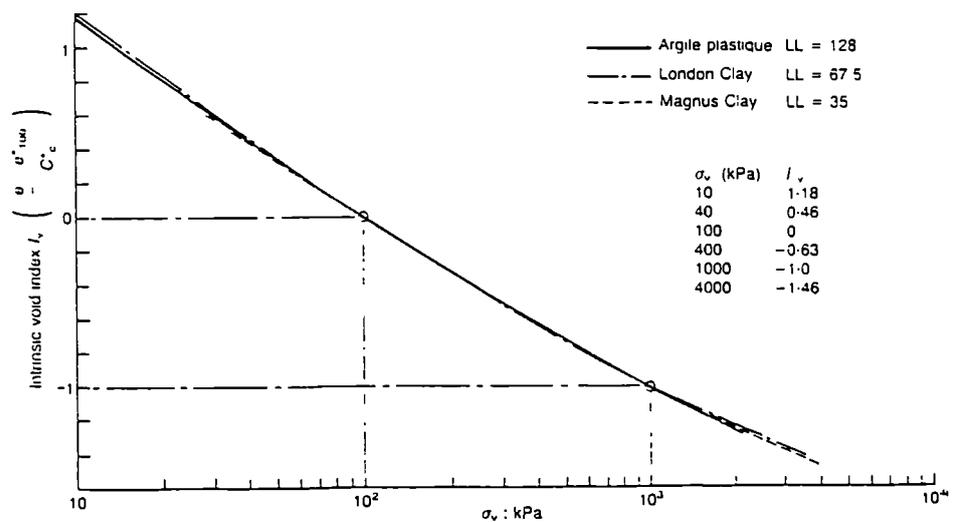
Figure 2.7 Normalized one-dimensional compression curves of reconstituted clays (after Burland, 1990).
