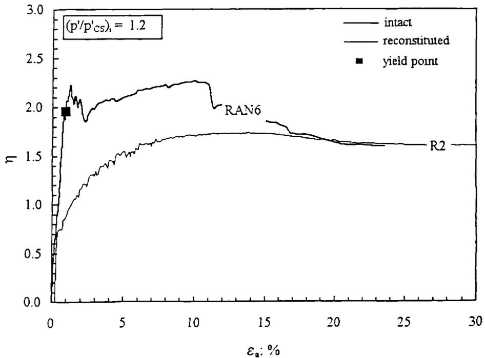
Figure 5.15 Shear behaviour of intact (after Coop and Atkinson, 1993) and reconstituted samples of calcarenite tested from similar initial values of  $p'/p'_{cs}$  at low confining pressures (constant  $p'$  tests).
