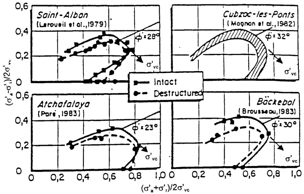
Figure 2.10 State boundary surfaces for intact and destructured clays (after Tavenas and Leroueil, 1987).
