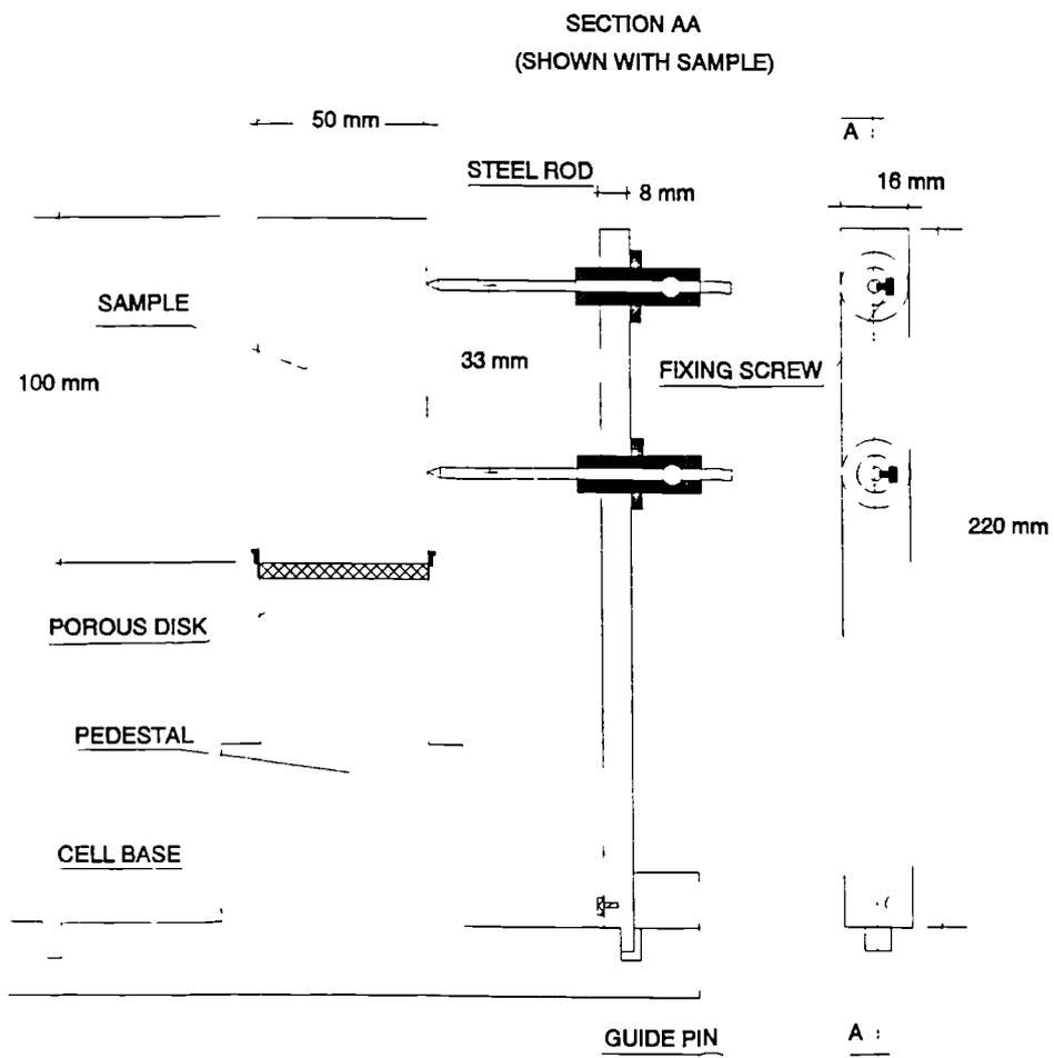
Figure 3.15 Device to check the sample centrality with respect to the apparatus axis.
