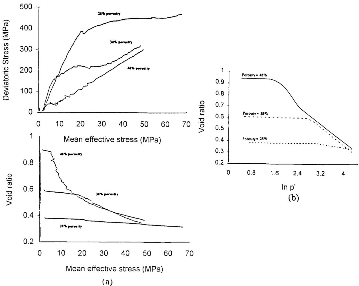
Figure 2.23 One-dimensional compression for samples of chalk with different initial void ratios: (a) after Leddra, 1990; (b) after Petley et al., 1993.
