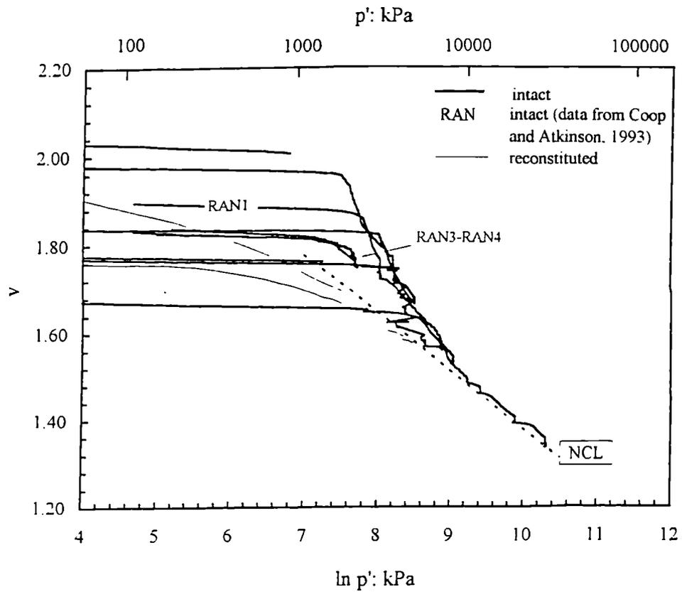
Figure 5.3 Isotropic compression of intact and reconstituted samples of calcarenite.
