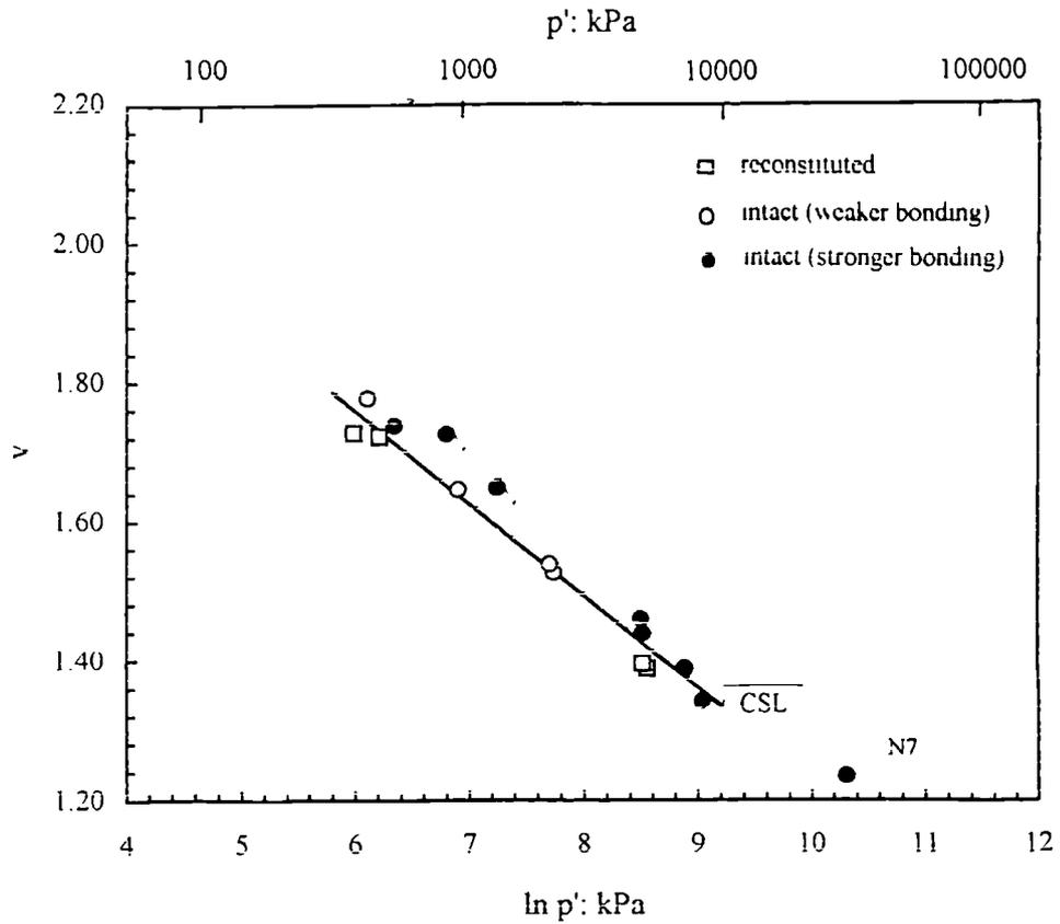
Figure 5.14 States at the end of shearing for intact and reconstituted samples of calcarenite.
