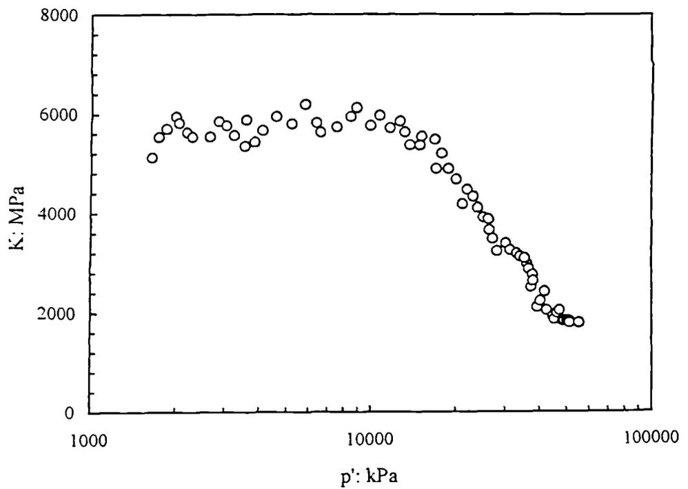
Figure 6.26 Variation of the bulk modulus of the silica sandstone with mean effective stress.
