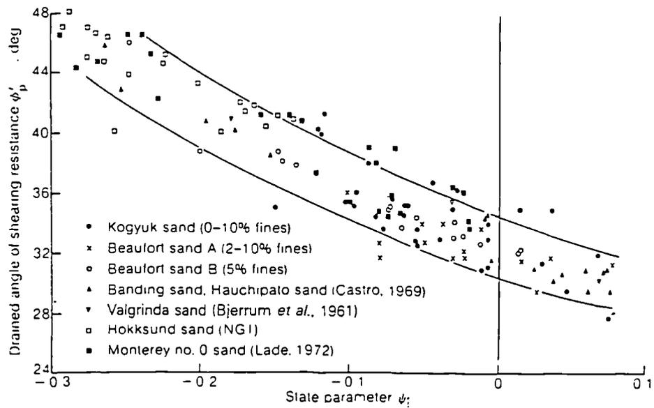
Figure 2.15 Variation of the peak angle of friction of sands with the state parameter  $\psi_i$  (after Been and Jefferies, 1985).
