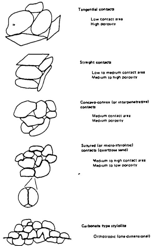
Figure 2.18 Intergranular fabric classification (after Dusseault and Morgenstern, 1979).
