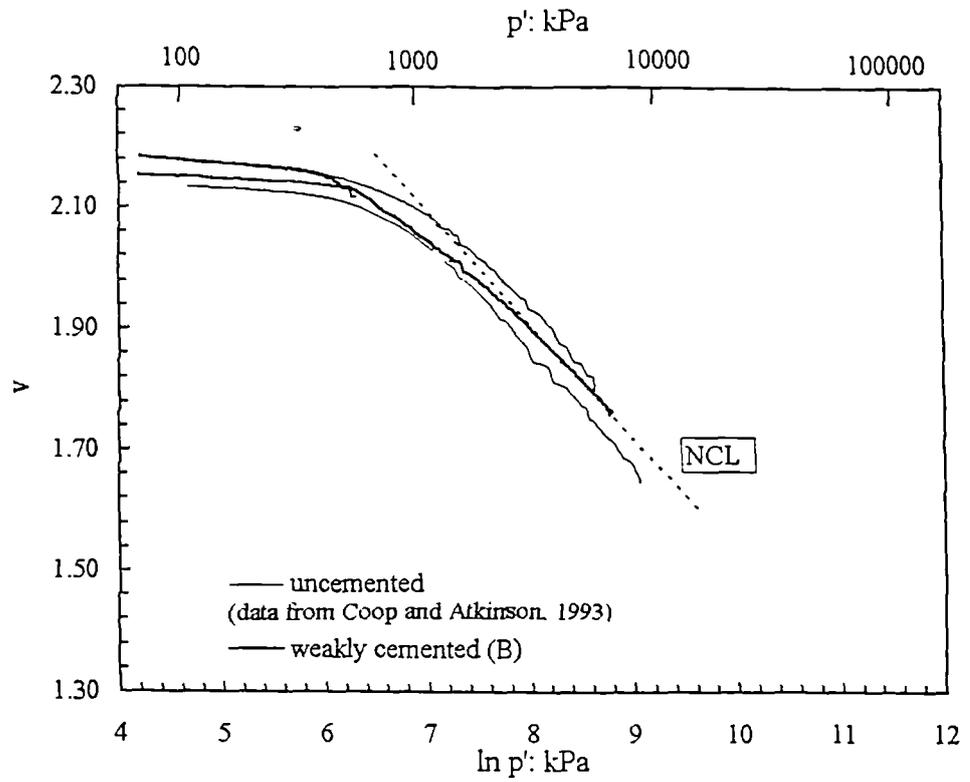
Figure 4.3a Isotropic compression of the weakly cemented sand prepared using method B and of the uncemented sand.
