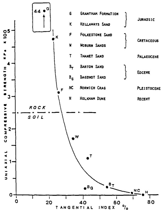
Figure 2.19 Unconfined compressive strength as a function of the tangential index (TI %) for a group of locked sands from the U.K. (after Dobereiner and De Freitas, 1986).
