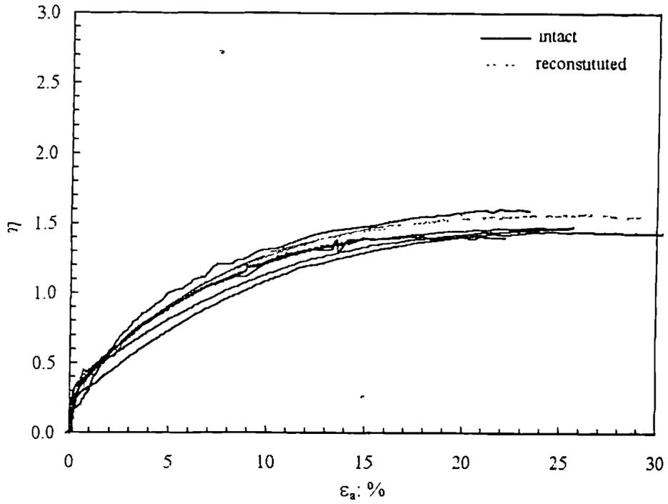
Figure 5.16 Shear behaviour of reconstituted and intact samples of calcarenite which yielded in isotropic compression (constant  $p'$  tests).
