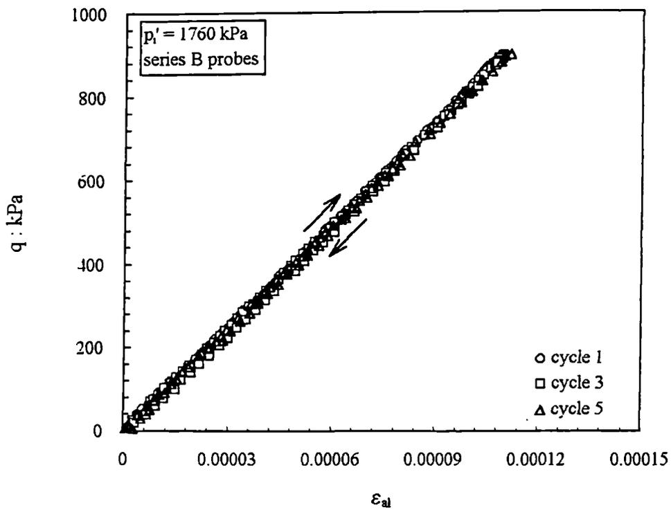
Figure 6.18 Pre-yield stress-strain relationships for undrained cycles performed on the silica sandstone.
