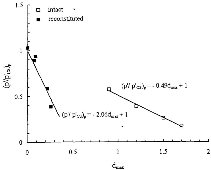
Figure 7.17 Normalized states at peak for reconstituted and intact samples of silica sandstone referred to the appropriate CSLs.
