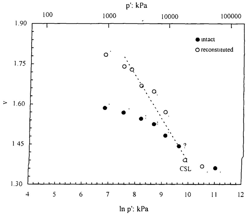
Figure 6.12 States at the end of shearing for intact and reconstituted samples of silica sandstone.
