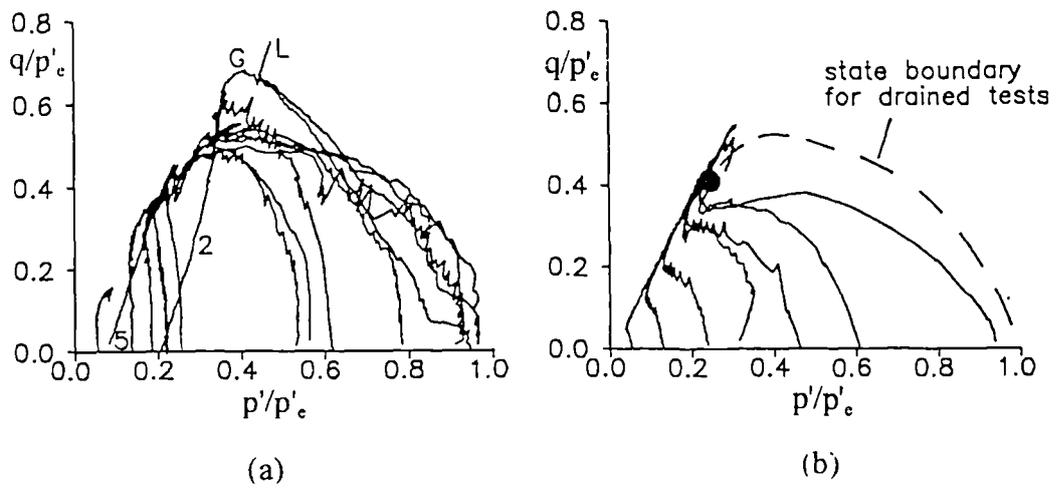
Figure 2.16 Normalized stress paths for Dog's Bay sand: (a) drained tests; (b) undrained tests (after Coop and Lee, 1993).
