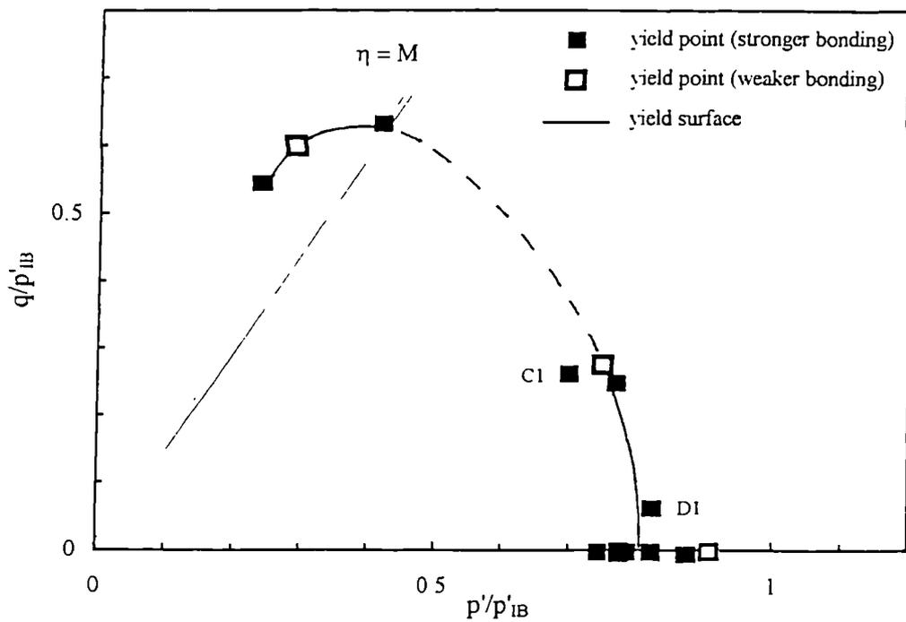
Figure 7.7 Yield surface for the calcarenite.
