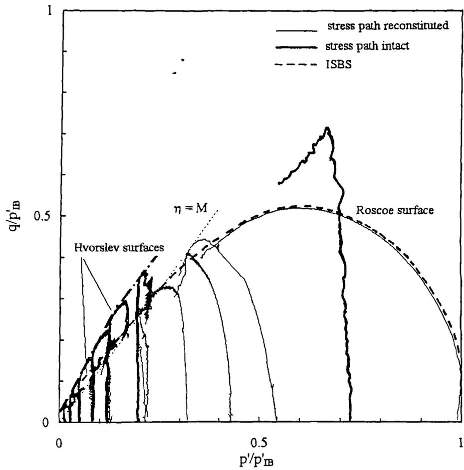
Figure 7.11 Normalized stress paths for intact and reconstituted samples of silica sandstone.
