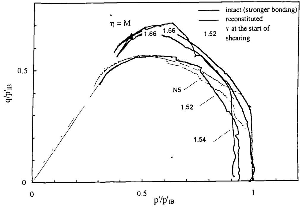
Figure 7.8a Normalized stress paths for reconstituted and intact samples of calcarenite with stronger bonding sheared after isotropic yielding.
