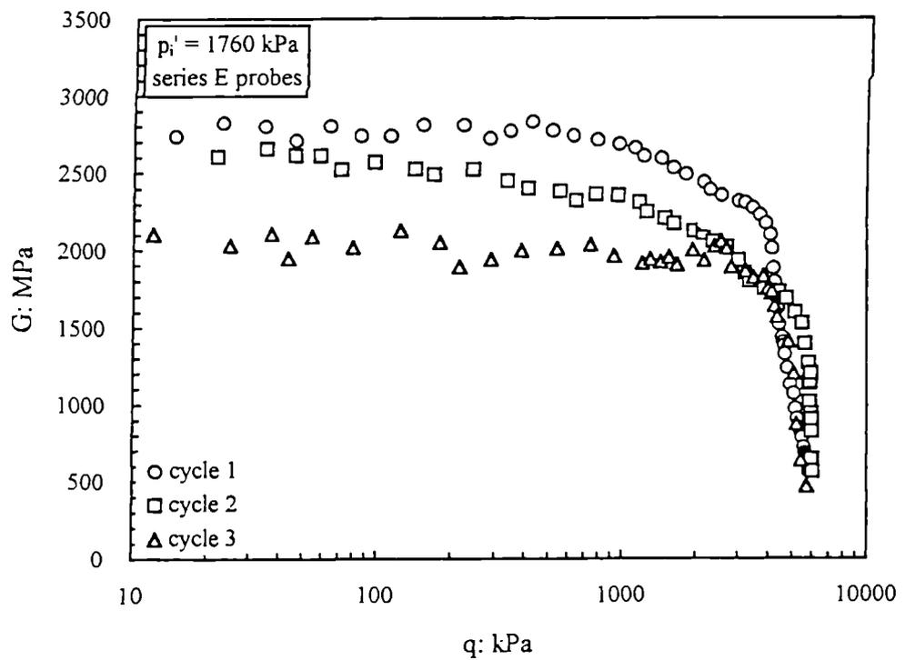
Figure 6.23 Tangent shear moduli from undrained probes performed on the silica sandstone ( $q_{\max} = 6000$  kPa).
