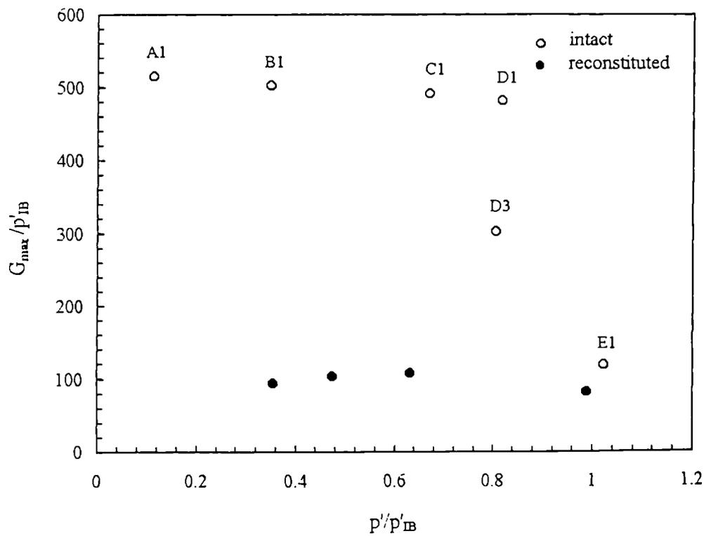
Figure 7.24 Comparison between the normalized maximum shear moduli of intact and reconstituted calcarenite as a function of the normalized state  $p'/p'_{IB}$ .
