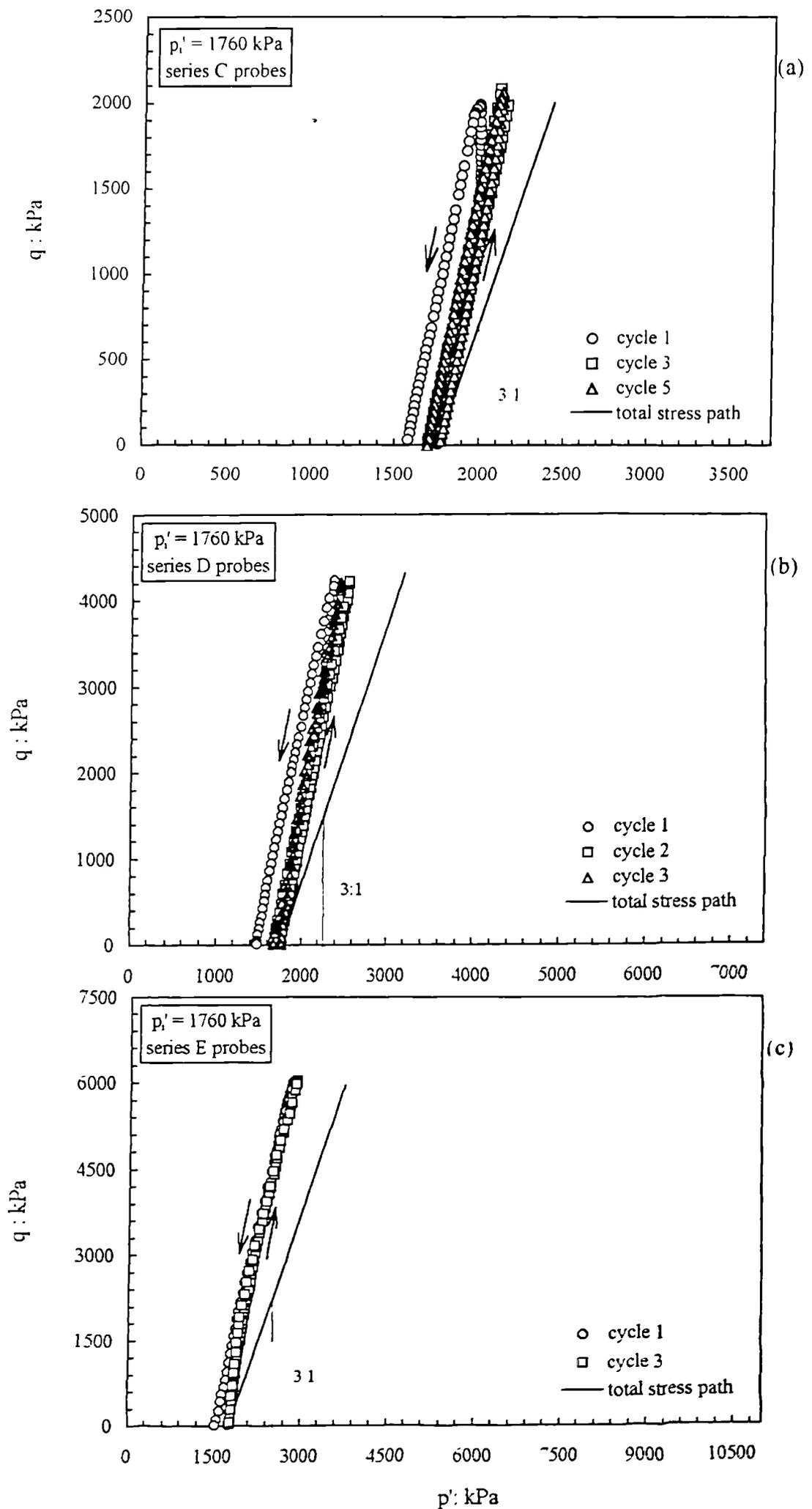
Figure 6.24 Effective stress paths for undrained cycles performed on the silica sandstone from the same isotropic state but up to different maximum deviator stresses.
