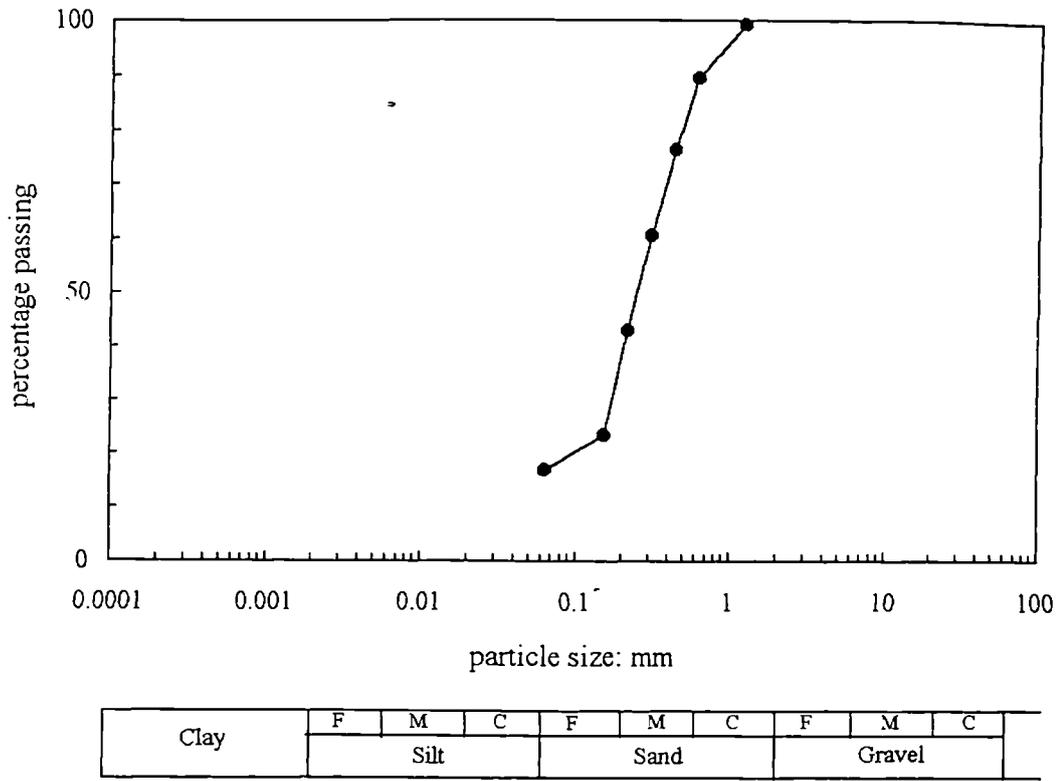
Figure 5.2 Grading curve determined for the reconstituted calcarenite.
