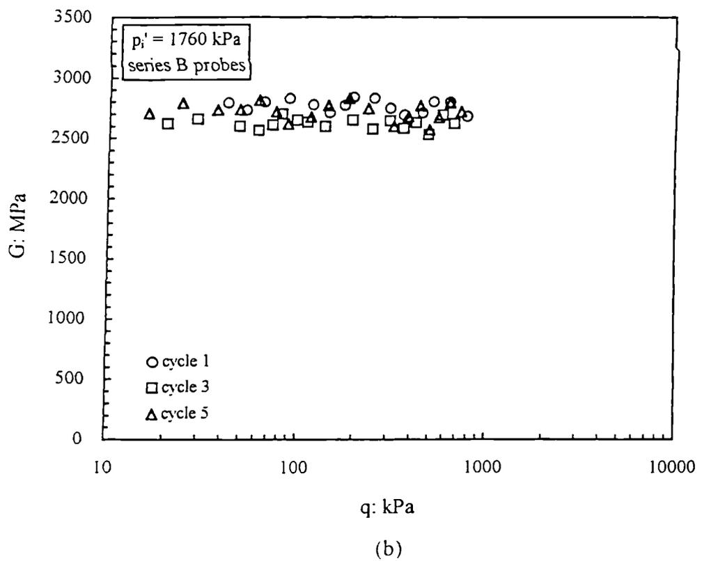
Figure 6.19 Tangent shear moduli as a function of (a) axial strain and (b) deviator stress obtained from undrained loading probes performed on the silica sandstone ( $q_{max} = 800$  kPa).
