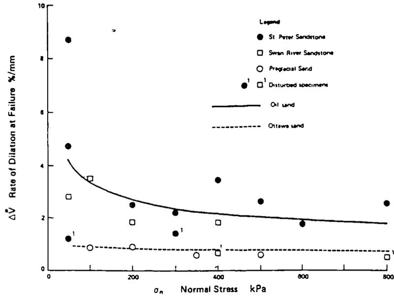
Figure 2.20 A comparison between the rate of dilatation at failure for shear box tests on locked sands (oil sands) and Ottawa sand (after Dusseault and Morgenstern, 1979).
