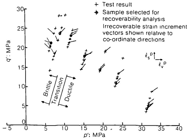
Figure 2.32 Stresses at yield for an oolitic limestone (after Elliott and Brown, 1985).
