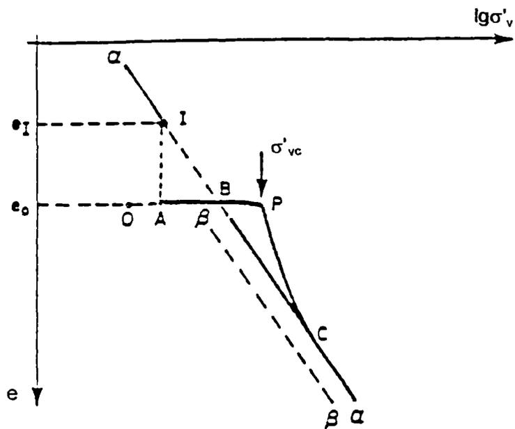
Figure 2.2 Schematic description of the consolidation of a natural clay deposit (after Tavenas and Leroueil, 1987).
