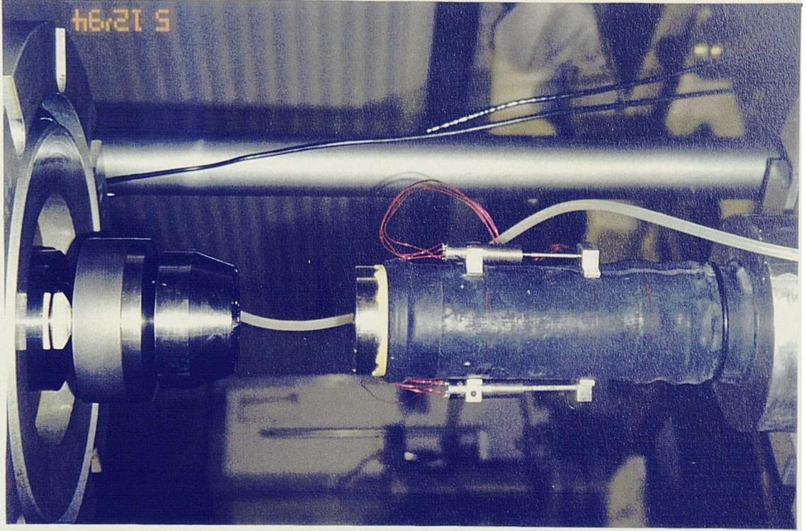
Figure 3.6 Arrangement of LYDTs in the 10 MPa apparatus.
