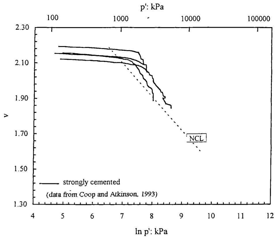
Figure 4.4 Isotropic compression of the strongly cemented sand.
