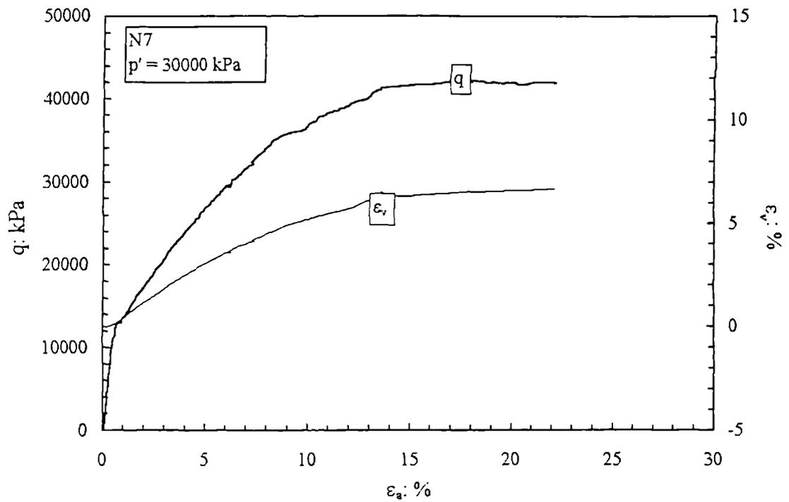
Figure 5.9 Stress-strain curve from a drained constant  $p'$  tests performed on the calcarenite at very high confining pressures.
