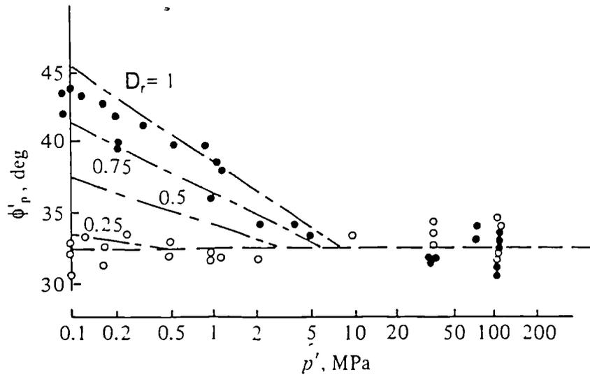
Figure 2.14 Variation of the peak angle of friction with mean effective stress and relative density  $D_r$  for initially loose ( $\circ$ ) and dense ( $\bullet$ ) samples of Chattahoochee River sand (after Vesic and Clough, 1968).
