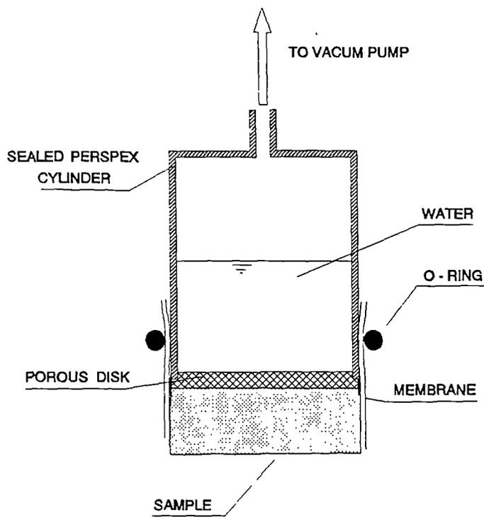
Figure 3.14 Device for the saturation of the sample.
