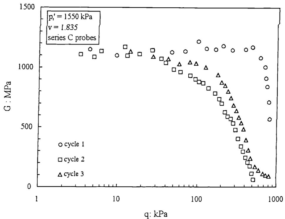
Figure 5.19b Variation of the tangent shear moduli with deviator stress for undrained loading probes performed on the calcarenite at intermediate values of  $p'$ .
