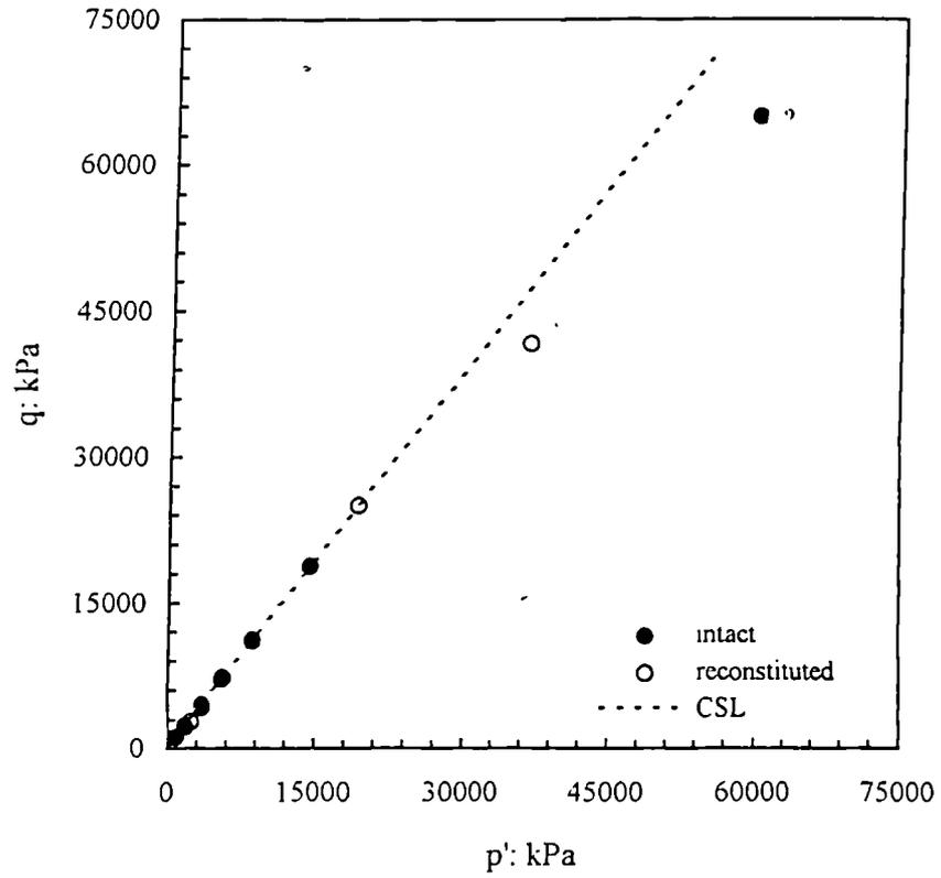
Figure 6.10 Ultimate states of intact and reconstituted samples of silica sandstone.
