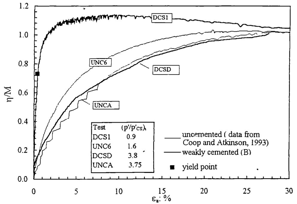
Figure 4.11 Shear behaviour of the weakly cemented samples (type B) and uncemented samples tested from similar initial values of  $p'/p'_{cs}$  at intermediate and high confining pressures.
