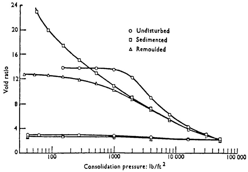
Figure 2.3 One-dimensional compression of Mexico City clay (after Mesri et al., 1975).
