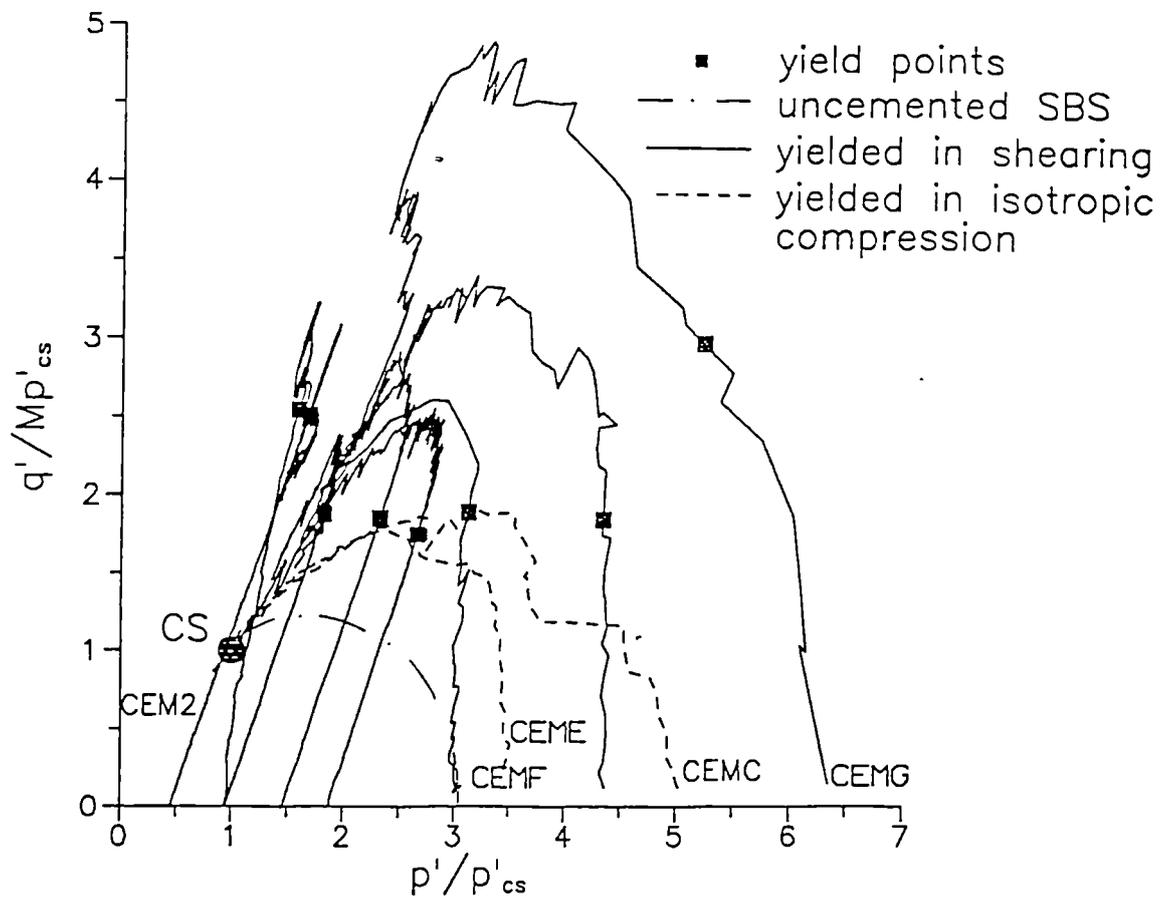
Figure 4.15 Normalized stress paths for the strongly cemented samples (after Coop and Atkinson, 1993).
