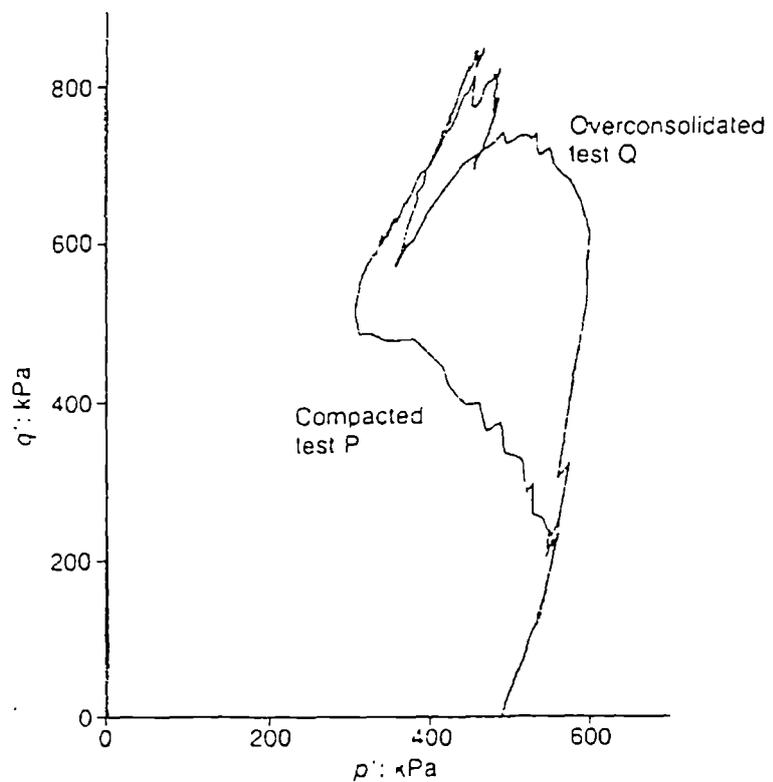
Figure 2.17 Stress paths for compacted and overconsolidated samples of a carbonate sand in undrained triaxial tests (after Coop and Lee, 1993).
