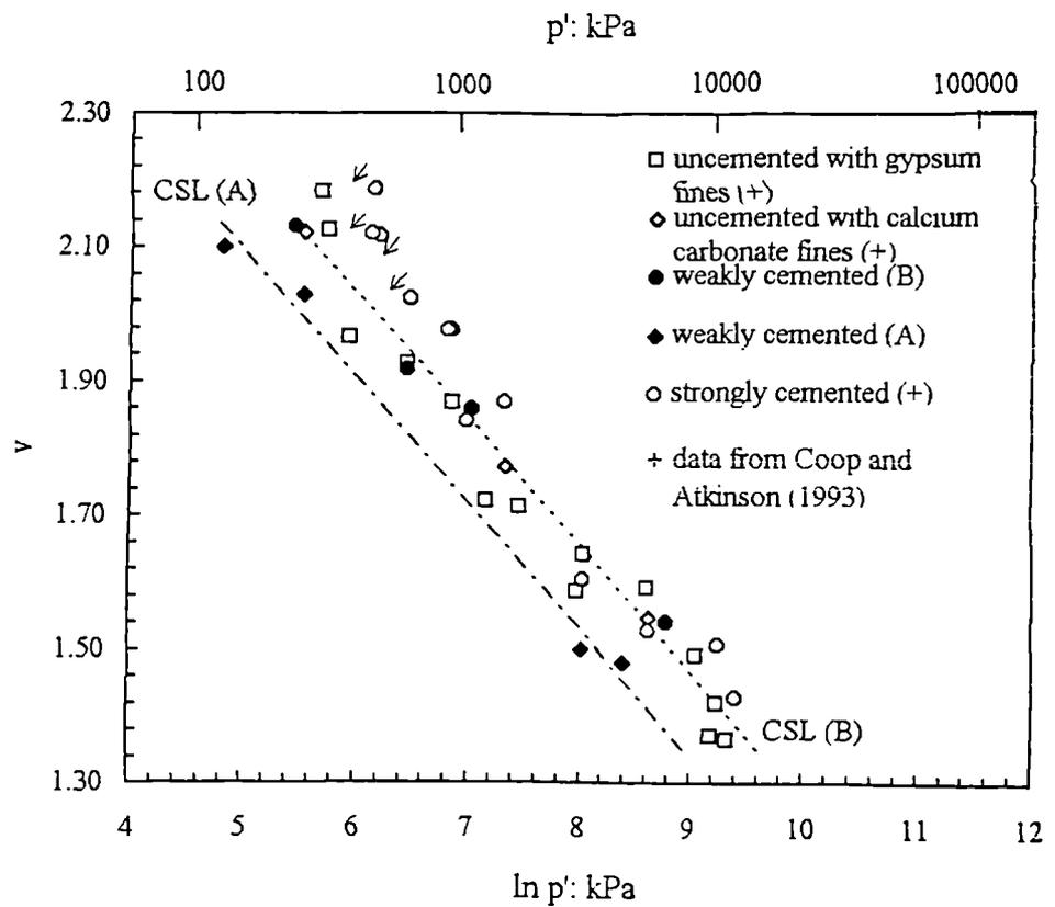
Figure 4.10 States at the end of shearing for uncemented, weakly and strongly cemented samples.
