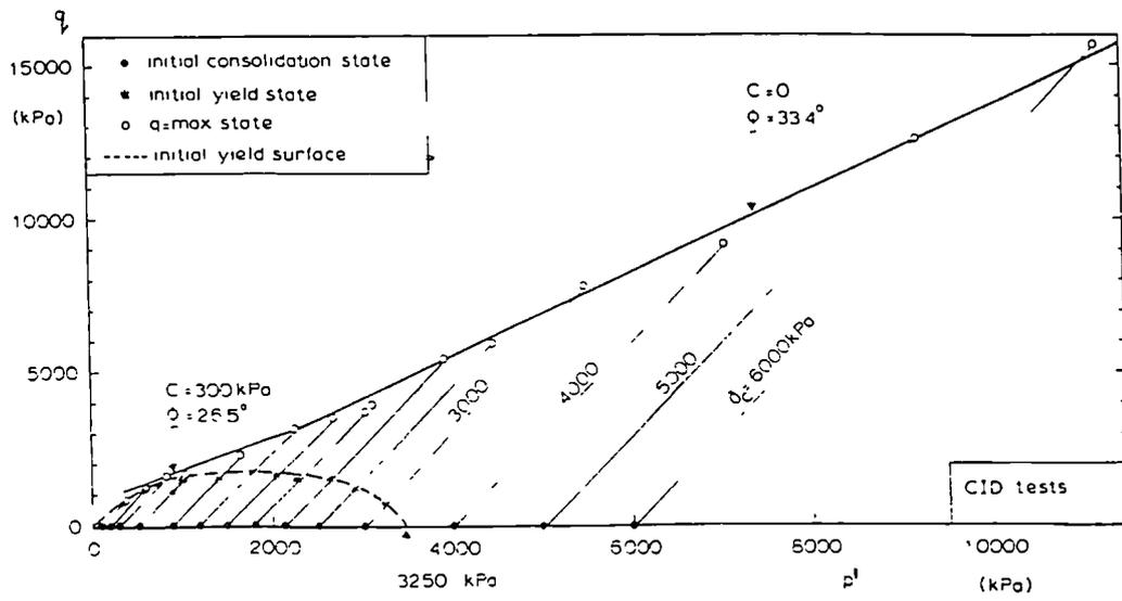
Figure 2.30 Stress paths for drained triaxial tests on a marl from the Corinth Canal (Anagnostopoulos et al., 1991).
