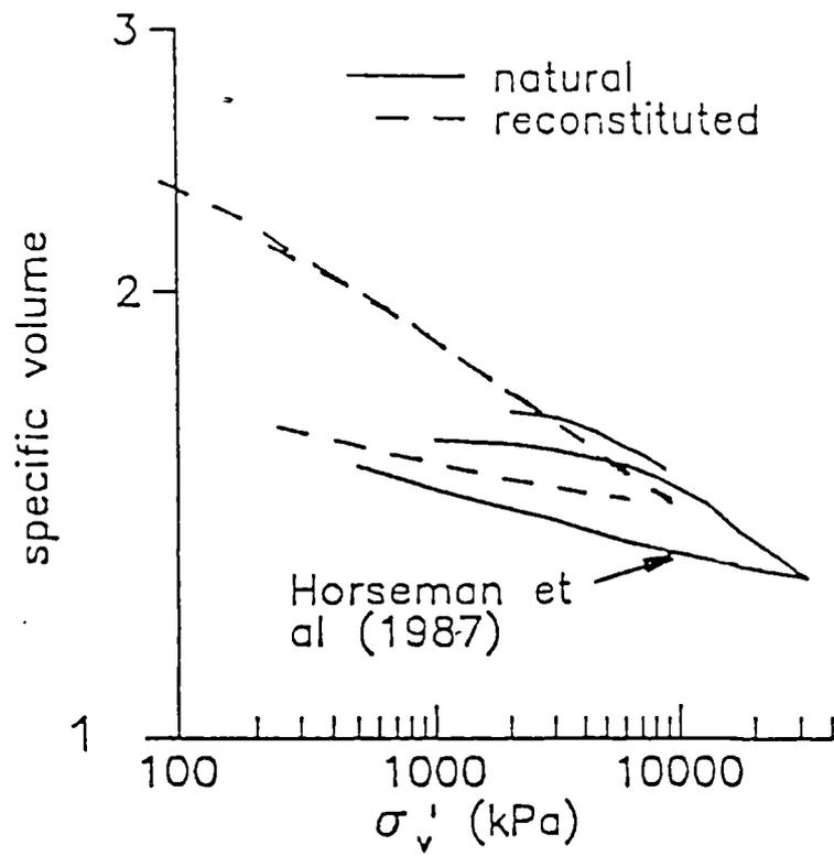
Figure 2.6 One-dimensional compression of Boom clay (after Coop et al., 1995).
