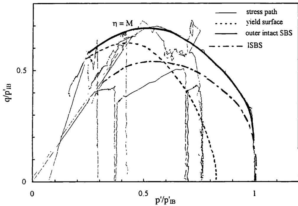
Figure 7.9 Shear behaviour of the calcarenite with identification of the yield surface, outer intact state boundary surface and intrinsic state boundary surface.
