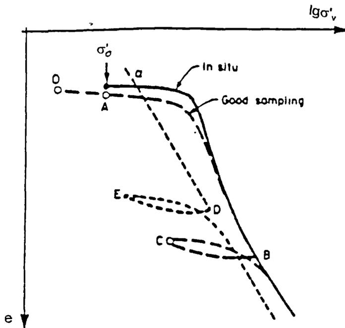
Figure 2.1 One-dimensional compression for a reconstituted sample, a good quality undisturbed sample and a natural clay in situ. (after Tavenas and Leroueil, 1987).
