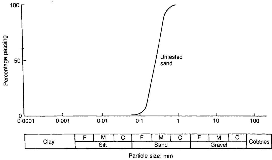
Figure 4.1a Grading curve of Dog's Bay sand (after Coop, 1990).
