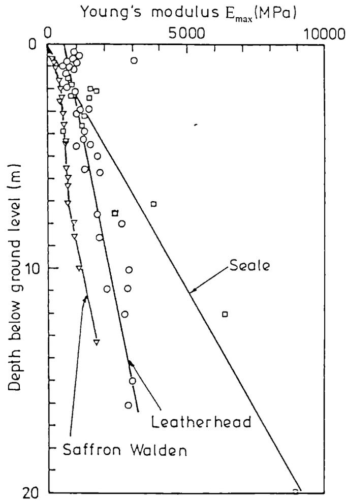
Figure 2.35 Variation of initial Young's modulus with depth for chalk at three different sites obtained from surface wave geophysics (Clayton, 1989).
