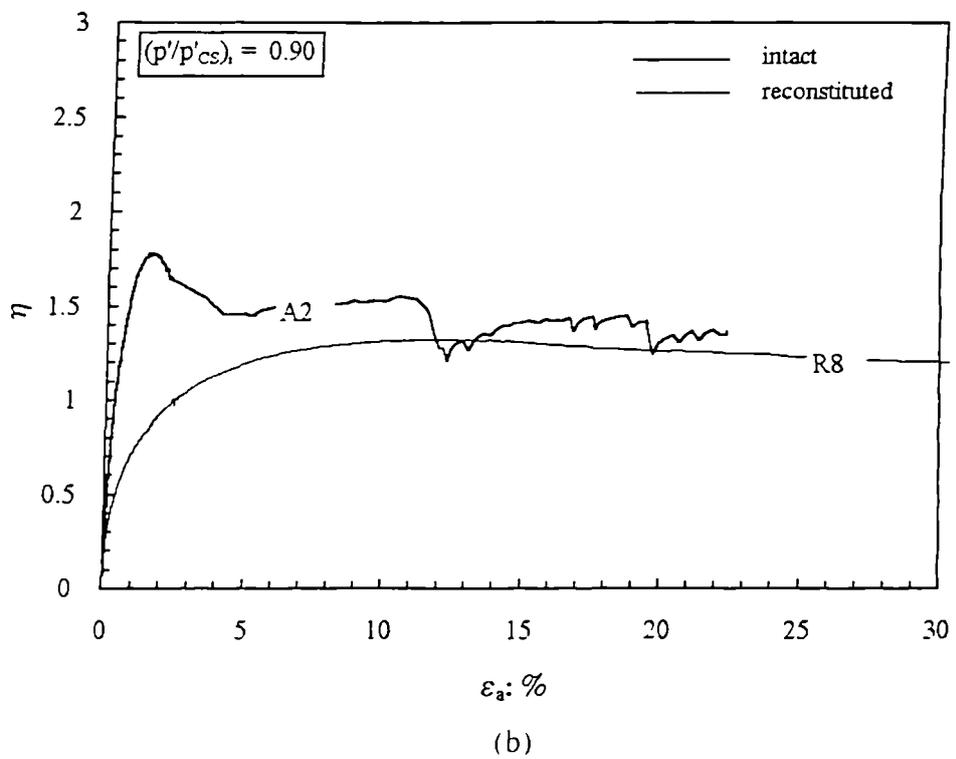
Figure 6.13 Shear behaviour of intact and reconstituted samples of silica sandstone tested from similar initial values of  $p'/p'_{cs}$  at (a) relatively low and (b) high confining pressures (constant  $p'$  tests).
