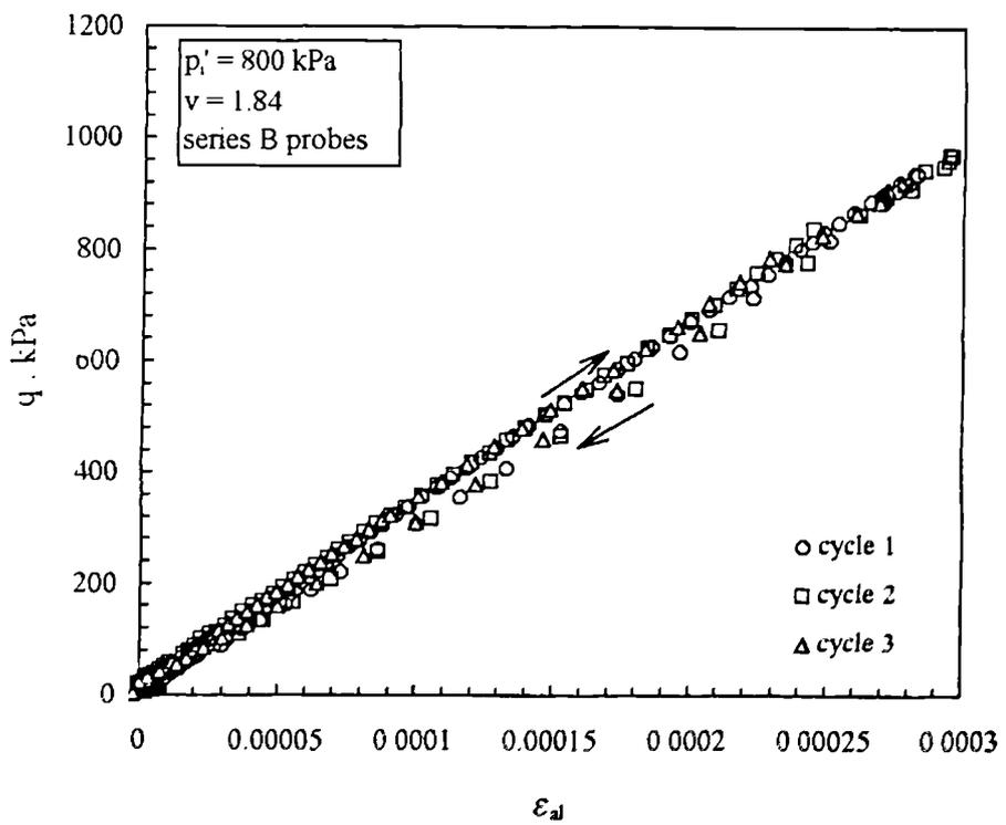
Figure 5.17 Pre-yield stress-strain relationships for undrained cycles performed on the calcarenite.
