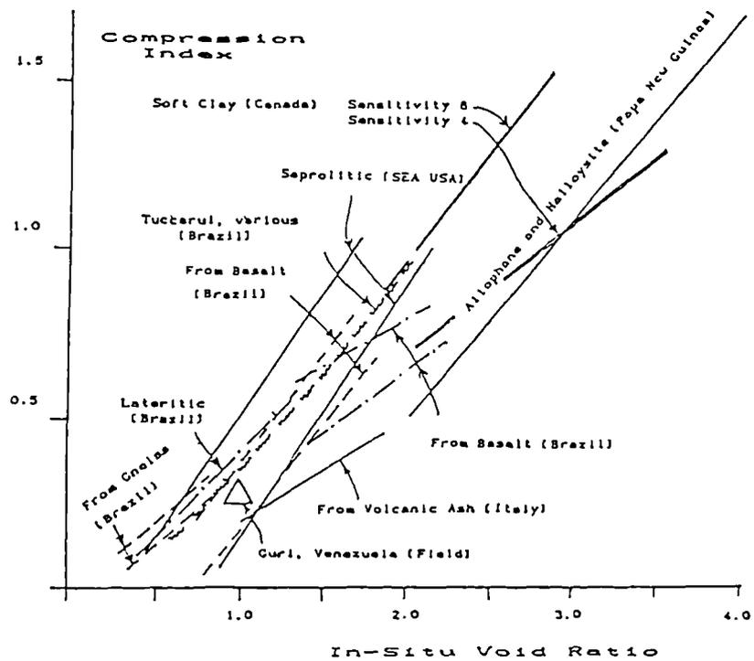
Figure 2.25 Relationship between compression index and initial void ratio in one-dimensional compression (after Vaughan, 1988).
