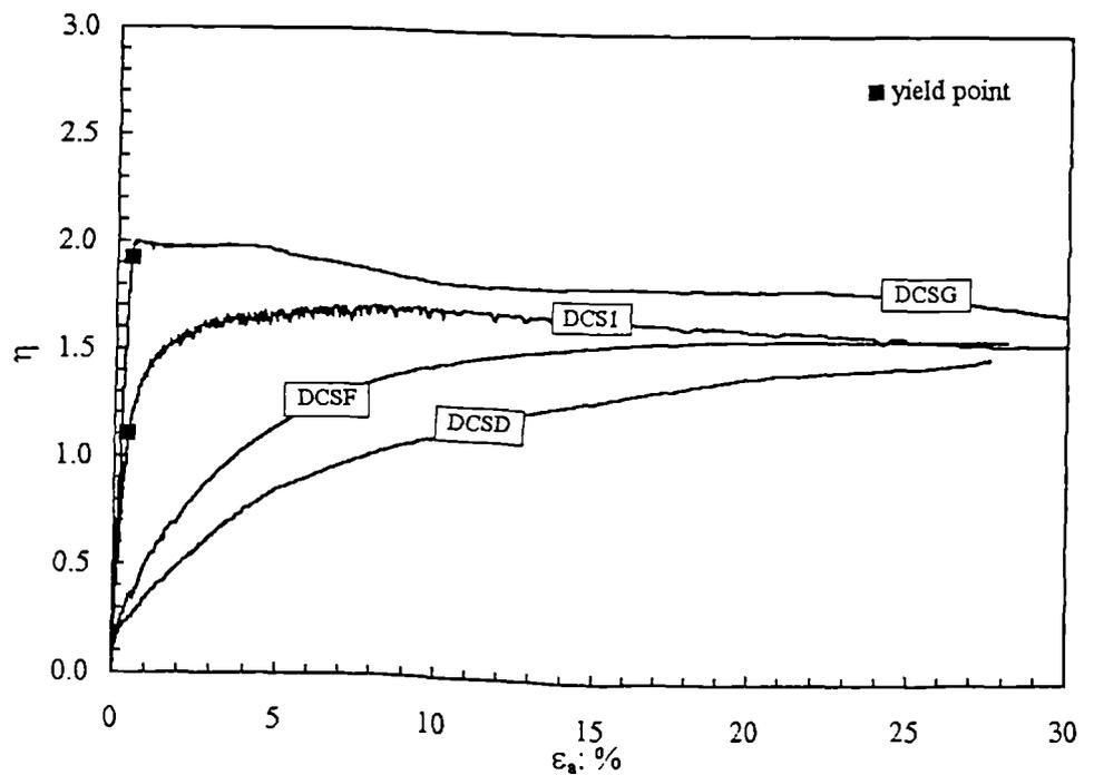
Figure 4.8 Stress ratios during shearing for all the weakly cemented samples prepared using method B.
