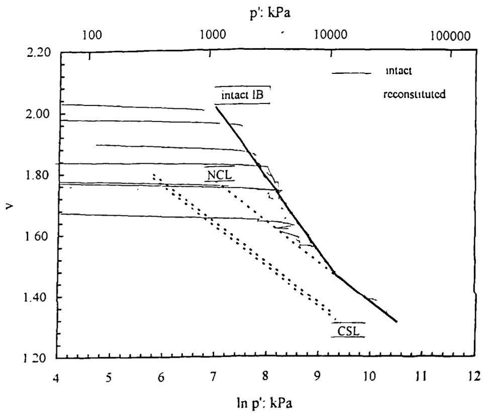
Figure 7.1 Isotropic boundary for the intact samples of calcarenite.
