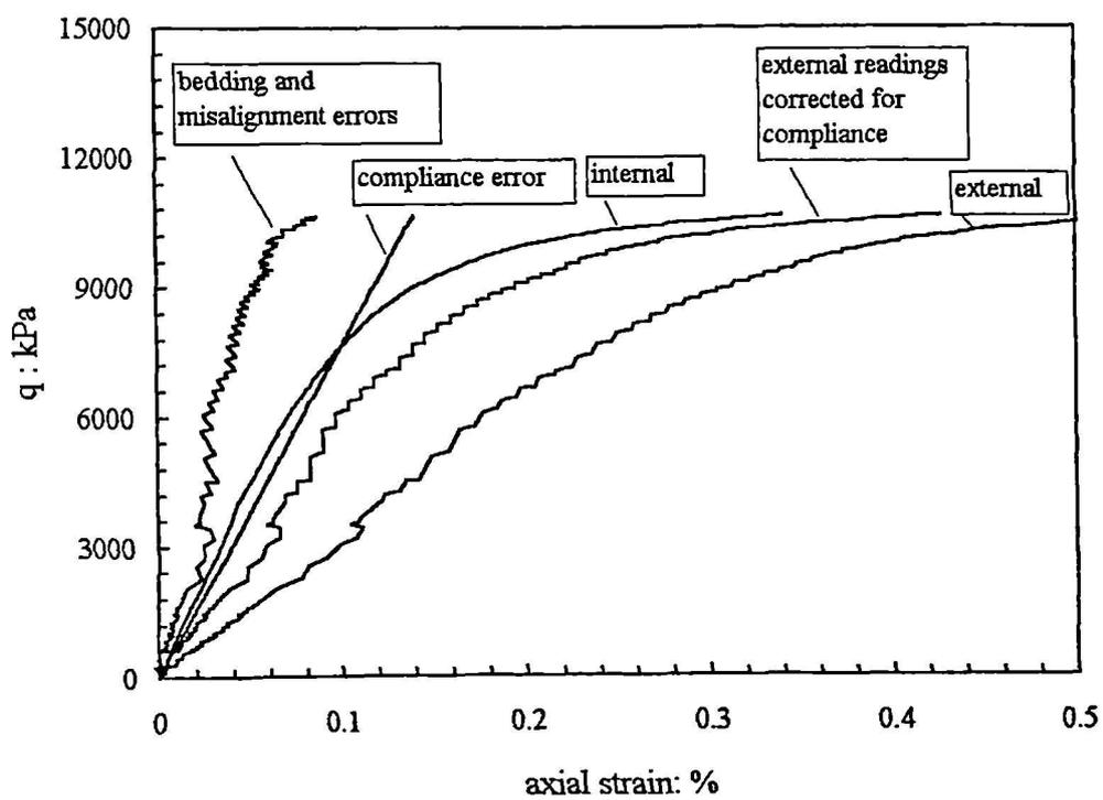
Figure 3.5 Errors affecting external axial strain measurements.
