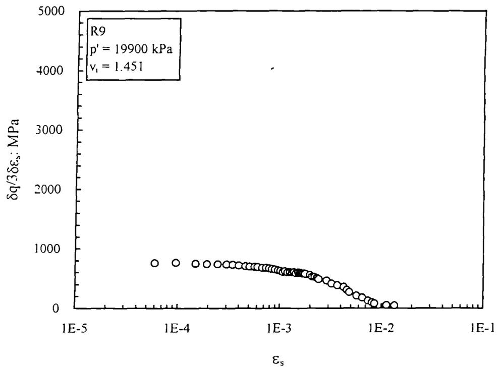
Figure 6.27 Tangent shear modulus as a function of shear strain for an overconsolidated reconstituted sample of the silica sandstone sheared at a constant value of  $p'$ .
