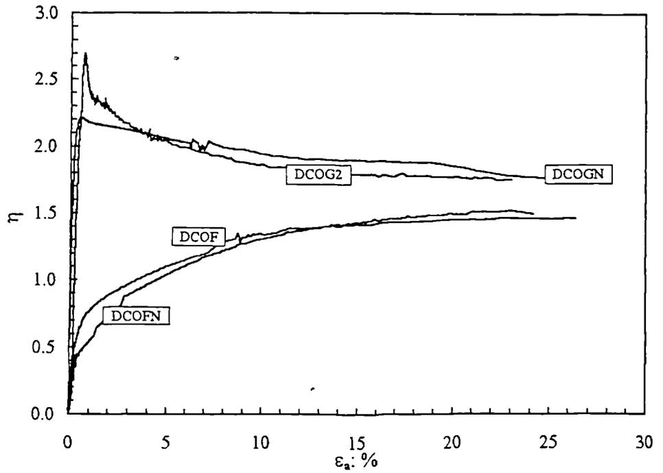
Figure 4.9 Stress ratios during shearing for all the weakly cemented samples prepared using method A.
