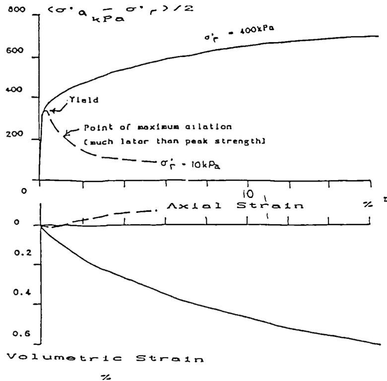
Figure 2.33 Drained triaxial tests on a residual soil from basalt (after Maccarini, 1987).
