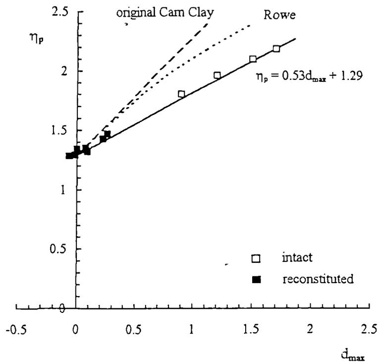
Figure 7.15 Peak stress ratio as function of maximum rate of dilation for intact and reconstituted silica sandstone.
