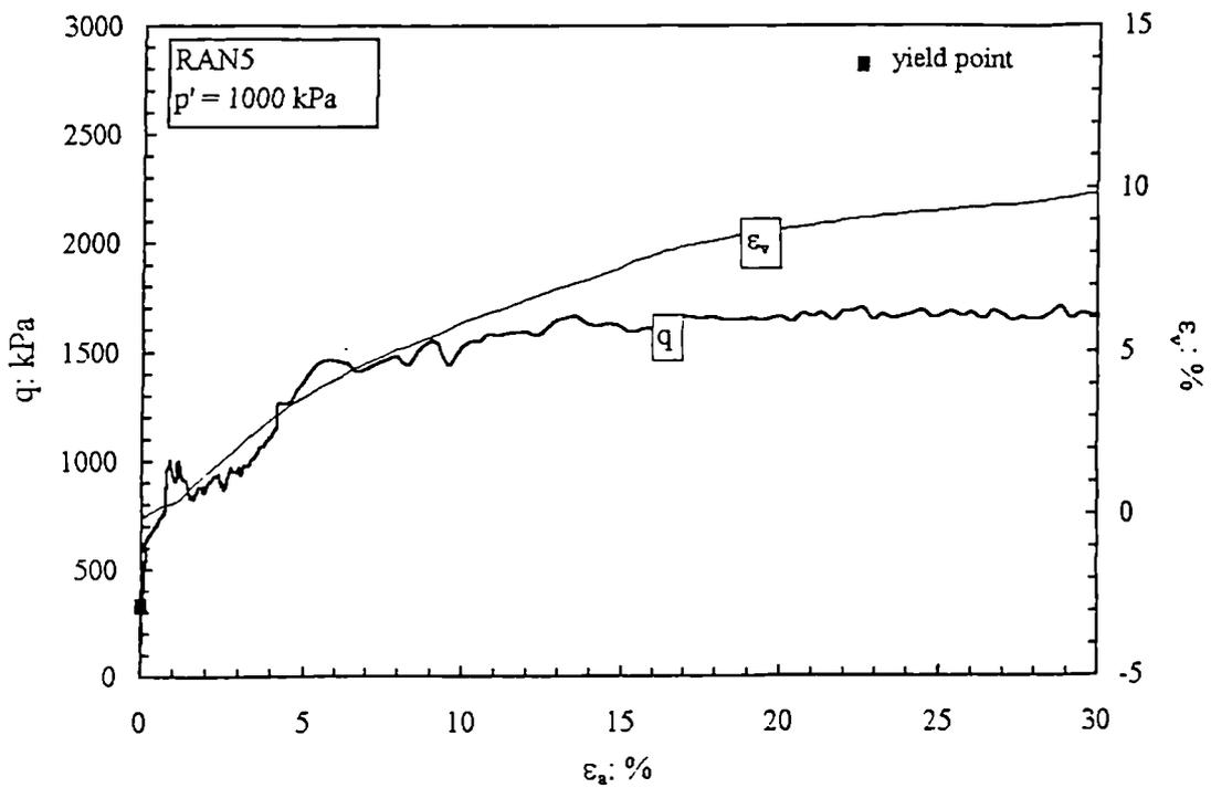
Figure 5.6 Stress-strain curve from a drained constant  $p'$  test performed on the calcarenite at intermediate confining pressures (after Coop and Atkinson, 1993).
