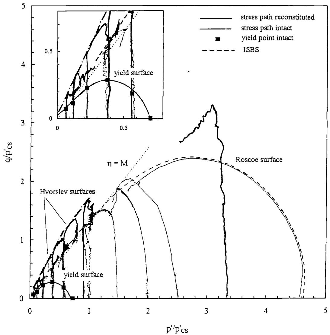
Figure 7.19 Shear behaviour of the reconstituted and intact silica sandstone referring the normalization of the intact soil to the CSL of the reconstituted soil.
