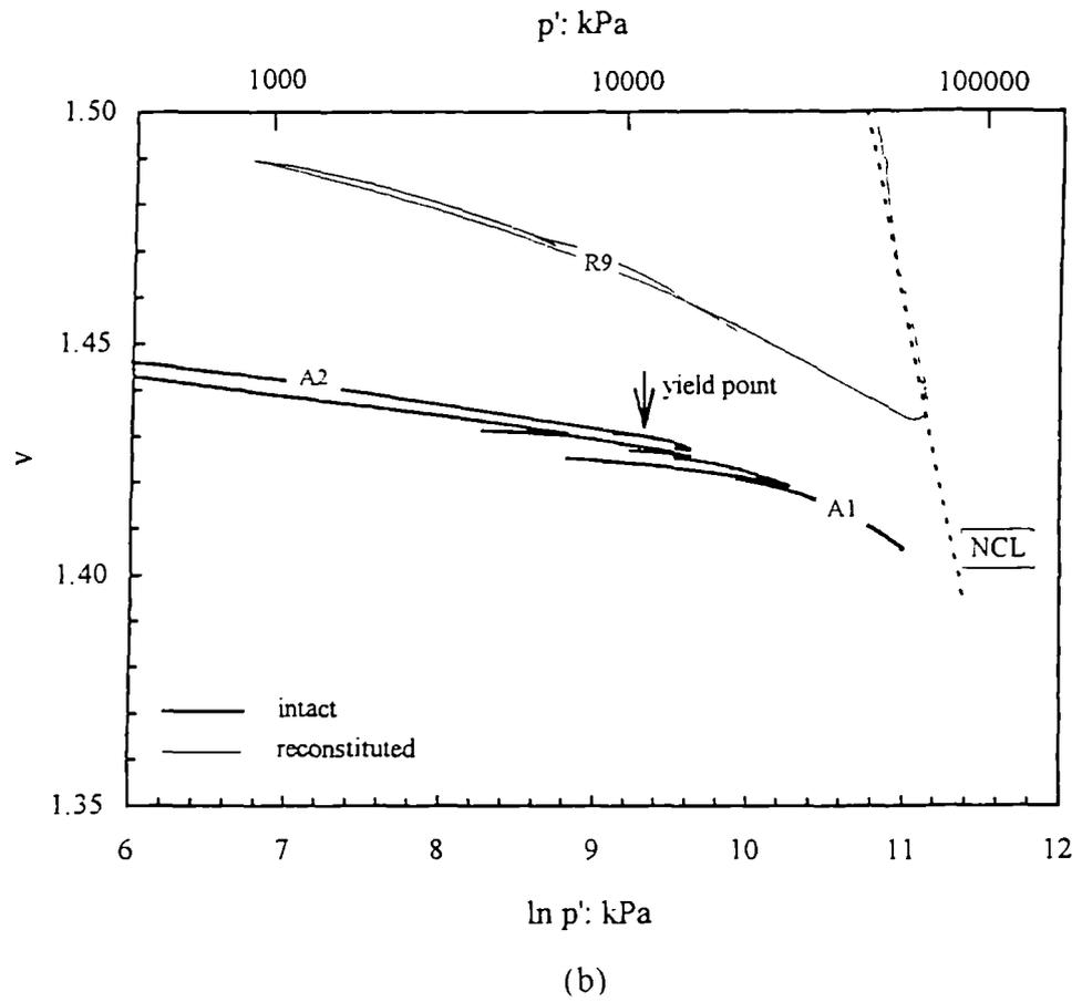
Figure 6.6 Isotropic compression of intact and reconstituted samples of silica sandstone.
