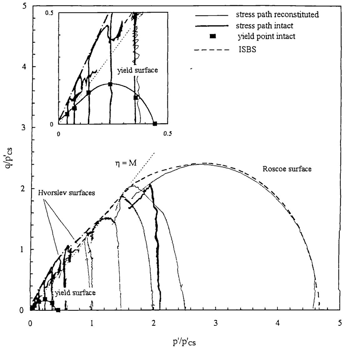
Figure 7.20 Shear behaviour of the reconstituted and intact silica sandstone referring the normalization of the intact soil to a CSL as indicated by Figure 7.16.
