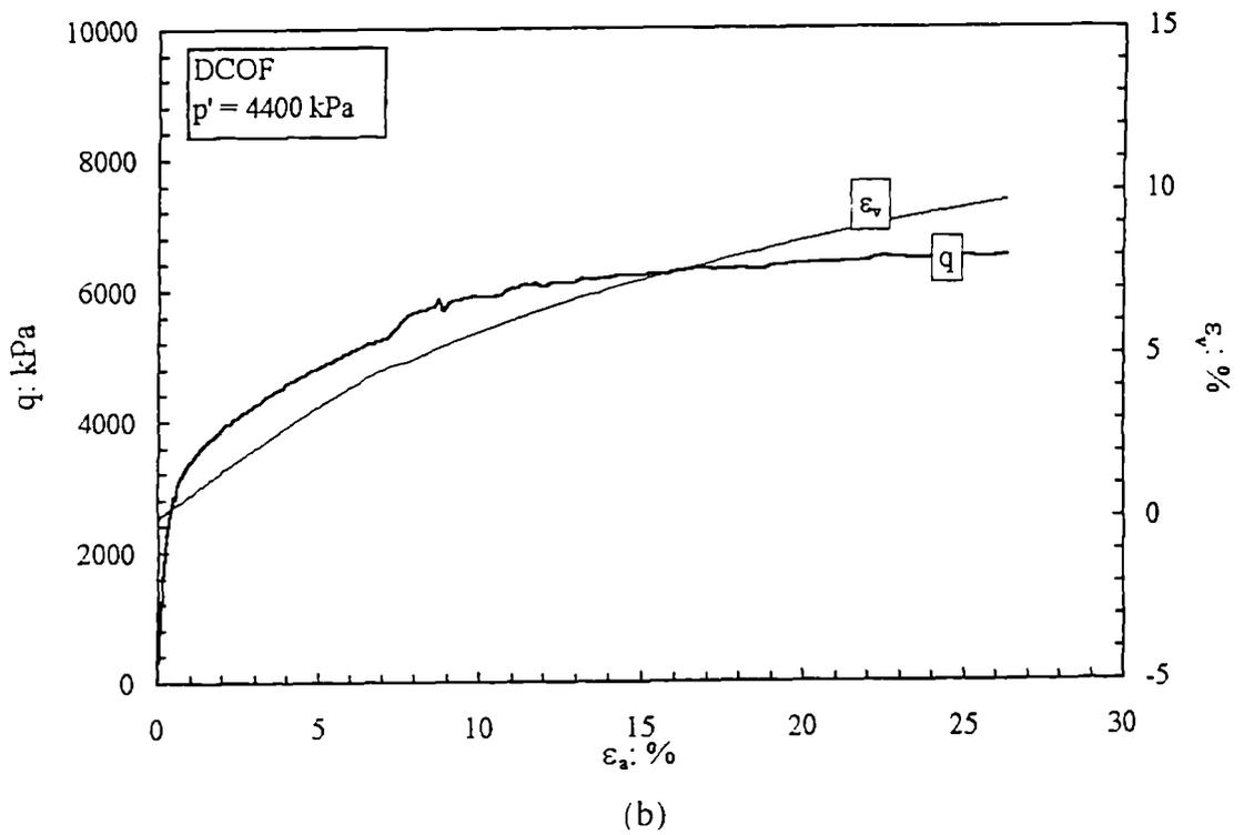
Figure 4.6 Stress-strain curves of the weakly cemented sand prepared by method A: (a) at low confining pressures; (b) at high confining pressures.
