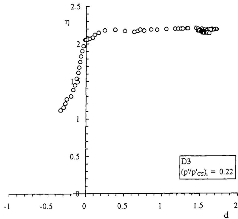
Figure 7.14 Stress-dilatancy relationship for an intact sample of silica sandstone sheared at a constant  $p'$  from a low value of  $p'/p'_{cs}$ .
