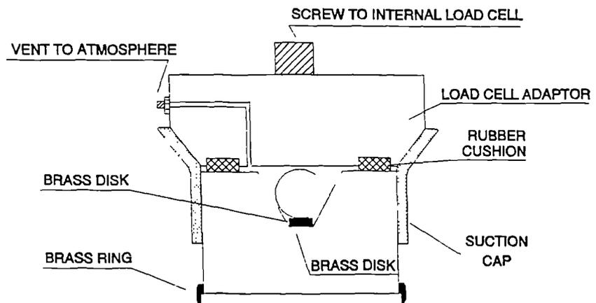
Figure 3.11 Redesigned connection between the sample and the internal load cell.
