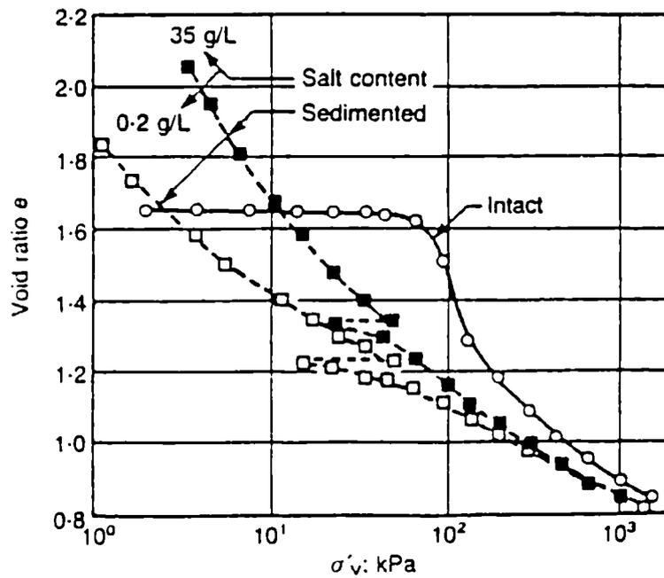
Figure 2.4 One-dimensional compression of the Grande Baleine clay (after Locat and Lefebvre, 1985).
