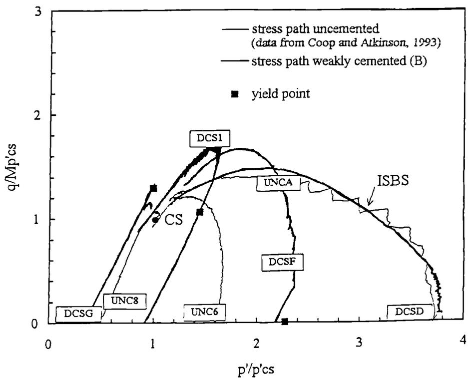
Figure 4.14 Normalized stress paths for the weakly cemented samples prepared using method B compared with those for the uncemented samples.
