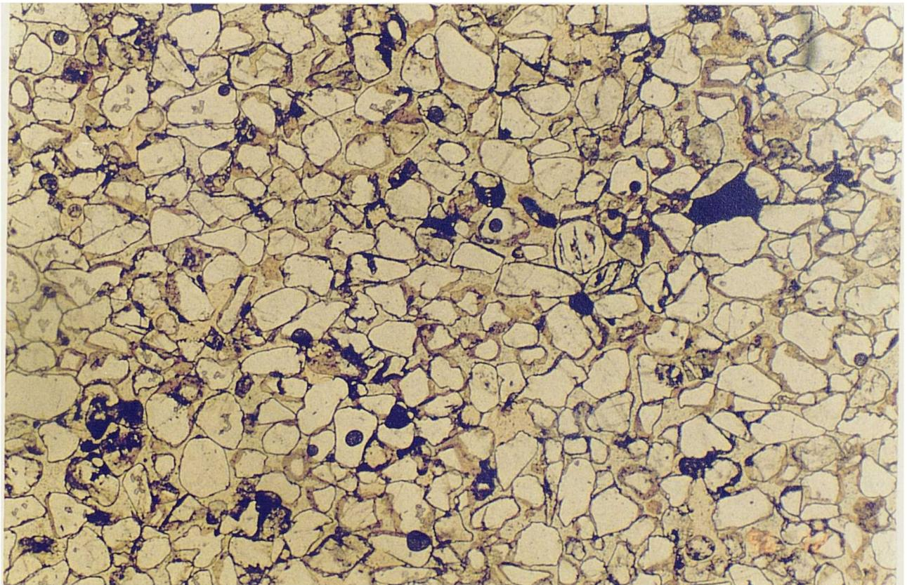
Figure 6.3 Thin section of the silica sandstone under plain white light.
