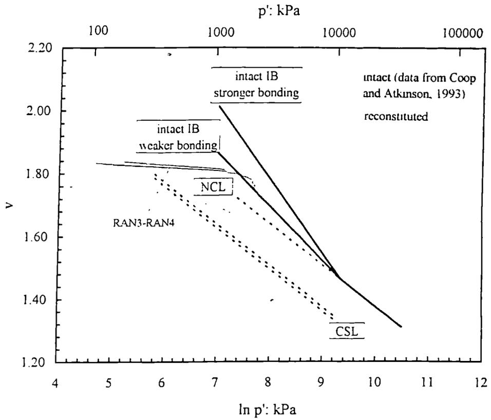
Figure 7.6 Isotropic boundary for the intact samples of calcarenite with weaker bonding.
