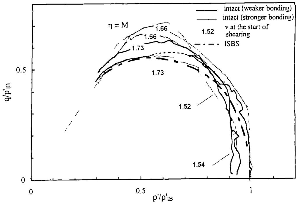
Figure 7.8b Normalized stress paths for intact samples of calcarenite with weaker and stronger bonding sheared after isotropic yielding.
