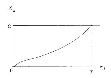
Figure 1.2 – Example of Threshold Failure Model
