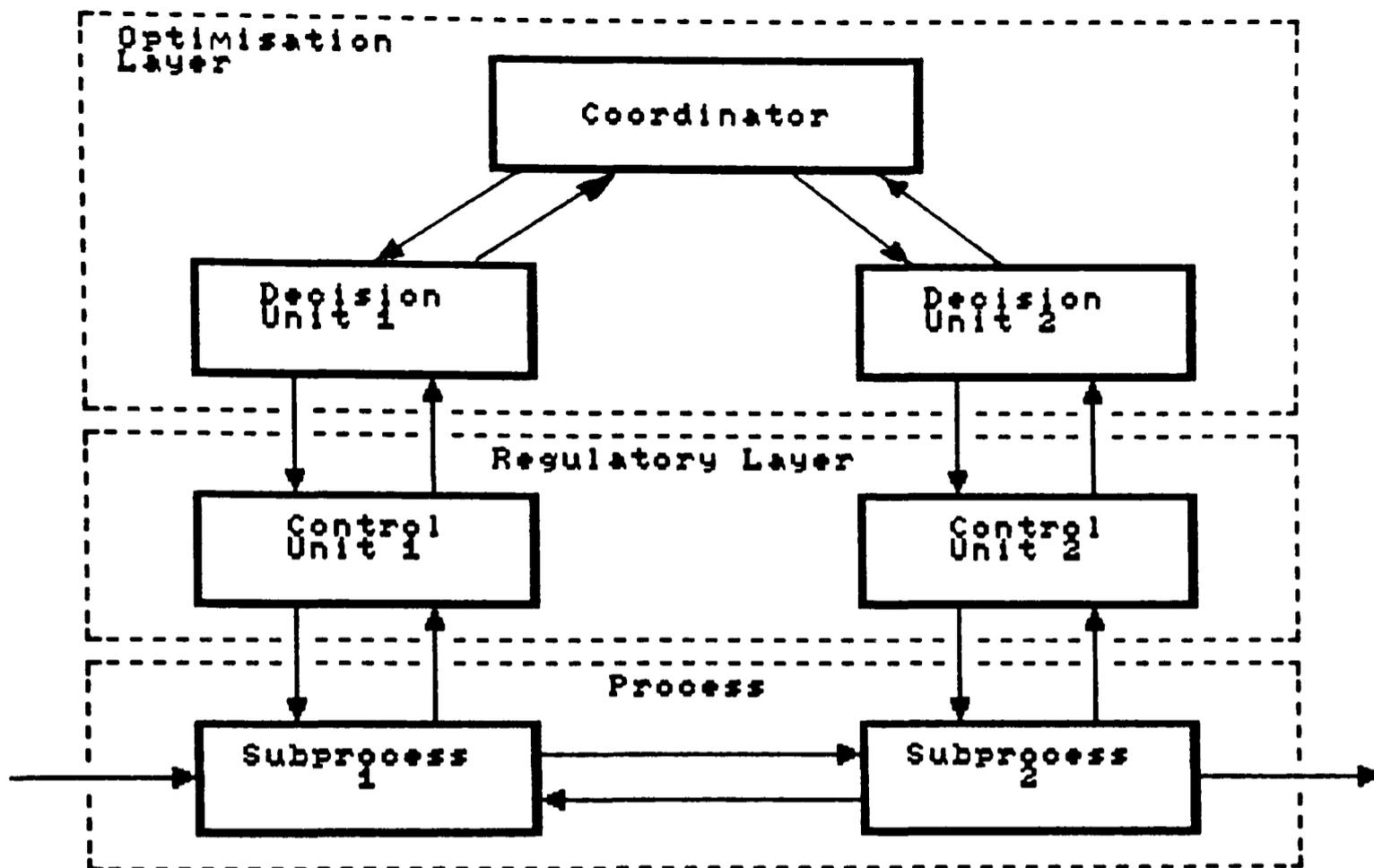
Figure (2.9) Two layer Hierarchical structure.
