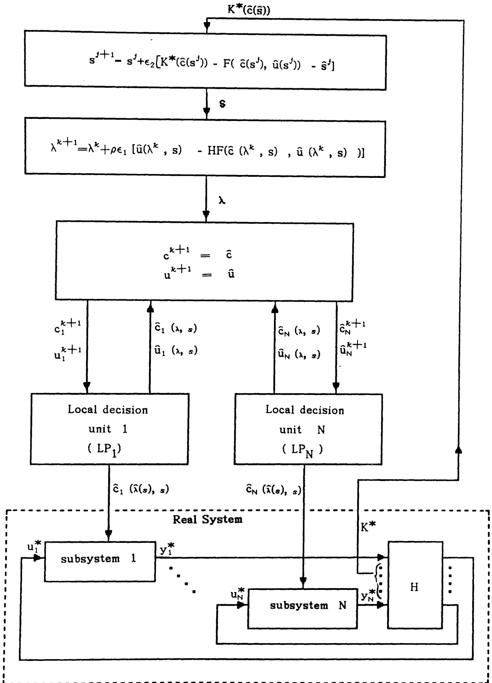
Figure ( 5. 2) Structure of Algorithm.
