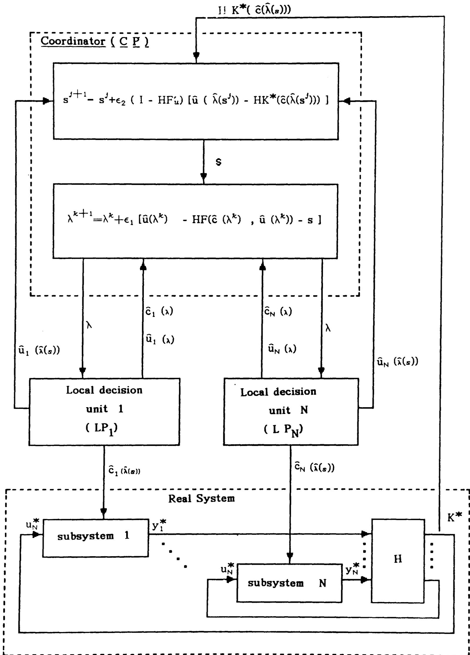
Figure ( 4. 2) Information Structure of Version 1 Algorithm.
