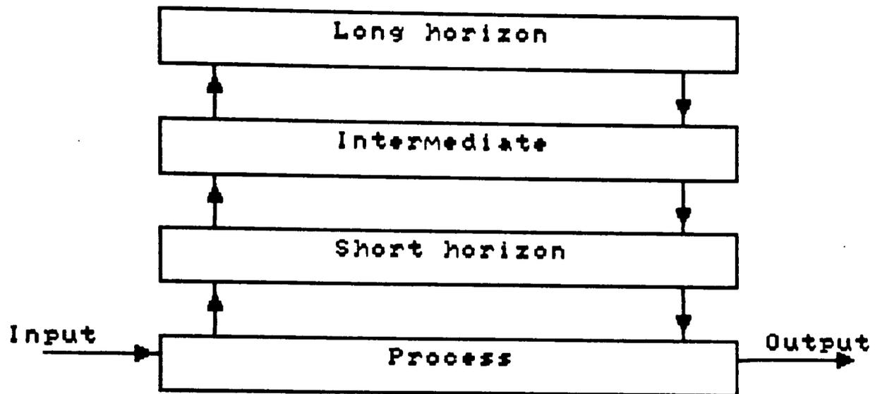
Figure (2.7) The stratified decomposition of control system.
