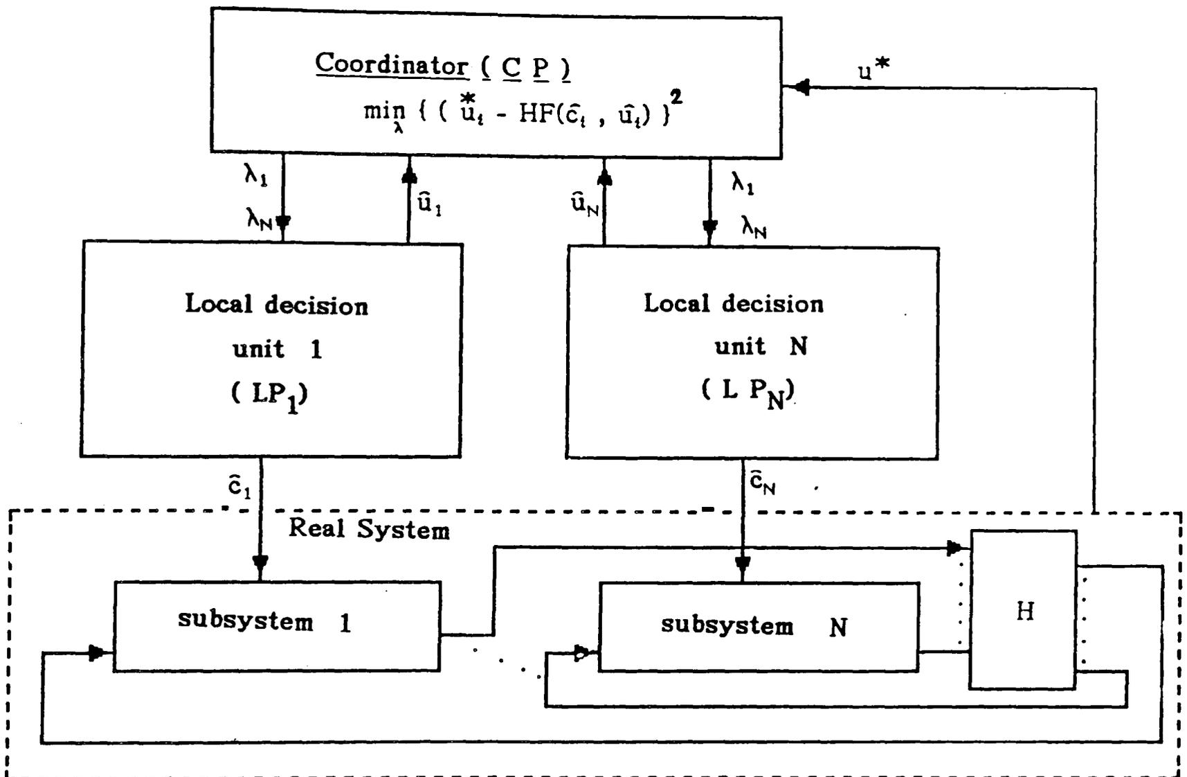
Figure ( 4. 1 ) Closed loop Price method with global feedback.
