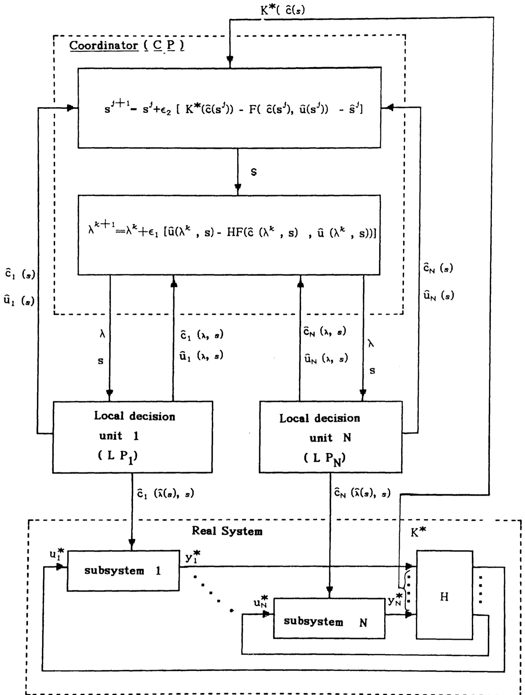
Figure ( 4. 3) Information Structure of Version 2 Algorithm.
