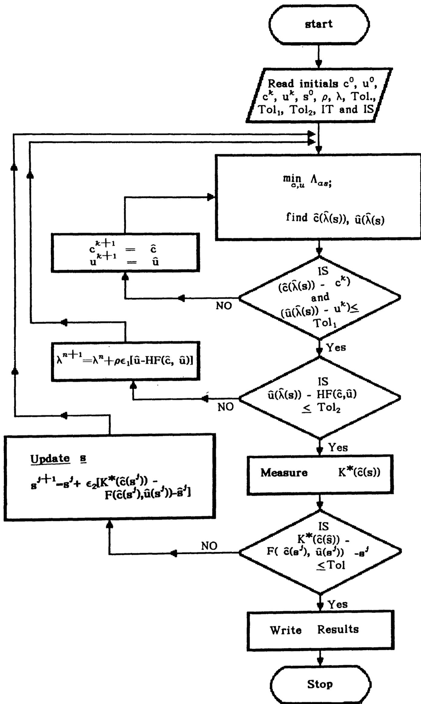
Figure (5.1) Flow chart of the Augmented Price Correction Algorithm.
